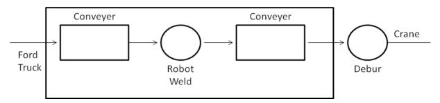
Figure 3.3 Automated Welding System Detailed Area for Simulation
