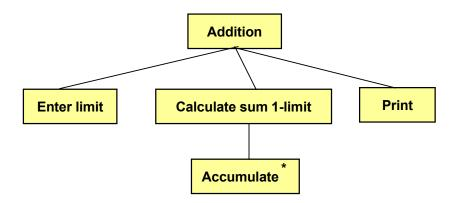
First the user is prompted for a limit. The following loop goes from 1 to limit with the loop variable i. For each turn of the loop we add the value of i to the sum, i.e. we accumulate the numbers. Finally we print the accumulated sum. Note that the operation to be repeated (Accumulate) in the loop is indicated by an asterix in the JSP graph.
