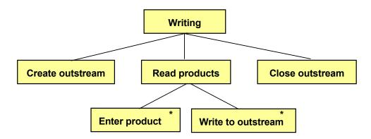
First we declare an outstream and attach it the file prodfile.txt. Entry of product names from the keyboard is made in a loop. As soon as a product name has been entered by the user, it is written to the outstream. At entry completion, we close the outstream.
