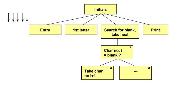
Searching for the blank is made in a loop. For each turn of the loop we check if character no. i is blank. If so, we take character no. i+1 as the second initial. Here is the code:
