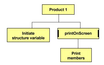
We initiate a structure variable, which is sent to the function, where the members are printed.
