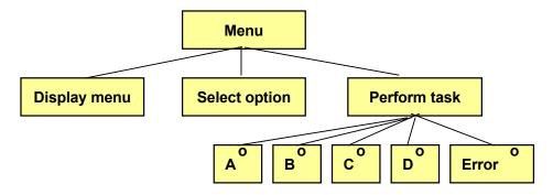
The first action is that the menu is displayed. Then the user is prompted for a choice by means of the letters A-D. Finally the requested option is executed, i.e. a simple text message will be printed. If the user enters another character than A-D, an error message is printed. Here is the code:
