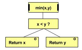
As shown by the JSP the function takes two parameters, x and y, and checks whether x is less than y. If so, x is returned, otherwise y.
