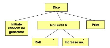
We begin with initiating the random number generator to a randomly selected start position. Then the loop is repeated until we get 6. For each turn of the loop we roll the dice once more and increase the number of rolls by 1. When 6 has been achieved, the loop is terminated and the number of rolls is printed. Here's the code: Download free eBooks at bookboon.com
