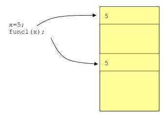
The variable x has the value 5 stored in a memory location. When func1() is called, that value is copied to another memory location used by the function. If a statement in the function would change the value to 6, the memory location of the function is affected, but not the original value of x:
