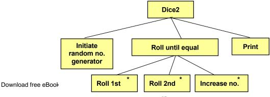
When having initiated the random number generator to a random start position, the loop begins. For each turn, we roll the 1<sup>st</sup> and then the 2<sup>nd</sup> dice, and then increase the counter by 1. When the two rolls are equal the loop is terminated and the number of "double" rolls is printed. Here is the code:
