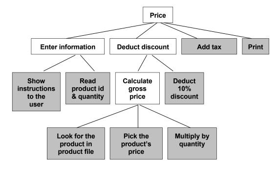
We could refine the algorithm further, but let us say that we are satisfied with the detail level. The shadowed boxes in the graph are the end points at the lowest level, the "leaves of the tree". These are the boxes to be used for coding, from left to right.
