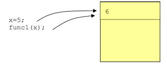
Defining a function parameter as reference parameter is made by placing an & character after the data type:
