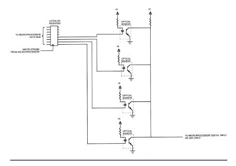
Figure 3.10 Multiple optical sensors with a single output.
