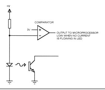
Figure 3.11 Detecting an open LED.
