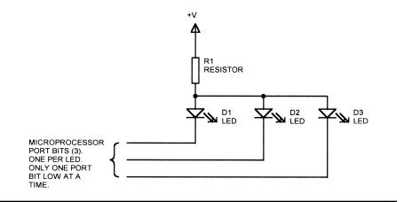
Figure 6.15 Multiple multiplexed LEDs.
