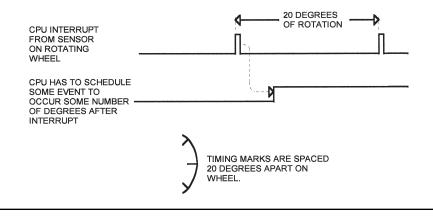
Figure 1.2 Rotating wheel timing.
