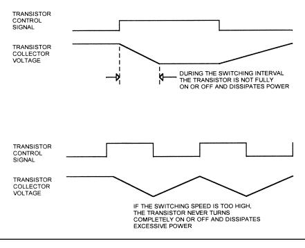
**Figure B.4** PWM switching dissipation.
