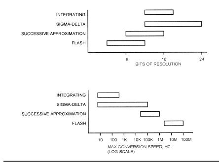
Figure 2.8 ADC comparison.
