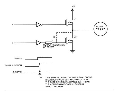
Figure 7.13 Shoot-through caused by MOSFET capacitance.
