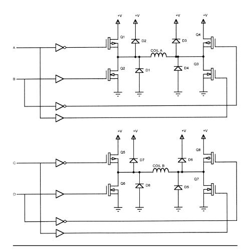
Figure 7.10 H-bridge circuit.
