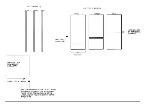
**Figure 3.21** Trilinear data alignment.
