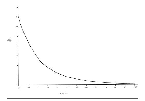
Figure 3.1 Thermistor resistance/temperature curve.
