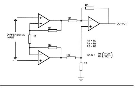
Figure A.6 Instrumentation amplifier.
