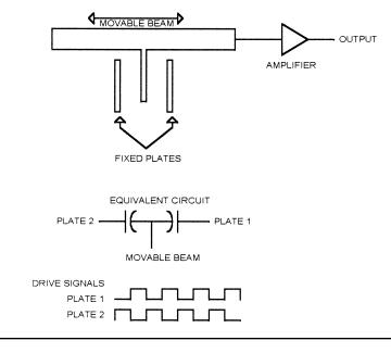
Figure 3.28 Solid-state acceleration sensor.
