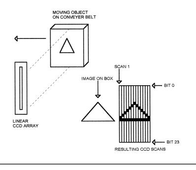
Figure 3.17 Linear CCD imaging.
