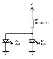
Figure 6.13 Multiple LEDs in parallel.
