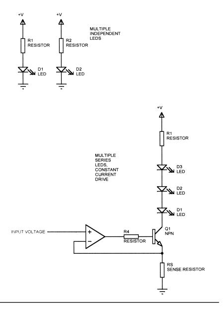
Figure 6.14 Multiple series LEDs.
