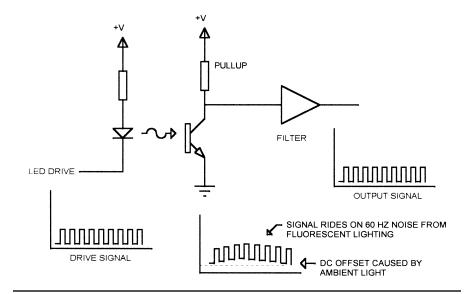
Figure 3.9 Optical sensor filtering.
