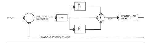
Figure 5.5 PID control system.
