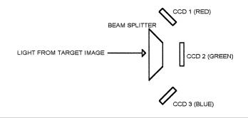
Figure 3.19 Color imaging with a beam-splitter.
