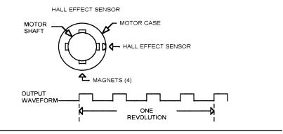
Figure 7.27 Hall effect motor shaft encoder.
