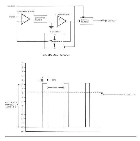
Figure 2.6 Sigma-delta ADC.
