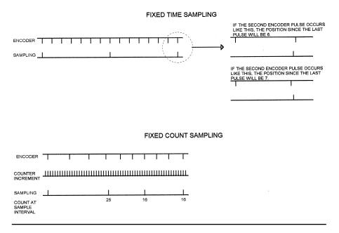
Figure 5.18 Motor sampling. If you use fixed-count sampling, you should include some kind of timeout to detect a stalled motor. If the motor stalls, no encoder counts will be generated and no sampling will occur.
