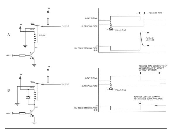
Figure 6.1 Relay control and clamping.
