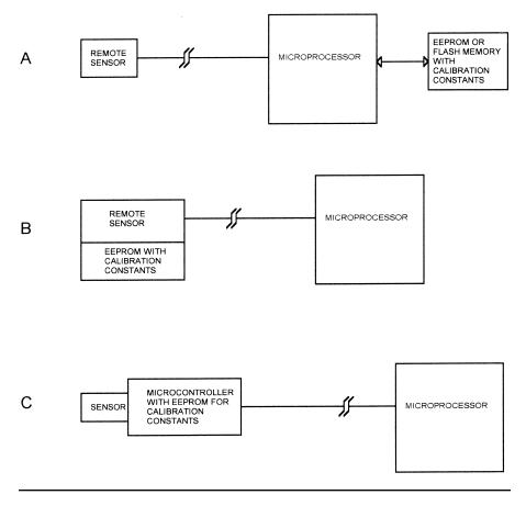
Figure 1.1 Sensor calibration methods.
