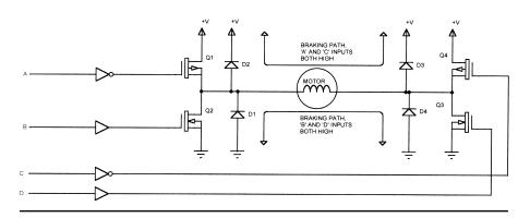
Figure 7.22 DC motor braking.
