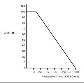
Figure 9.3 LM318 gain versus frequency.
