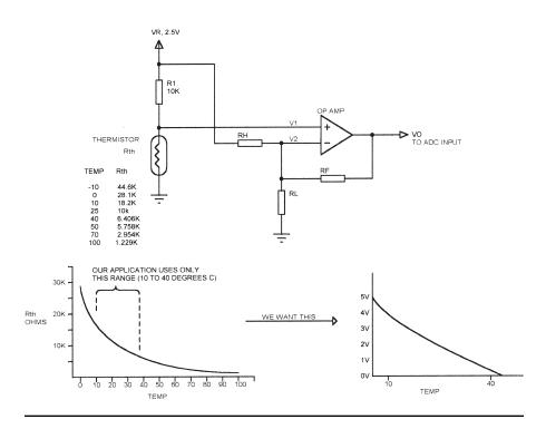
Figure 3.3 Thermistor scaling.
