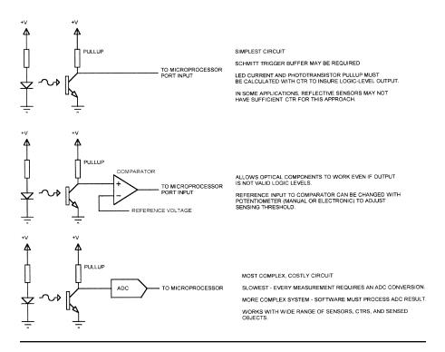
Figure 3.14 Interfacing optical sensors to a microprocessor.
