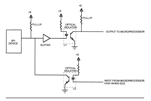
Figure 3.15 Bidirectional signal buffering with optoisolators.
