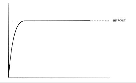
Figure 5.12 Critically damped system.
