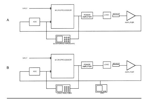
Figure 5.21 Monitoring a control system.
