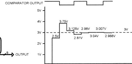
CONVERSION OF 3V INPUT USING 0-5V DAC. SAR SETS BIT 7, MAKING DAC OUTPUT 2.5V. COMPARATOR OUTPUT HIGH, SO INPUT > DAC. BIT 6 IS SET, MAKING DAC OUTPUT 3.75V. COMPARATOR OUTPUT LOW, SO BIT 6 IS RESET AND BIT 5 IS SET. PROCESS CONTINUES UNTIL ALL 8 BITS HAVE BEEN PROCESSED.
