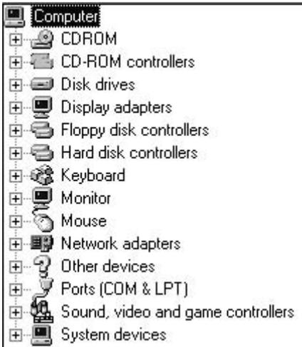
This list shows the range of input and output devices for a typical desktop microcomputer. These devices may often be memory-mapped and data is written from/to them via interface adaptors. Some ports are not memory mapped and a signal on the control bus identifies to the CPU that the address is that of a port and not a memory location.
