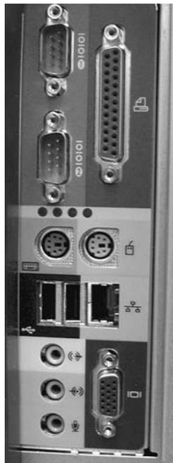
Typical I/O ports on a microcomputer
