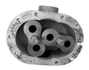
of liquid that is captured between the lobes of the impellers and the pulse count rate can thus be calibrated to provide flow rate in litres/minute. There should be enough back pressure on the outlet side of the flowmeter so that no gas pockets are formed during its operation. The positive displacement flowmeter is only suitable for liquid flow measurements.
