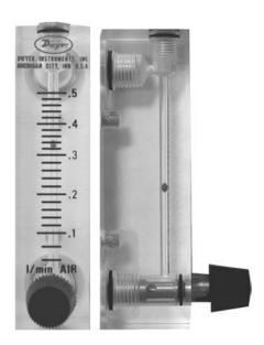
This type of flowmeter is very sensitive to the arrangement of inlet and discharge piping configurations. The inlet piping should be as large a diameter as the inlet to the meter and be as straight as possible – free from elbows, kinks and any other restrictions.
