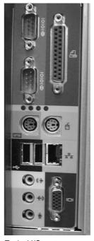
Typical I/O ports on a microcomputer
