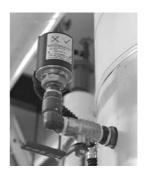
The diaphragms are typically made from stainless steel which allows them to be used with water and other corrosive fluids. In some applications, **silicon diaphragm** sensors are available that are useful for high frequency measurements. These devices have their strain gauges bonded to them by atomic diffusion during manufacture.
