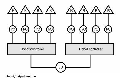
"I/O" are I/O modules. There are two separate robotic systems in this example, and their controllers are connected by an I/O module, allowing communication between the systems.
