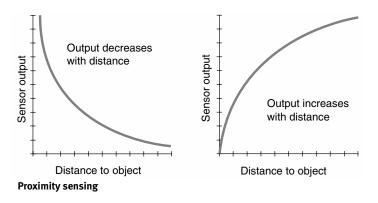
In theory, either type of displacement transducer can function in any application, but one type is usually easier to work with, in a given situation, than the other.
