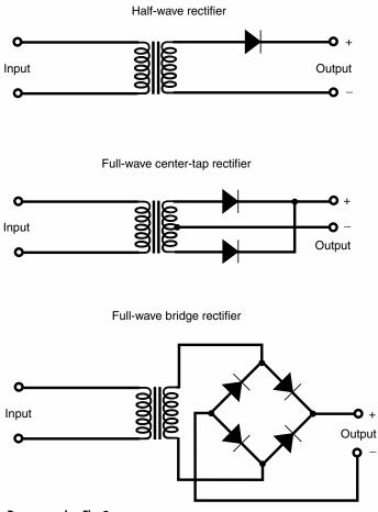
For high-current equipment, a *full-wave rectifier* is preferred. The full-wave scheme is also better when good voltage regulation is needed. This circuit makes use of both halves of the AC cycle to derive its DC output. There are two basic circuits for the full-wave supply. One version uses a center tap in the transformer, and needs two diodes. The other circuit uses four diodes and does not require a center-tapped transformer.
