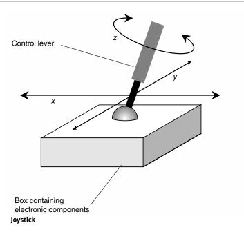
Joysticks are used in computer games, for entering coordinates into a computer, and for the remote control of robots. Many of these are more sophisticated than the basic device shown here; some require gripping with one or both hands.
