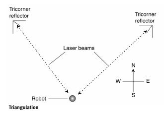
Triangulation need not use laser beams. Instead of the reflecting targets, beacons can be used. Instead of visible light, radio waves or sound waves can be used. Beacons eliminate the need for the 360° scanning transmitter in the robot.
