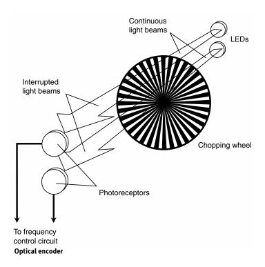
Optical encoders are used in various robotic applications. In particular, they are used in manipulators to measure the extent of joint rotation. See also ARTICULATED GEOMETRY and ROBOT ARM.
