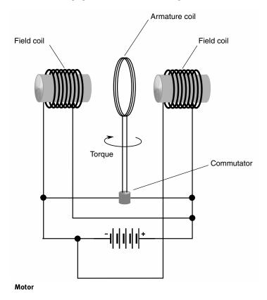
All motors operate by means of electromagnetic effects. Electric current flows through a set of coils, producing magnetic fields. The magnetic forces result in rotation. The greater the current in the coils, the greater is the rotating force. When the motor is connected to a load, the force needed to turn the shaft increases. The more the force, the greater the current flow, and the more power is drawn from the power source.
