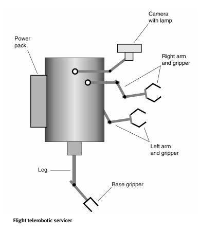
The FTS is a remote-controlled robot. The extent to which it is controlled depends on the design. The simplest FTS machines are programmable from the spacecraft's main computer. More complex FTS devices make use of *telepresence*.
