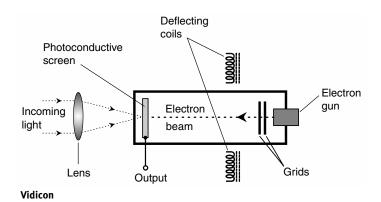
The camera in a common *videocassette recorder* (*VCR*) uses a vidicon. Closed-circuit television systems, such as those in stores and banks, also employ vidicons. The main advantage of the vidicon is its small physical bulk; it is easy to carry around. This makes it ideal for use in mobile robots.
