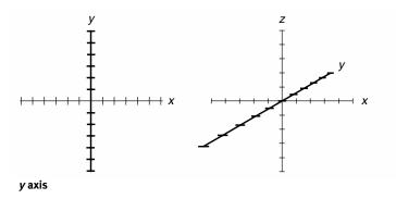
In *wrist-force sensing*, the *y* axis refers to inward/outward linear force vectors. Compare *x* axis and *z* axis.
