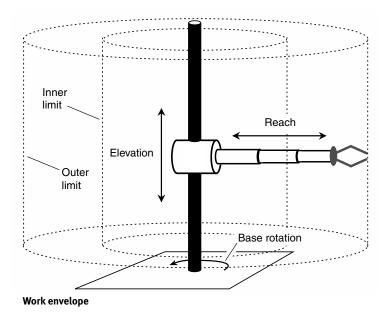
When choosing a robot arm for a certain industrial purpose, it is important that the work envelope be large enough to encompass all the points that the robot arm will be required to reach. But it is wasteful to use a robot arm with a work envelope much bigger than necessary. Compare **CONFIGURATION SPACE** and **WORK ENVIRONMENT.**
