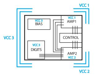
*Figure 7–11. Rearranged blocks now align with our premiere pin-out plan.*
