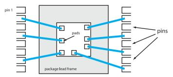
*Figure 9–3.* The circuit is connected to the bond pad that is connected to the wire that is connected to the package pin that is connected to the circuit board that Jack built.
