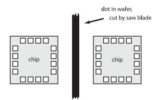
Figure 9–23. We must consider room for the saw blade.
