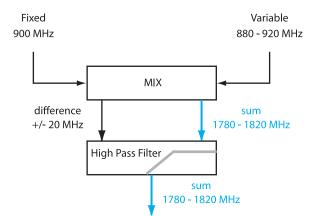
**Figure CS2–2.** High pass filter lets us listen to the sum of the two signals. Up-convert mixer can place information onto a carrier wave, useful for transmitters.
