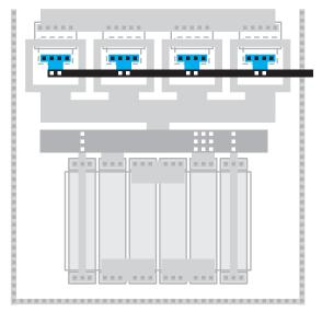
Figure CS2-31. Bases connected in Metal Two.
