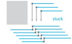
Figure 2–6. Metal Two is already used in this area.
