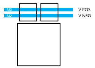
Figure CS1-67. ESD supply rails in Metal Two, built into the chip.
