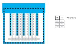
*Figure CS1–51. Positive power rail connected to device and N well contacts.*
