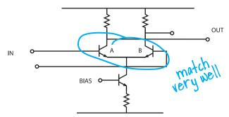
*Figure 5–14.* Two devices to be matched very well. This sounds like a job for cross-quading.
