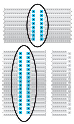
*Figure CS1–6.* Rotating devices. Gate connections are close to each other to improve matching.
