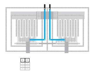
Figure CS1-56. Symmetrical output traces heading toward bond pads.
