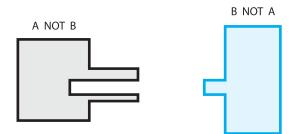
*Figure 10–10. The NOT function is order-sensitive. Notice the different results just by switching A and B in the order:*<sup>2</sup>
