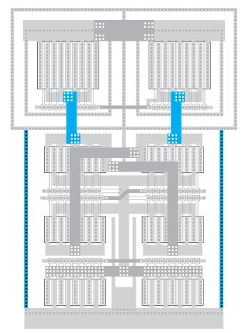
Figure CS1-55. Connecting PMOS to NMOS in Metal Two.
