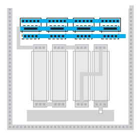
*Figure CS2–8.* Four devices in parallel make up the Current Source transistor.
