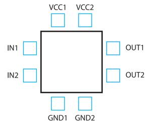
Figure 7-1. Like items set side by side. One possible pin-out.
