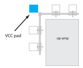
Figure CS1-80. Placement of VCC pad.
