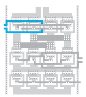
Figure CS2–50. Equal length inputs help matching.
