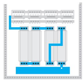
*Figure CS2–9.* Connecting the emitter to the resistor that leads to ground. Since we cannot stretch, we use four transistors in parallel, and we use four resistors in series. However, this is the same as one large transistor connecting to one large resistor.
