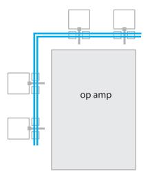
Figure CS1–77. ESD supplies wired to protection devices.
