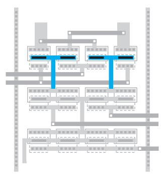
*Figure CS2–17. Emitters of each pair of devices in Upper Quad fed centrally.*
