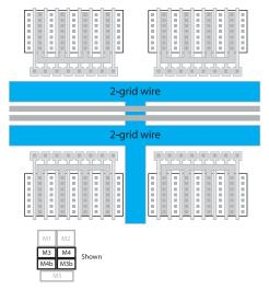
*Figure CS1–35. Moving the transistors back to allow room for the 2-grid wire.*
