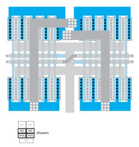
*Figure CS1–42.* Cross-quad area finished. Device outputs are connected in Metal Two with plenty of vias and wire width to allow good current flow.
