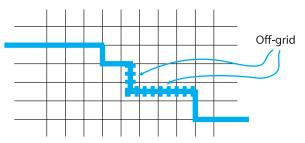
*Figure 11–1.* Two segments of the fine-grid trace are not placed on the coarser grid.
