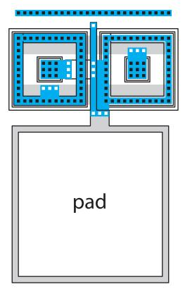
Figure CS1-75. Completed ESD protection cell.
