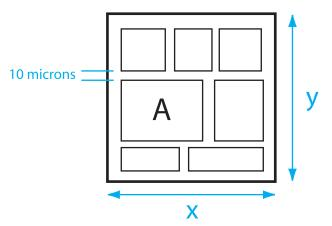
*Figure 7–15.* We are so proud of cramming in our blocks tightly. However, we only left 10 microns to run all our wires. This will lead people to believe you can produce a smaller chip than you really can. You tease, you.
