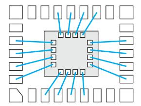
*Figure 9–11. Example of a good bond-out. It looks nice, so it will work well.*
