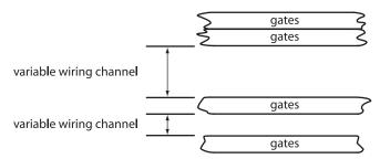
*Figure 2–26.* In variable-width channeling, our open spaces can be altered according to the needs predicted by the software.
