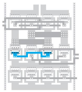
Figure CS2-40. Connecting bases of two device halves in Metal Two.
