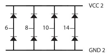
Figure 7-4. Pins 6, 8, 10, and 14 protected to VCC2 and GND2.
