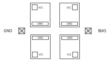
Figure CS1-86. Ground and bias pad placement.
