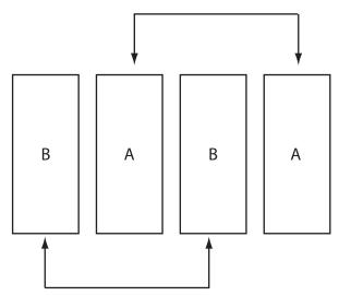
Figure CS2-53. Planning to interdigitate the resistor Loads.
