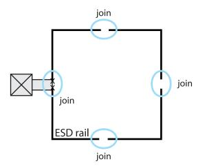
Figure CS1-87. ESD ground wiring connections.
