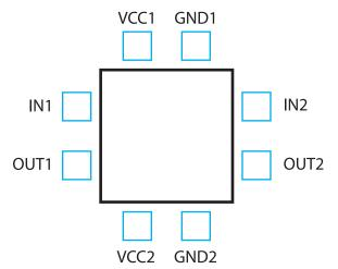
*Figure 7–2. Very different pin placement will produce a very different layout.*
