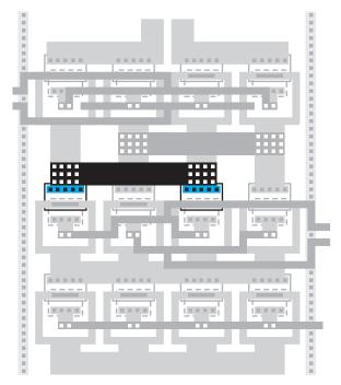
*Figure CS2–38.* Forced to jump up into Metal Two (highlighted) to connect two halves of the device QL1.
