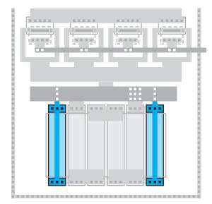
*Figure CS2–34.* Two dummies to help the four circuit resistors etch identically.
