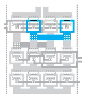
Figure CS2–46. Connecting QU3 and QU4 to the Lower Pair. Jumping across horizontally we will use Metal Two.
