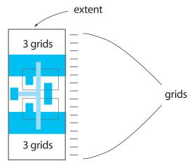
Figure 2–24. Inverter cell using 3-grid routing channels.
