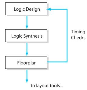
Figure 1–7. The floorplan/timing loop.
