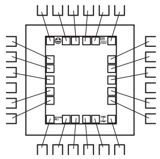
Figure CS1-93. Final chip bonding diagram.
