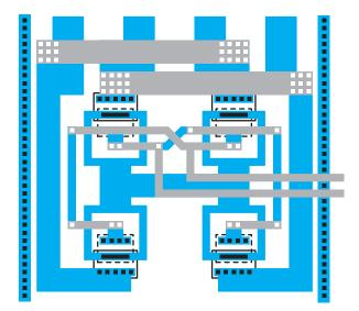
Figure CS2-60. Finished view of cross-quad of Lower Pair.
