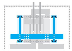
*Figure CS2–57. Dummy resistors placed to improve matching of inner resistors.*
