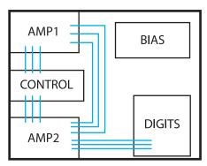
Figure 7–9. Better layout avoids cross wiring, keeps wires shorter.
