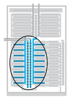
Figure CS1–25. M3 and M4 are to be cross-quaded. How do you crossquad two devices? Also notice the amplifier input and outputs are running alongside each other.
