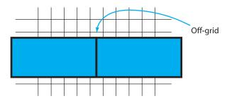
*Figure 11–3.* Our shapes are butted together, but off-grid. They won't be able to go that far if the program rounds to the inside gridline.
