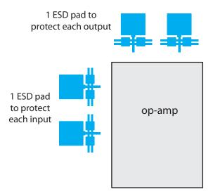
Figure CS1-76. Initial placement of op-amp and protection devices.
