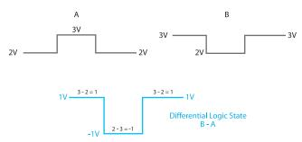
*Figure 5–21.* Differential logic. Low and high are determined by the difference between two voltages.
