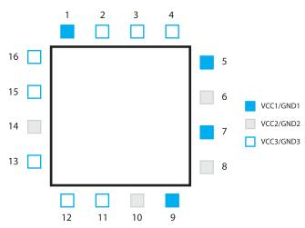
Figure 7-6. Scattered pins on the same protect circuit.
