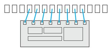
Figure 9–19. Improved pad spacing.
