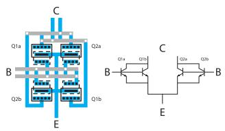
Figure 5–16. Cross-quad Bipolar transistor layout.
