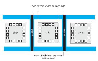
*Figure 9–26. Final chip size is just short of the step and repeat dimension, by the width of the saw blade.*
