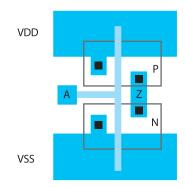
*Figure 2–9. Standard inverter cell. How can we guarantee good hookups for this cell if wires only exist on given gridlines?*
