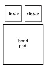
Figure CS1-66. Space-saving placement of diodes and pad.
