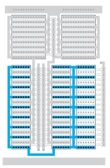
*Figure CS1–20.* Merged metal connection of differential pair and current source device.
