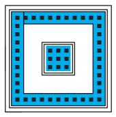
Figure CS1-64. ESD diode layout.
