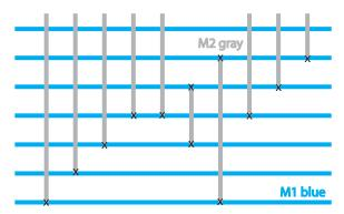
*Figure 2–4. Technique allowing wires to run in complex knots using only two metals, without becoming trapped. Metal One runs horizontally only. Metal Two runs vertically only.*
