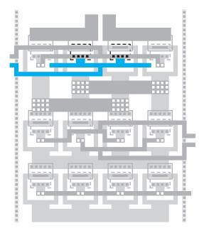
*Figure CS2–49.* Bases of QU2 and QU3 easily connect. Extensions are added to try to even the parasitics with the other diff pair.
