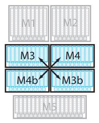
Figure CS1-30. Input devices split to allow cross-quading.
