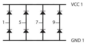
Figure 7-3. Pins 1, 5, 7, and 9 protected to VCC1 and GND1.
