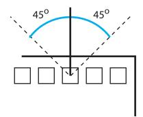
*Figure 9–14.* A maximum deviation of 45 degrees in either direction helps keeps wires to themselves.
