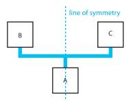
Figure 5–19. Imaginary line of symmetry helps components match.
