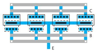
Figure 5–17. Poor man's cross-quad.
