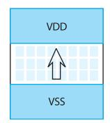
*Figure 2–18.* Power and ground rails are placed all the way to the extents of your cell. The middle is full of transistors.
