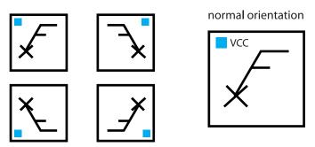
Figure CS1-85. Op-amp placement and orientation.
