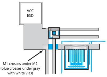
Figure CS1-82. Op-amp VCC connection to bond pad.
