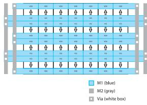
Figure 2–20. Typical power ring using Metal Two buses.
