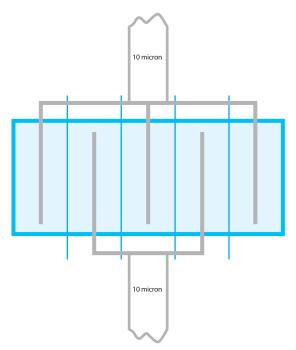
Figure 3–4. Routing the wire through the top of the device.
