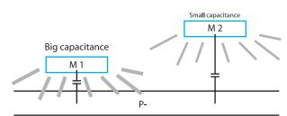
*Figure 4–3.* Usually, closer metals have larger capacitance to substrate.
