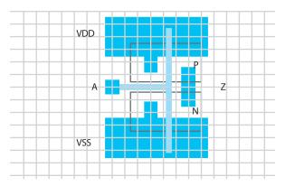
*Figure 2–10.* Grid system overlaid on our standardized inverter. Notice that the input and output align with gridlines. This cell will work with an automated wiring program.
