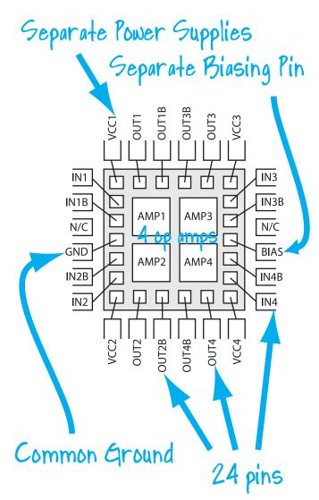
Figure CS1-1. Bond-out design using a 24-pin package.
