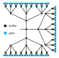
*Figure 1–3.* Large nets are broken into many smaller sections that can more easily be driven.
