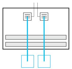
*Figure 7–13.* Would you settle for this choice? Pads are wired to two transistors high in the block.
