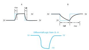
*Figure 5–25. Realistic wave forms, showing time constant delays. The differential signal almost never flattens out to a constant low value.*
