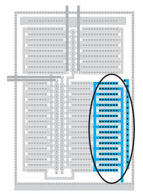
*Figure CS1–26.* Rotating M5 by 90 degrees would allow better current flow from the far end of the device.
