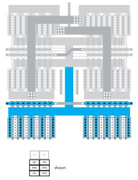
Figure CS1-46. Common wire complete and gates joined in M2.
