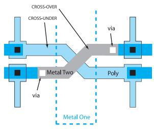
Figure CS1-40. Close-up of the center cross-over/cross-under.
