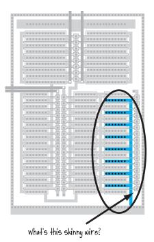
*Figure CS1–24. Ted spots a potential problem. The wire will not handle the current.*
