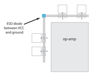
Figure CS1-79. Placement of supply protection diode.
