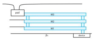
*Figure 4–12.* Cross-section. Running three metals in parallel to save real estate and reduce series resistance.
