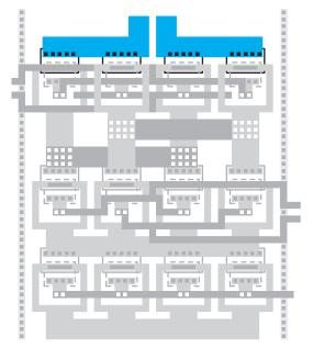
Figure CS2-47. Connecting collectors using widened wires.
