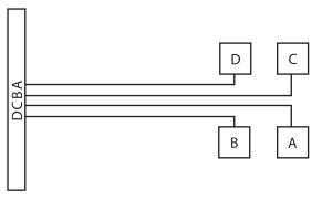
*Figure 10–23.* Nice symmetry and organization can disguise an error. DCBA to DCBA, what's the problem?
