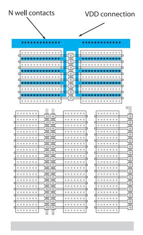
Figure CS1–13. Connecting VDD's in devices M1 and M2.
