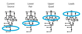
Figure CS2-3. Our mixer is made of four sections.
