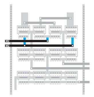
Figure CS2-18. Running input signals to two diff pairs.
