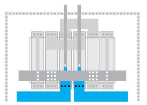
*Figure CS2–54.* Collectors from below connect directly to center of resistors in wide metal.
