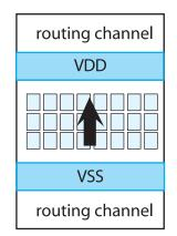
Figure 2–21. Leave room at the extent for additional wiring.
