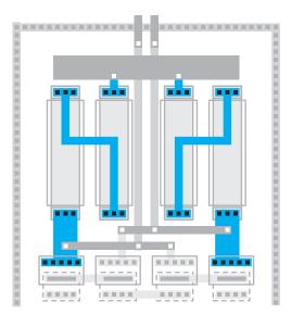
Figure CS2-24. Connecting the Load resistors.
