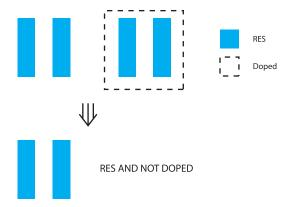
*Figure 10–8.* We ran a NOT function to eliminate the specially treated areas.
