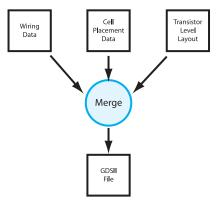
*Figure 1–13. The data is merged with the actual transistors to produce a GDSII stream file.*
