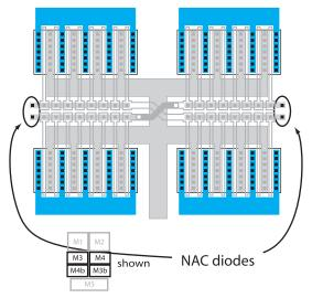
Figure CS1-41. Source-drains that need to be connected.
