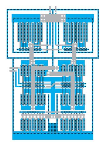
Figure CS1–57. One finished op-amp. Most excellent layout.
