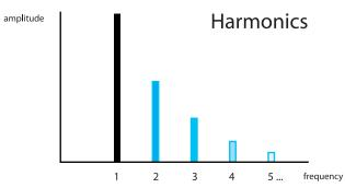
Figure 6–17. Fundamental Frequency and The Harmonics. (Sounds like a good name for Brian Setzer's backup band.)
