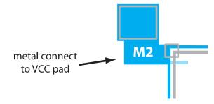
Figure CS1-81. Connection of VCC pad.
