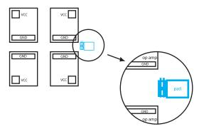
Figure CS1–90. ESD protection for bias pin.
