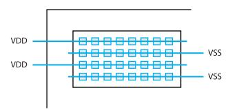
Figure 1–9. Power rails running through our gates.
