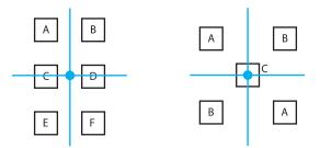
Figure 5–13. More examples of common centroid placement.
