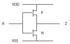
**Figure 2–8.** Schematic reference for our standard inverter cell. We need input A and output Z to align perfectly with our grid wires, or they will miss the connections placed by the auto-router.
