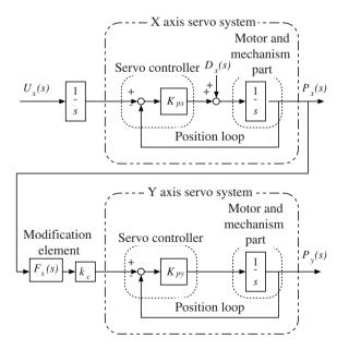
Fig. 7.1. Block diagram of master-slave synchronous positioning control method
