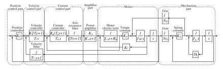
Fig. 1.1. Construction of position control system of one-axis mechatronic servo system
