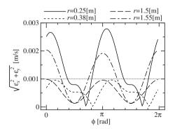
Fig. 2.15. Working linearized approximation error for various movement direction  $\phi$ , initial position of robot arm r (r = 0.25[m], r = 0.38[m], r = 1.5[m], r = 1.55[m])
