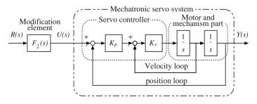
Fig. 6.3. Block diagram of the modified taught data method based on the 2nd order model  $\mathbf{F}$
