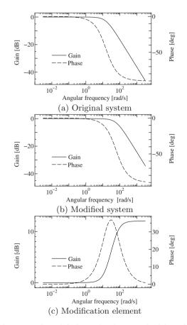
Fig. 6.4. Bode diagram of modified taught data method based on the 1st order model ( $K_p = 15[1/s], \gamma = -60[1/s]$ )
