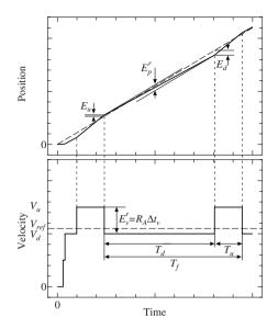
Fig. 4.8. Deterioration of ramp response in software servo system
