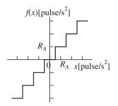
Fig. 4.6. Quantization of angular acceleration
