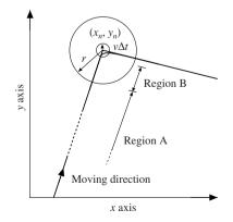
Fig. 7.10. Contour control at the corner part
