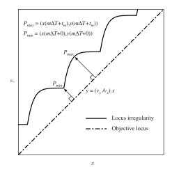
Fig. 3.7. Locus irregularity in mechatronic servo system
