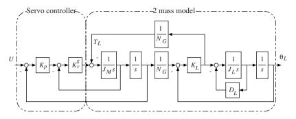
Fig. 2.2. Block diagram of 4th order model of industrial mechatronic servo system
