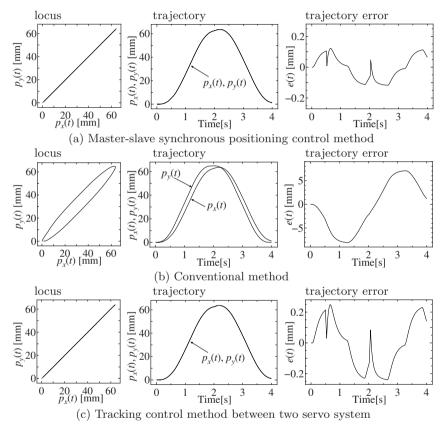
Fig. 7.4. Simulation results on step disturbance
