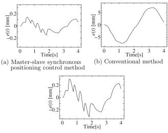
(c) Tracking control method between two servo systems
