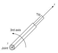
Fig. 2.17. Three-degree-of-freedom robot arm x axis and the third axis
