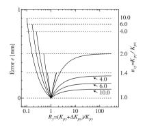
Fig. 7.11. The relationship between the locus error e and the modeling error rate  $R_y$
