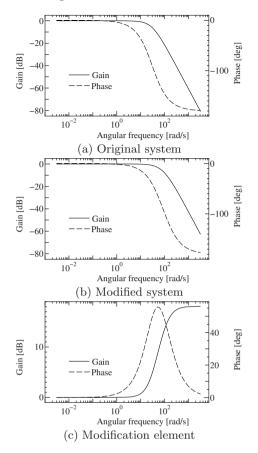
Fig. 6.5. Bode diagram of modified taught data method based on the 2nd order model ( $K_p = 15[1/s], K_v = 60[1/s], \gamma_1 = \gamma_2 = -60[1/s], \mu = -120[1/s]$ )
