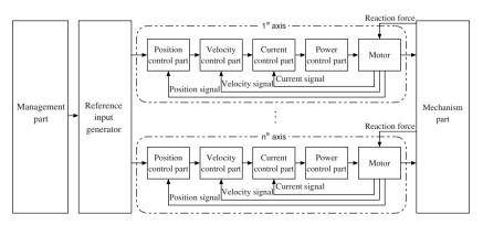
Fig. 2.1. Industrial mechatronic servo system structure
