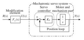
Fig. 6.2. Block diagram of the modified taught data method based on the 1st order model
