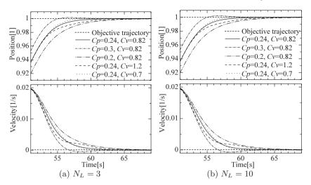
**Fig. 2.5.** Simulation results of normalized 4th order model as equation (2.15) with various  $c_p and c_v \ c_p = 0.24, \ c_v = 0.82; \ c_p = 0.3, \ c_v = 0.82; \ c_p = 0.24, \ c_v = 0.82; \ c_p = 0.24, \ c_v = 0.7$ , (a)  $N_L = 3$ , (b)  $N_L = 10$ .
