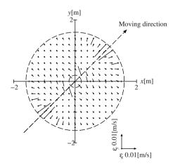
Fig. 2.14. Working linearized approximation error for various initial position (bullet •: initial position of robot arm; division from bullet •: working linearized approximation error vector  $(\varepsilon_x, \varepsilon_y)$ )
