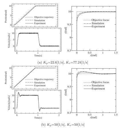
Fig. 2.6. Experimental results by using DEC-1 experiment device and comparison with simulation results by using 4th order model
