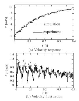
Fig. 3.6. Experimental results using DEC-1 and simulation results using 2nd order model
