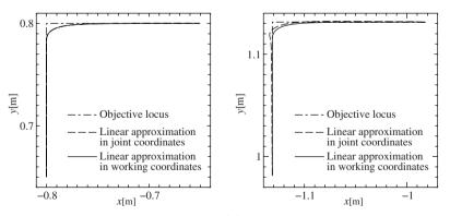
(a) Inside of working linearizable region (b) Outside of working linearizable region
