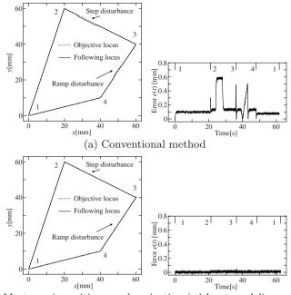
(b) Master-axis position synchronization (without modeling error)
