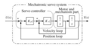
Fig. 2.8. Middle speed 2nd order model of industrial mechatronic servo system
