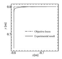
Fig. 2.19. Experimental results in the working linearizable region of the six-degreeof-freedom robot
