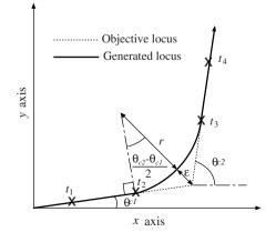
Fig. 5.7. Trajectory generation corresponding to the objective trajectory of two lines
