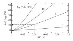
Fig. 3.5. Relation between velocity fluctuation  $e_v^s$  and reference input time interval  $\Delta T$  ( $K_v = 100[1/s]$ )
