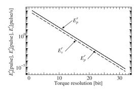
Fig. 4.9. Relation between the resolution of A/D, D/A conversion and control performance
