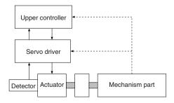
Fig. 1.3. Structure of industrial servo system
