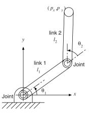
Fig. 2.11. Structure of two-degree-of-freedom articulated robot arm
