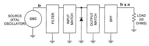
Figure 8.8 Frequency multiplication with a nonlinear element.
