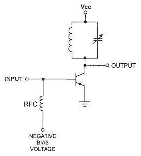
**Figure 3.70** A Class C amplifier with external bias.
