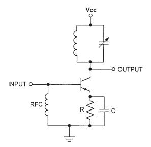
Figure 3.71 A Class C amplifier with self-bias.
