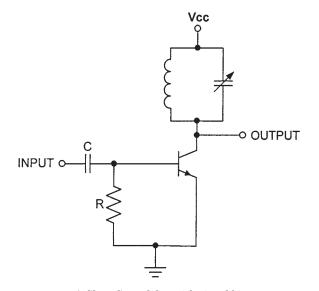
Figure 3.69 A Class C amplifier with signal bias.
