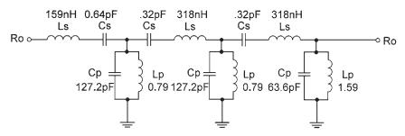
Figure 6.36 Completed 6-pole bandpass filter.
