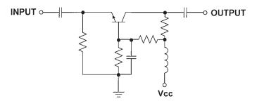
Figure 3.1 A basic common-base amplifier circuit.
