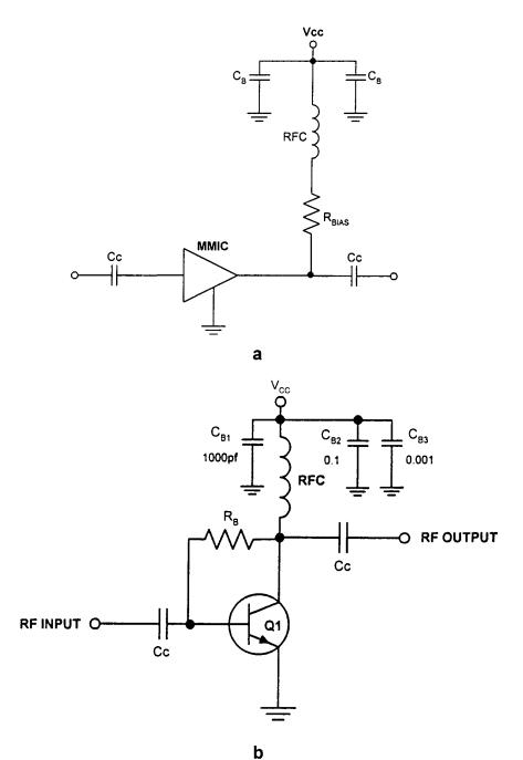
Figure 10.8 (a) Proper decoupling for a MMIC; (b) proper DC bias RF capacitor decoupling for a transistor.
