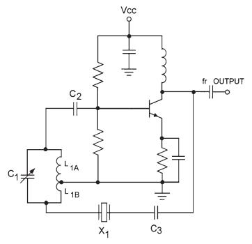
Figure 4.23 A type of Hartley crystal oscillator circuit.
