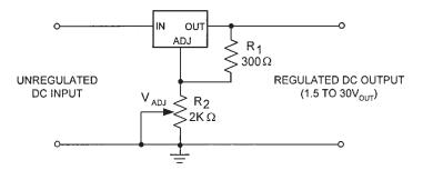
Figure 8.43 The common three-terminal (3-T) regulator with adjustable output voltage.
