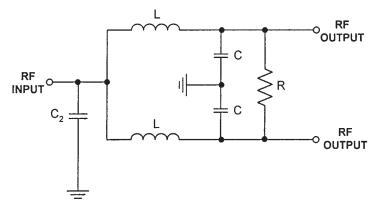
Figure 8.34 A reactive 50-ohm splitter/combiner for low loss.
