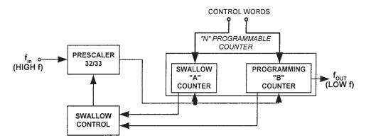
Figure 5.5 A dual-modulus prescaler for a PLL.
