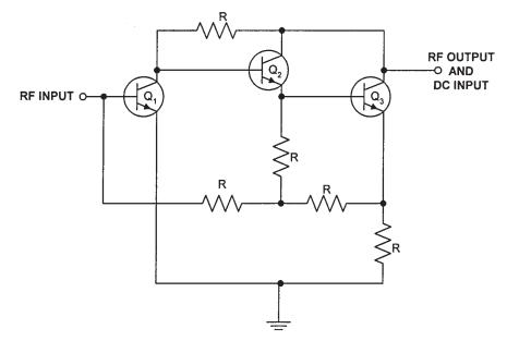
Figure 3.94 Internal circuit arrangement of an average MMIC.
