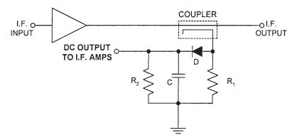
Figure 8.23 An AGC detector circuit.
