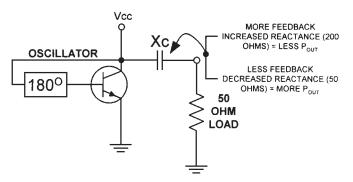
Figure 4.10 Comparisons between a high and a low coupling reactance on the output power of the oscillator.
