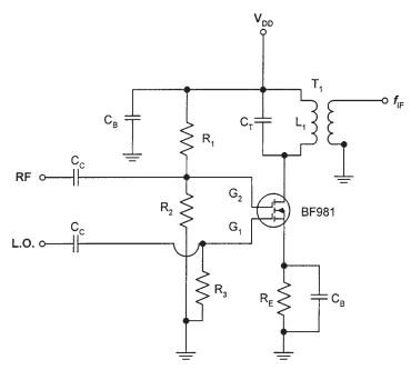
Figure 7.15 A dual-gate MOSFET mixer design.
