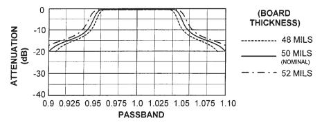
Figure 10.5 Variations in the bandwidth of a distributed filter as the board thickness is varied.
