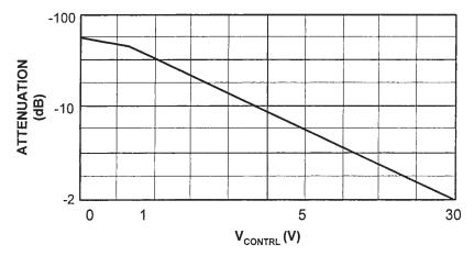
Figure 8.30 The HP (Agilent) attenuator's approximate attenuation versus control voltage ( $V_{\rm CONTRL})$  at 100 MHz.
