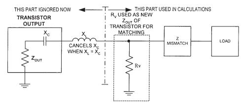
**Figure 3.49** Using a virtual resistor  $(R_{\mu})$  as the active device's temporary output resistance.
