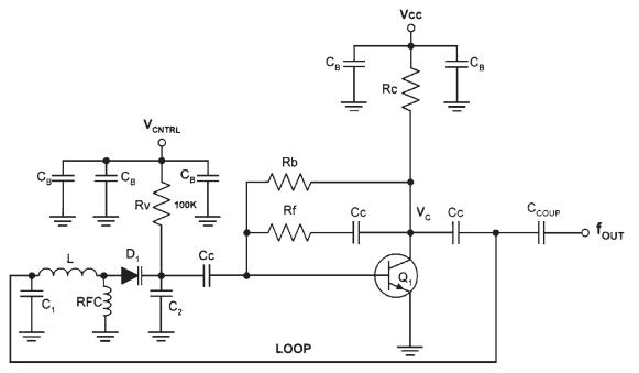
Figure 4.18 A complete bipolar VCO circuit.
