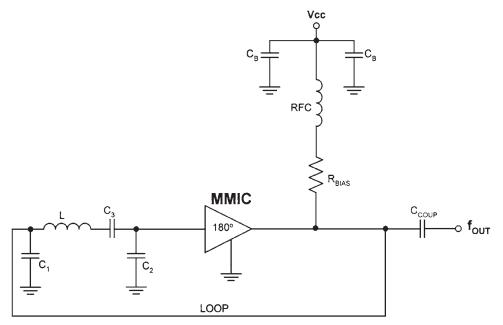
Figure 4.16 A complete MMIC LC oscillator.
