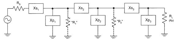
Figure 3.44 Matching for very wide bandwidths.
