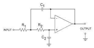
Figure 6.53 An active low-pass filter.
