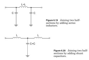
To design a low-pass filter, a half-section (as depicted in Fig. 6.16) can be calculated by:
