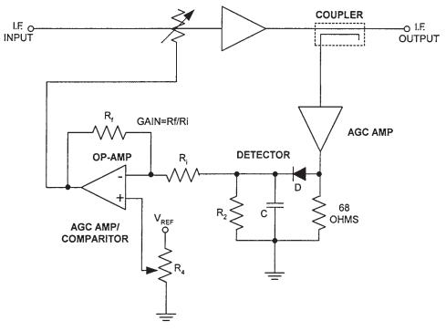
Figure 8.20 A common AGC circuit.
