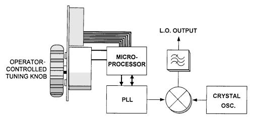
Figure 5.2 Premixing with a PLL and a crystal oscillator.
