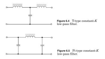
The point that  $X_L = X_C$  is called the *resonant frequency*  $(f_r)$ , and will vary depending on the values of the *LC* components. The series resonant frequency can be calculated by:
