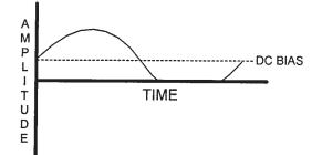
Figure 3.58 A Class AB amplifier's output waveform.
