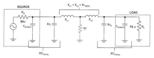
Figure 3.38 Pi network before combining calculated components.
