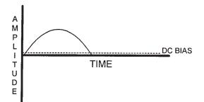
Figure 3.59 A Class B amplifier's output waveform.
