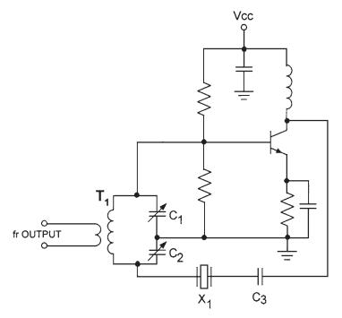
Figure 4.24 A type of Colpitts crystal oscillator circuit.
