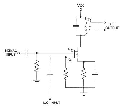
Figure 7.11 A dual-gate MOSFET mixer circuit.
