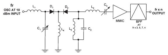
Figure 8.6 An odd-order frequency multiplier.
