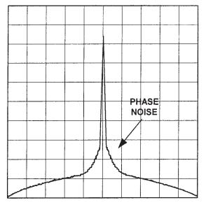
Figure 5.8 Spectra showing phase noise out of PLL.
