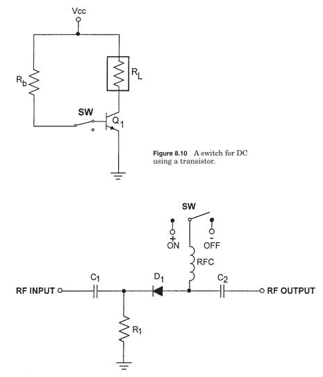
Figure 8.11 An RF switch using a diode.
