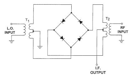
Figure 7.1 A double-balanced mixer stage.
