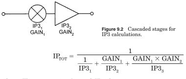
where  $IP_{TOT}$  = receiver's total IP3 from its input to its output and  $IP3_n$  and  $GAIN_n$  are linear terms, not decibels.
