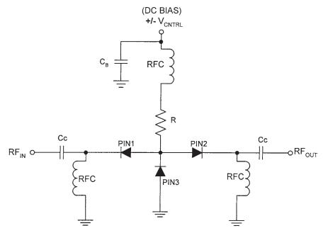
Figure 8.12 A high-isolation RF PIN diode switch.
