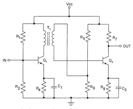
Figure 3.114 Low-frequency transformer coupling between two stages.
