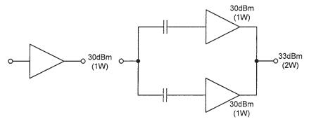
Figure 3.106 The output power of a single MMIC compared to two paralleled MMICs.
