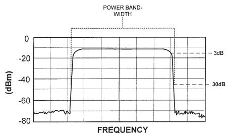
Figure 2.42 A digital signal's bandwidth for an average power measurement.
