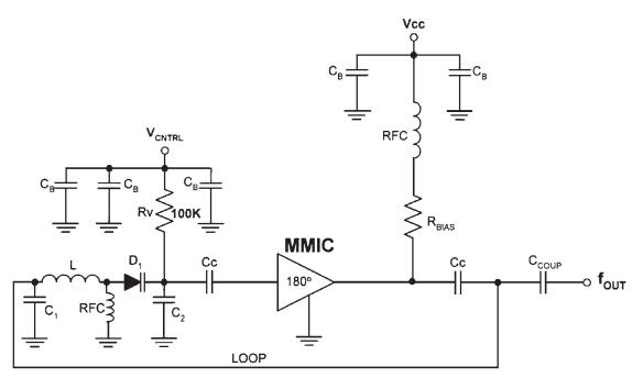
Figure 4.19 A complete MMIC VCO circuit.
