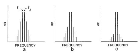
**Figure 7.7** Different mixers levels and their two-tone output spectra: (*a*) Level 7; (*b*) Level 17; (*c*) Level 23.
