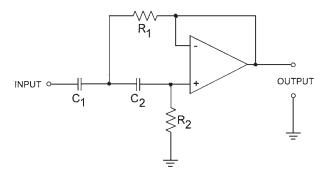
Figure 6.54 An active high-pass filter.
