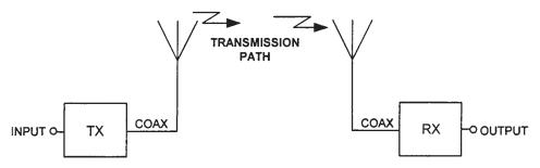
Figure 9.4 Transmitter and receiver path.
