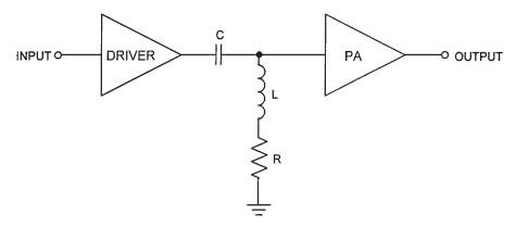
Figure 3.55 Gain flattening with an *LR* losser network.
