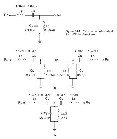
**Figure 6.35** (*a*) Two single half-sections; (*b*) combining the shunt tanks.
