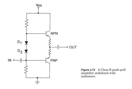
nonlinear operation, Class B can employ single-ended amplifiers fed into high-Q tuned RF circuits, with any biasing arrangement that sets the transistor at approximately 0.7 V above cutoff.
