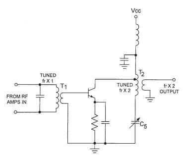
Figure 8.1 A low-frequency Class C frequency multiplier.
