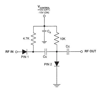
Figure 8.13 A high-isolation series/shunt PIN diode switch.
