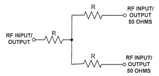
Figure 8.36 A 50-ohm resistive wideband splitter/combiner.
