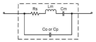
Figure 4.9 Equivalent internal structure of a crystal.
