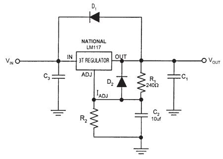
Figure 8.51 Other 3-T regulator protection circuits.
