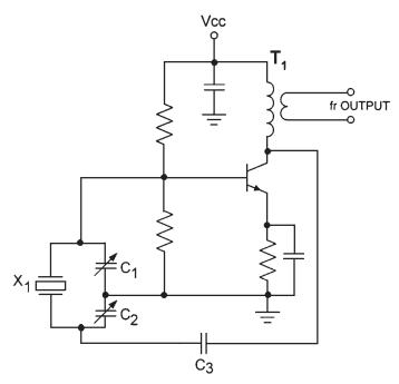
Figure 4.25 A type of Pierce crystal oscillator circuit.
