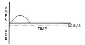
Figure 3.60 A Class C amplifier's output waveform.
