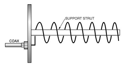
Figure 10.24 A helical circularly polarized antenna.
