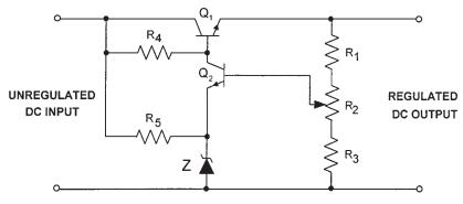
Figure 8.47 The series-pass regulator with feedback.
