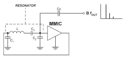
**Figure 4.22** Point B of the oscillator results in lower harmonic and fundamental outputs.
