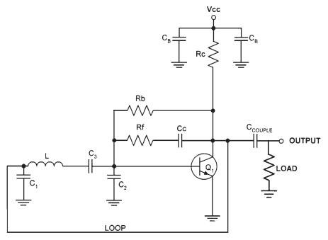
Figure 4.8 Loop closed after Bode analysis for a functionig oscillator.
