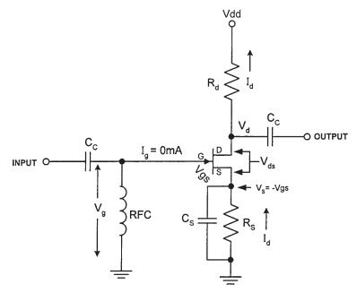
Figure 3.90 JFET biasing up to medium frequencies.
