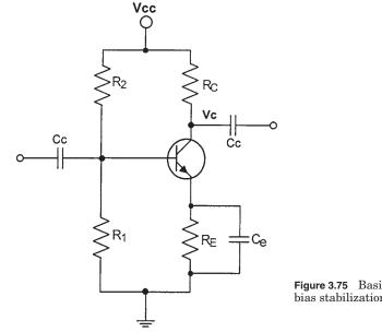
Figure 3.75 Basic C-E circuit for bias stabilization calculation.
