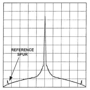
Figure 5.9 Spectra showing reference spurs out of PLL.
