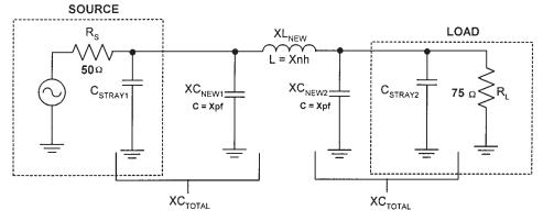
Figure 3.39 Pi matching network after combining components.
