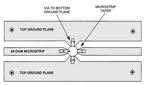
Figure 10.6 Proper board layout for a transistor as seen from top of PCB.
