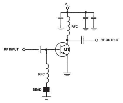
Figure 3.92 A high-frequency Class C power amplifier.
