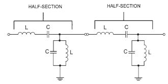
Figure 6.31 Improper way to join BPF half-sections.
