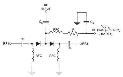
Figure 8.17 An SPDT PIN diode switch.
