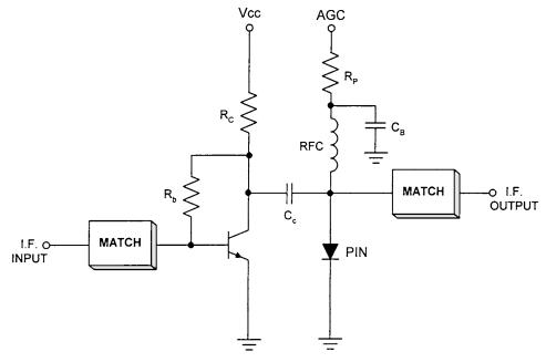
Figure 3.109 A simple but low-cost VGA circuit.
