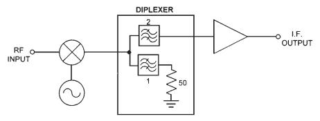
Figure 6.46 A BPF diplexer placed at the output of a conversion stage to decrease IMD.
