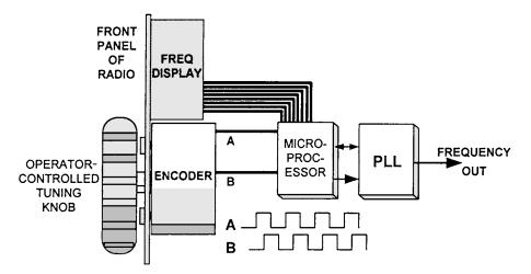
Figure 5.3 A common PLL manual tuning method.
