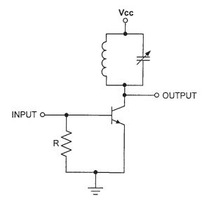
Figure 3.67 A Class C amplifier showing lack of bias.
