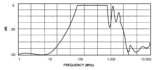
Figure 6.28 A real-life high-pass filter's frequency response.
