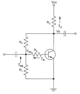
Figure 3.80 Class A HF, VHF, and UHF moderately stable amplifier design with voltage feedback.
