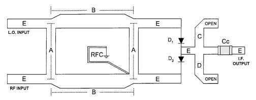
Figure 7.5 A narrowband microwave mixer for applications of UHF and above.
