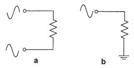
**Figure 8.31** (*a*) Balanced input; (*b*) Unbalanced input.
