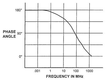
**Figure 3.4** A phase-versus-frequency graph for a commonemitter amplifier circuit.
