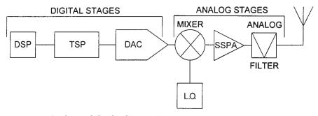
Figure 10.14 A software-defined radio transmitter.
