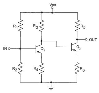
Figure 3.113 Direct coupling between two stages.
