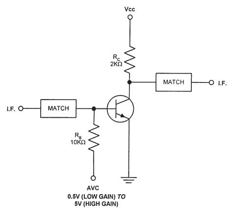
Figure 3.110 A circuit for a variable-bias gain amplifier.
