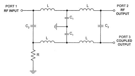
Figure 8.56 A lumped directional coupler circuit.
