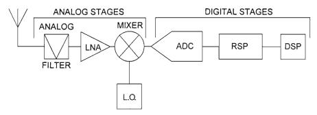
Figure 10.15 A software-defined radio receiver.
