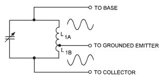
Figure 4.12 A tapped coil showing the phase relationships.
