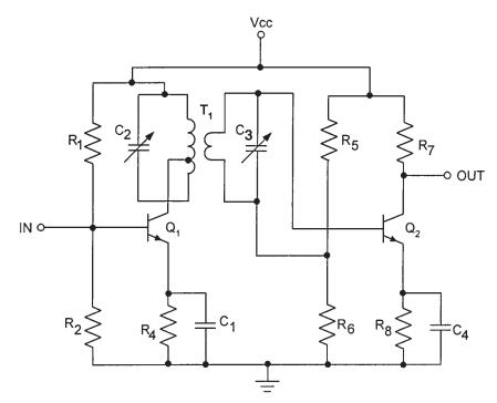
Figure 3.115 High-frequency transformer coupling between two stages.
