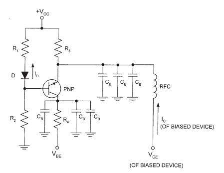
Figure 3.87 Class A active bias circuit.
