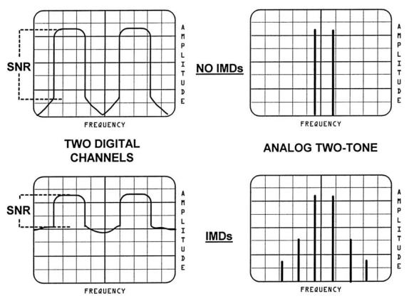
Figure 2.33 Digital signals as affected by IMD, along with a standard CW two-tone display for comparison.
