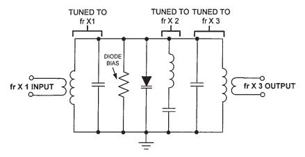
Figure 8.3 A varactor frequency multiplier circuit.
