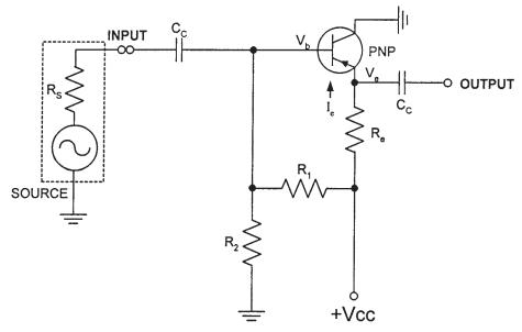
Figure 3.83 A common-collector buffer circuit.
