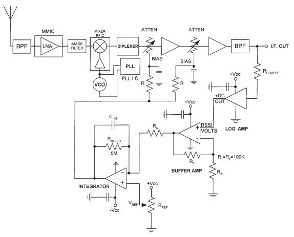
Figure 8.21 A log amp used in a receiver's AGC circuit.
