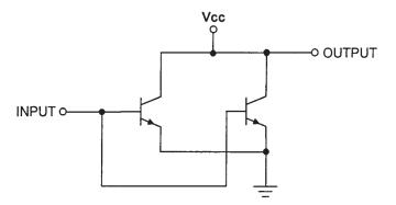
Figure 3.104 A parallel amplifier circuit without bias components.
