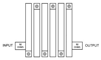
Figure 6.40 Sixth-order interdigital distributed BP filter.
