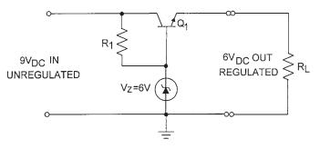
Figure 8.46 A series-pass transistor regulator.
