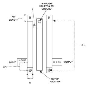
Figure 6.44 Third-order interdigital distributed BP filter design.
