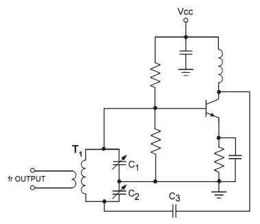
Figure 4.13 A type of *LC* Colpitts oscillator.
