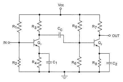
Figure 3.111 Capacitive coupling between two stages.
