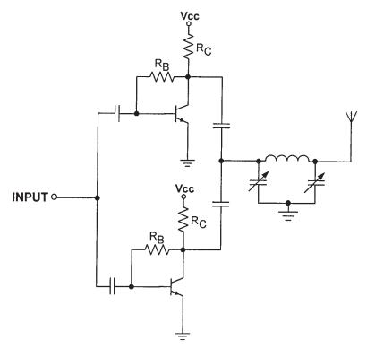
Figure 3.105 A parallel power amplifier with bias components.
