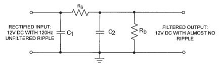
Figure 8.41 A type of power supply filter using a series resistor.
