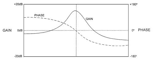
Figure 4.5 Bode plot of oscillator gain and phase.
