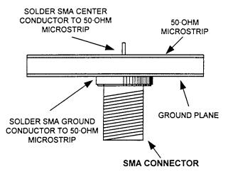
Figure 10.13 SMD connector board-mounted on top of ground plane.
