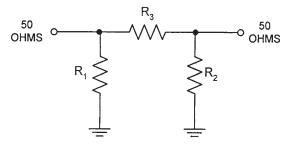
Figure 8.27 A 50-ohm pi attenuator.
