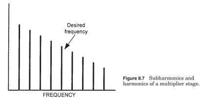
action of multiplication. However, Schottky diodes will not have this increased noise problem: Doubler and tripler topologies using low-noise Schottky diodes can usually maintain a good 20 log N phase noise degradation, even up to  $\times 7$ . Varactor multipliers (Fig. 8.8) can be delicate to tune for top performance, but they too add very low levels of phase and amplitude noise beyond the unavoidable 20 log N.
