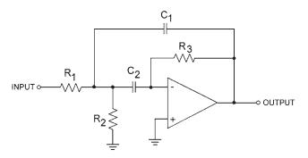
Figure 6.55 An active bandpass filter.
