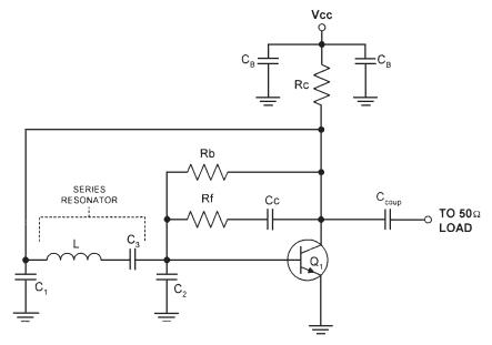
Figure 4.15 An LC oscillator design good to 500 MHz.
