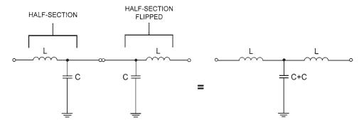
Figure 6.21 One way of properly combining half-sections.
