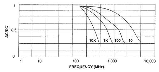
Figure 10.11 Ratio of resistance at DC to resistance at AC at different frequencies for standard SMD resistors.
