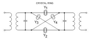
Figure 6.50 A crystal-lattice BPF circuit.
