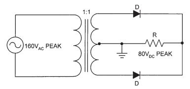
Figure 8.39 A full-wave rectifier circuit.
