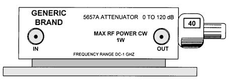
Figure 8.25 A common manually switched step attenuator.
