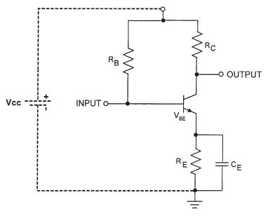
**Figure 3.62** A C-E amplifier displaying its  $V_{CC}$  connection.
