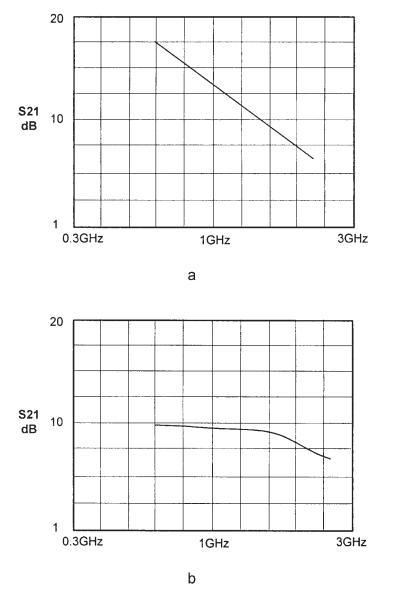
Figure 3.100 Gain flattening of an RF amplifier: (a) not compensated; (b) compensated.
