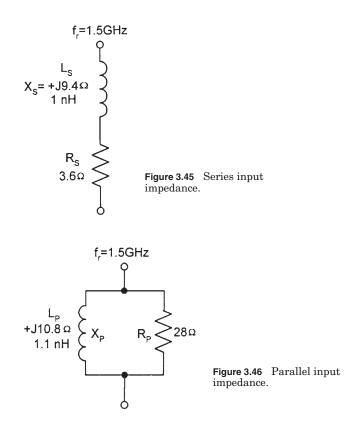
where  $R_p$  = equivalent parallel resistance, ohms  $R_s$  = series resistance, ohms  $X_s$  = series reactance, ohms  $X_p$  = equivalent parallel reactance, ohms
