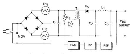
Figure 8.44 A switching-mode power supply.
