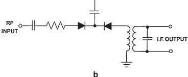
**Figure 7.2** (*a*) A single-diode mixer and a (*b*) double-diode mixer stage.
