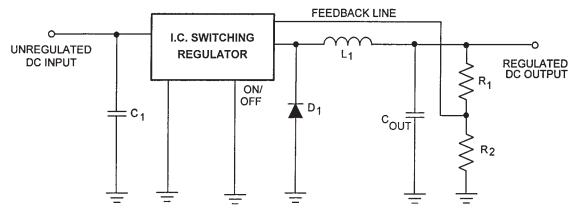
Figure 8.49 A switching regulator integrated circuit with support components.
