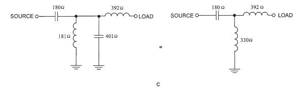
Figure 3.42 The T network and its various legal configurations before and after combination.
