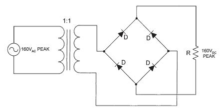
Figure 8.40 A bridge rectifier circuit.
