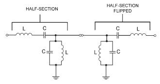
Figure 6.30 Proper way to join BPF half-sections.
