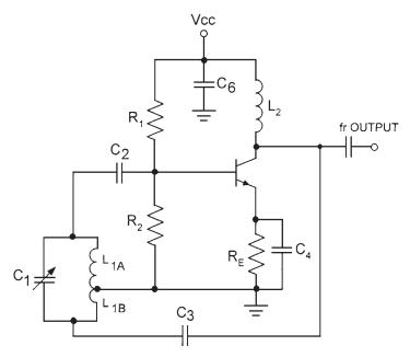
Figure 4.11 A type of *LC* Hartley oscillator.
