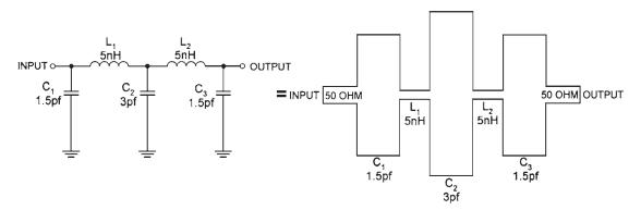
Figure 6.45 Lumped low-pass filter structure and distributed equivalent.
