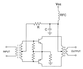
Figure 3.72 A Class B push-pull amplifier.
