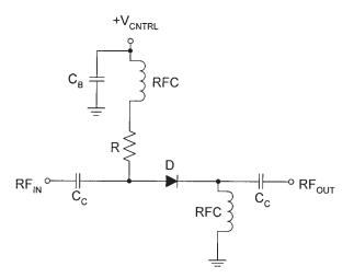
Figure 8.16 A low parts count PIN diode switch.
