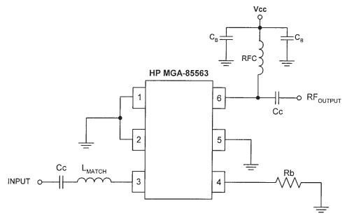
Figure 3.96 Agilent (HP) voltage-biased LNA MMIC.
