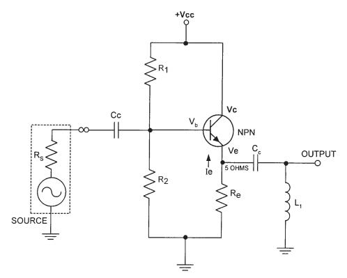
Figure 3.84 Another common-collector buffer circuit.
