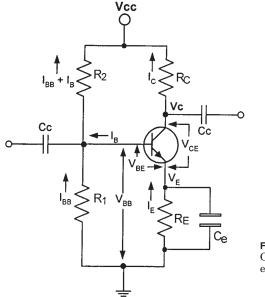
**Figure 3.81** A low-frequency Class A amplifier for bias design example.
