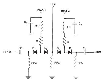
Figure 8.14 A wideband, low-distortion SPDT PIN diode switch.
