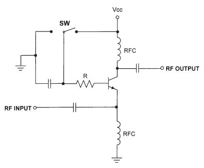
Figure 8.9 An RF switch using a transistor.
