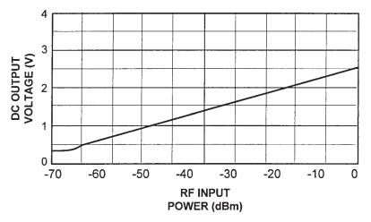
Figure 8.22 A log amp's DC output versus RF input power.
