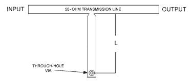
Figure 6.41 Proper distributed component length to ground via.
