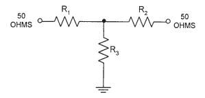
Figure 8.28 A 50-ohm T attenuator.
