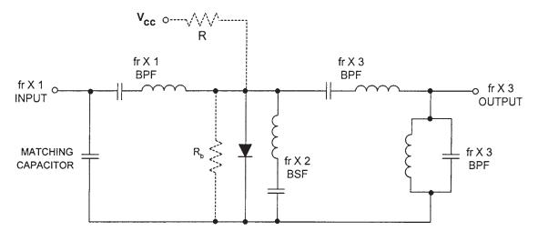
Figure 8.4 A harmonic generator for frequency multiplication showing two different diode bias methods, R<sub>b</sub> and V<sub>cc</sub>.
