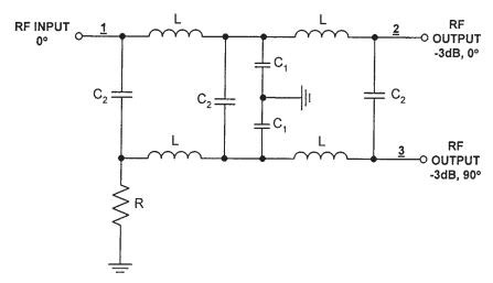
Figure 8.35 A lumped 90 degree directional coupler.
