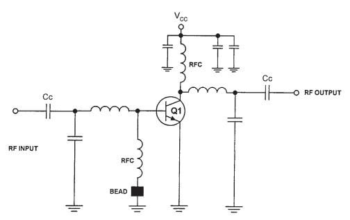
Figure 3.53 Class C power amplifier with matching networks and bias and decoupling circuits.
