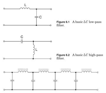
Figure 6.3 An 8-pole low-pass filter.
