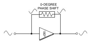
Figure 4.2 An amplifier with degenerative feedback cannot oscillate.
