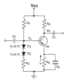
**Figure 3.79** Class A diodetemperature-stabilized amplifier for bias calculations.
