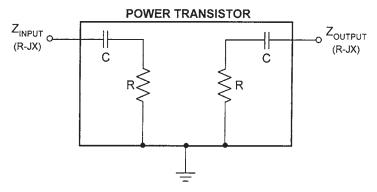
Figure 3.52 The complex series impedance of a power transistor.
