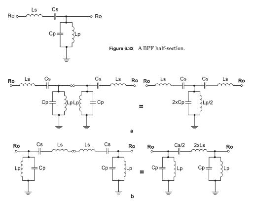
Figure 6.33 Combining two BPF half-sections when placed (a) tank-to-tank and (b) series-to-series.
