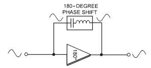
**Figure 4.3** An amplifier with regenerative feedback can oscillate.
