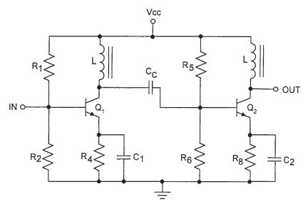
Figure 3.112 Inductive coupling between two stages.
