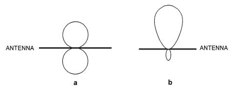
**Figure 10.21** The radiation patterns of (a) a dipole antenna and (b) a Yagi antenna.
