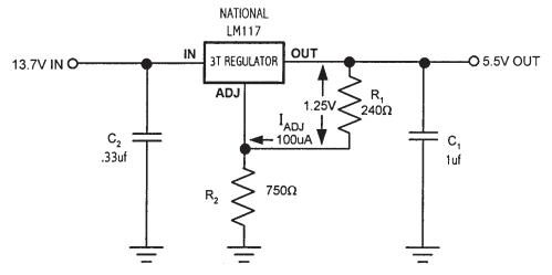
Figure 8.50 3-T regulator set for 5.5-V output.
