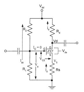
**Figure 3.91** A low-frequency Class A JFET bias circuit.
