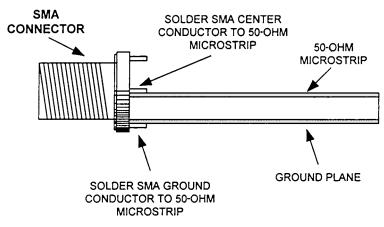
Figure 10.12 SMD connector edge-board-mounted.
