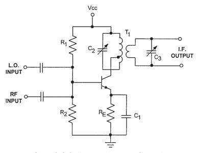
Figure 7.12 One method of using a transistor as a nonlinear mixer stage.
