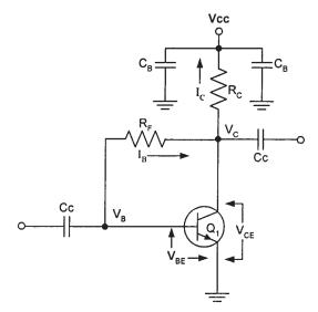
Figure 3.82 A Class A high-frequency amplifier.
