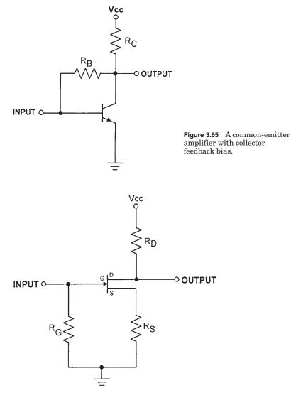
Figure 3.66 Class A source-biased FET amplifier.
