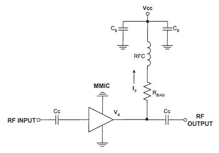
Figure 3.95 Standard MMIC gain block with biasing.
