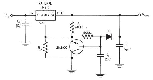
Figure 8.52 3-T regulator for slow-turn-on applications.
