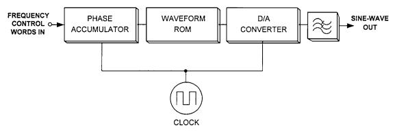
Figure 5.11 A DDS frequency synthesizer circuit.
