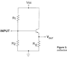
Figure 3.5 A typical commoncollector amplifier circuit.
