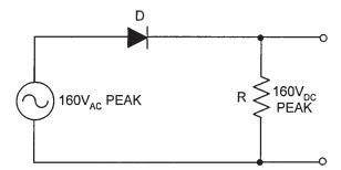
Figure 8.38 A half-wave rectifier circuit.
