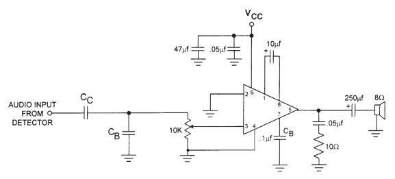
Figure 3.108 An integrated circuit audio power amplifier.
