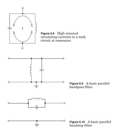
But *LC* filters are low in cost and can fit into a tight form factor (as opposed to distributed designs). They are not suitable for very tight bandwidth requirements that demand steep skirts.
