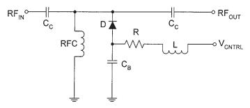
Figure 8.15 A shunt PIN diode switch.
