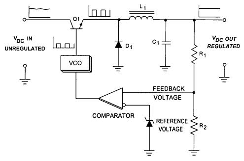
Figure 8.48 Switching regulator operation.
