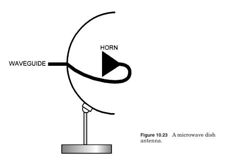
the actual size of the dish, with its diameter being about 10 times its wavelength of interest for high gain, low loss, and extreme directivity.
