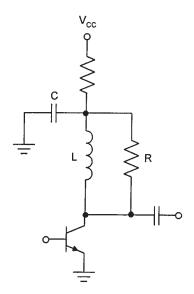
**Figure 3.101** A collector inductor load for decreasing low-frequency oscillations.
