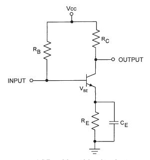
**Figure 3.61** A C-E amplifier with base-biased emitter feedback biasing.
