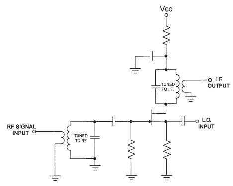
Figure 7.10 A single-ended JFET mixer circuit.
