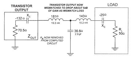
Figure 3.51 The completed mismatched amplifier with our desired gain.
