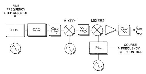
Figure 5.12 A method of synthesizing new frequencies with direct digital synthesis.
