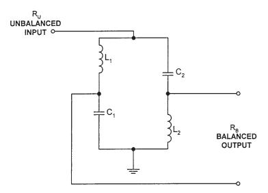
Figure 8.32 Narrowband balun structure.
