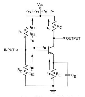
**Figure 3.63** A voltage divider emitter feedback-biased C-E amplifier with current flow.
