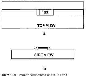
**Figure 10.9** Proper component width (a) and component soldering (b) for decreased reflections.
