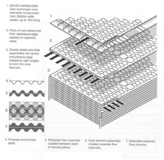
Figure 2.1.11 - Core Structure of a Bavex unit
