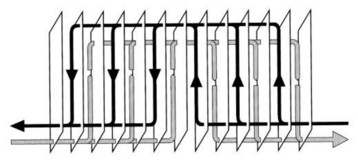
Figure 2.1.3 – A Two-Pass Plate and Frame Flow Arrangement
