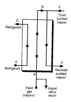
Figure 2.2.4 – Plate-Fin Heat Exchanger Dephlegmator Arrangement
