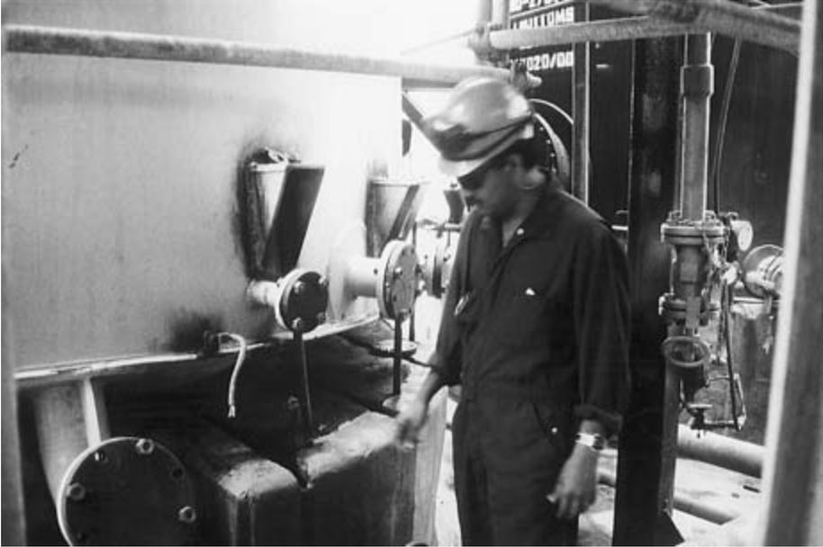
FIGURE 3-3 Tank bottom is bulged during a hydrotest.
