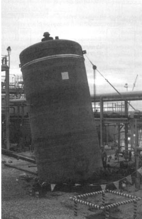
FIGURE 5-12 A large acid tank fails due to blocked vent and a blocked overflow line.
