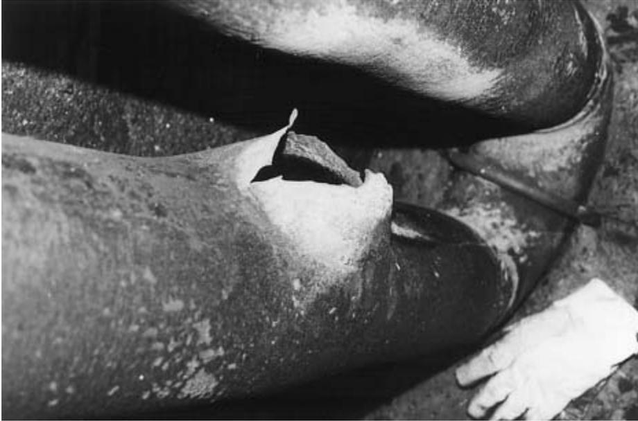
FIGURE 6-2 Tube rupture in a fired heater.
