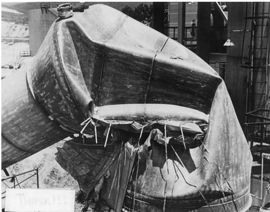
FIGURE 3-7 A close-up of a collapsed stripper column.
