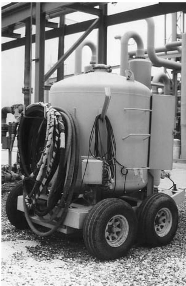
FIGURE 8-4 Repairs to a portable sandblast pot do not meet specifications and the lid flies off.
