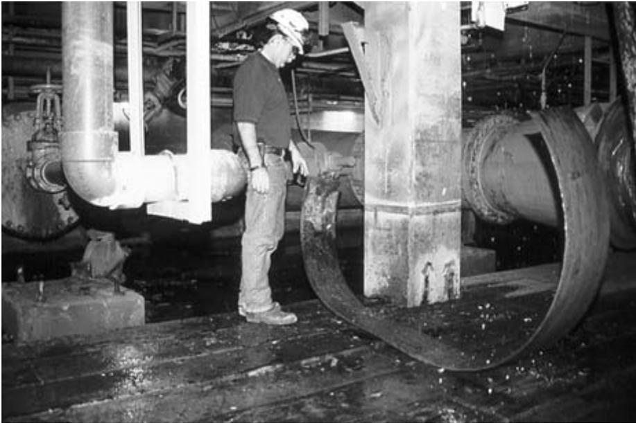
FIGURE 7-10 Photo of how the pump pipe coupling yielded during the explosion.
