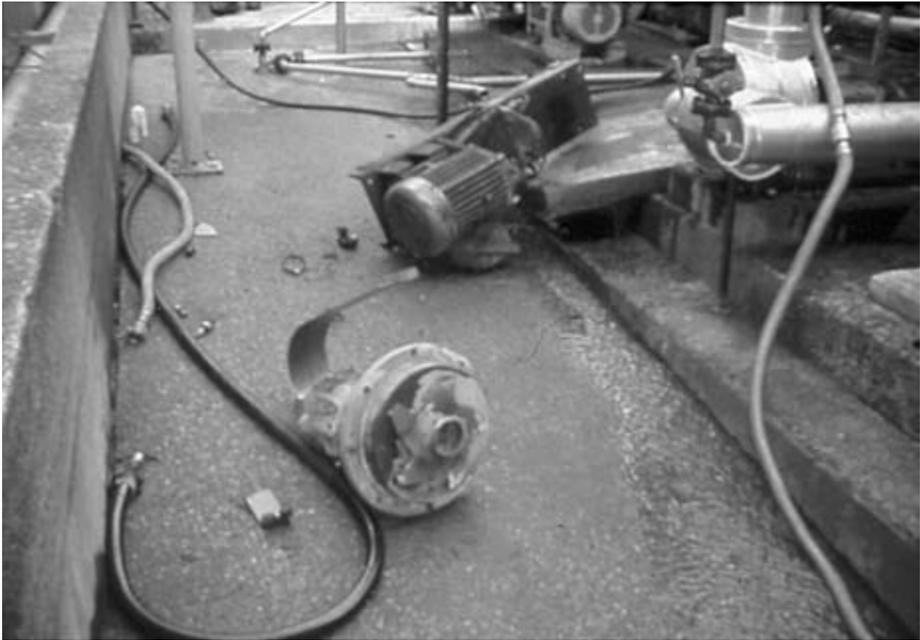
FIGURE 7-14 Pump base plate and motor as well as the position of the bearing housing with impeller document the explosion. Courtesy of Eastman Chemical Company.
