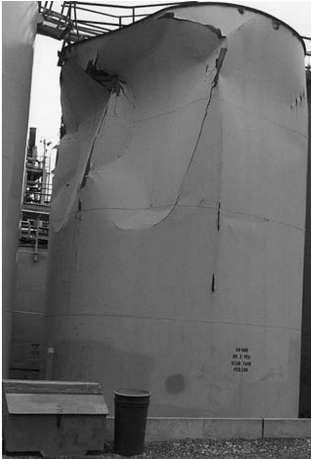
FIGURE 2-13 A 12-ft.-diameter tank ruined after vent system is improved.
