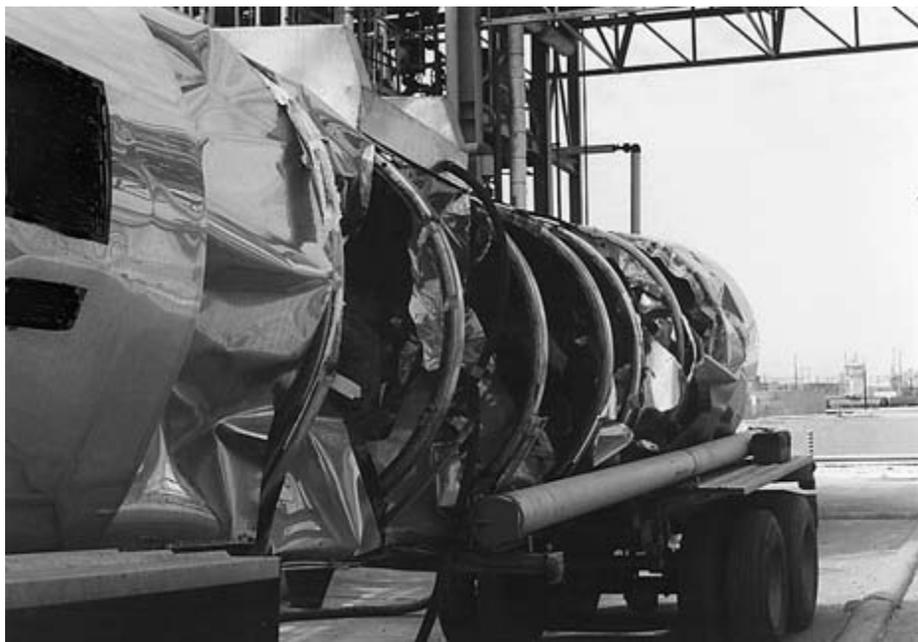
FIGURE 2-5 Close-up of tank failure and exposed ribs.
