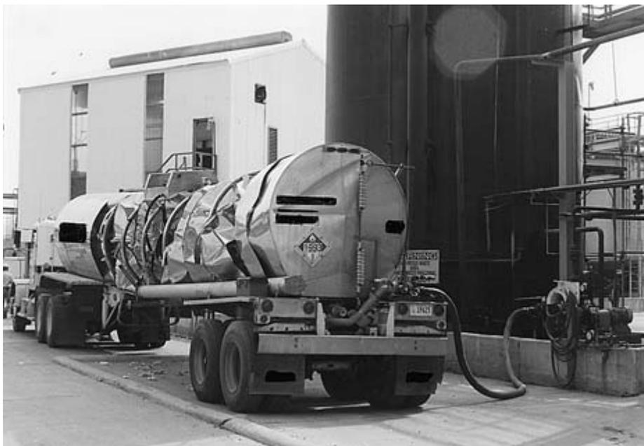
FIGURE 2-2 Collapsed tank truck with unloading hose connected.
