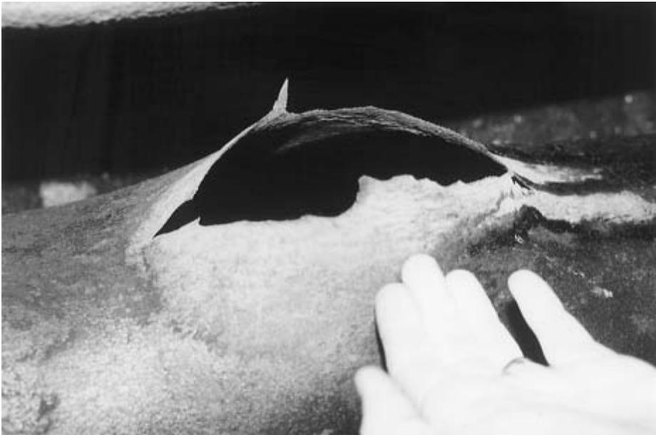
FIGURE 6-3 Close-up of the tube failure.
