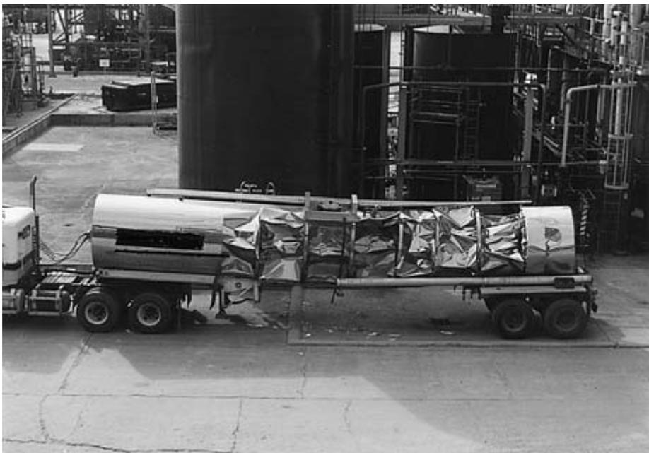
FIGURE 2-4 Side view of collapsed tank truck.
