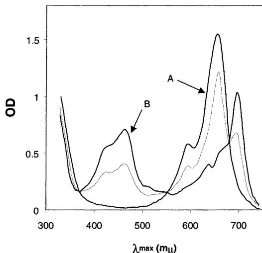
**Figure 7.** Visible spectra of cobalt phthalocyanine under CCT conditions in HMPA demonstrating the reduction to  $\text{Co}^{\text{I}}$ .<sup>187</sup> A and B are before and after polymerization.
