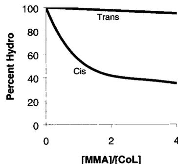
**Figure 8.** Hydrogen/deuterium dependence at the  $\beta$ -carbon atom of (TAP)Co–(3-tetrahydrofuranyl) on the concentration of MMA-*d*<sub>8</sub> relative to cobalt.<sup>197</sup>
