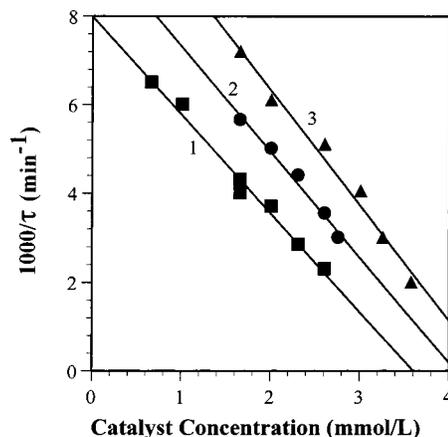
**Figure 3.** Dependence of reciprocal time of the maximum polymerization rate on the concentration of catalyst for  $Co^{II}$ -mesoporphyrin-II (1),  $Co^{III}$ (pyridine)bis(dimethylglyoximate) iodide (2), and  $Co^{II}$ tetra-*tert*-butylbenzoporphyrin (3).
