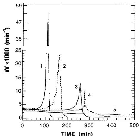
**Figure 1.** Temporal dependence of the rate of polymerization of bulk MMA under CCT conditions.
