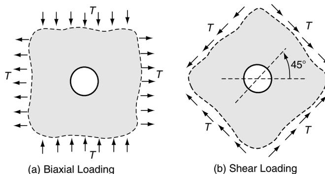
FIGURE 8-15 Stress-free hole under biaxial and shear loading.
