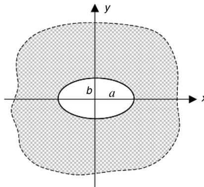
FIGURE 11-9 Elliptical hole in an infinite anisotropic plane.
