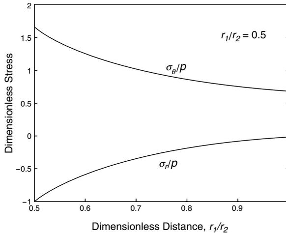
FIGURE 8-9 Stress distribution in thick-walled cylinder example.
