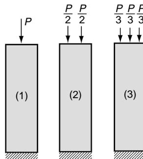
FIGURE 5-7 Statically equivalent loadings.
