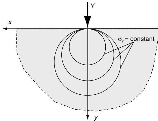
**FIGURE 8-21** Radial stress contours for the Flamant problem.
