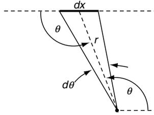
**FIGURE 8-25** Surface geometry for distributed loading example.
