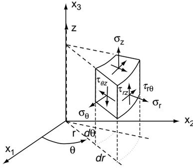
FIGURE 3-9 Stress components in cylindrical coordinates.
