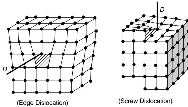
FIGURE 14-2 Schematics of edge and screw dislocations.
