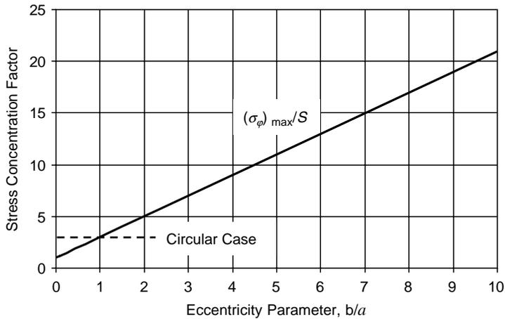
FIGURE 10-18 Stress concentration factor for elliptical hole problem.
