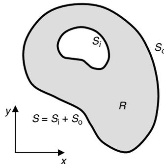
**FIGURE 7-2** Typical domain for the plane elasticity problem.
