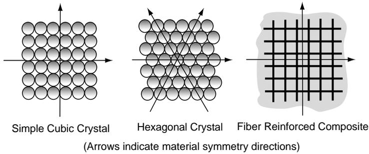
FIGURE 11-1 Material microstructures.
