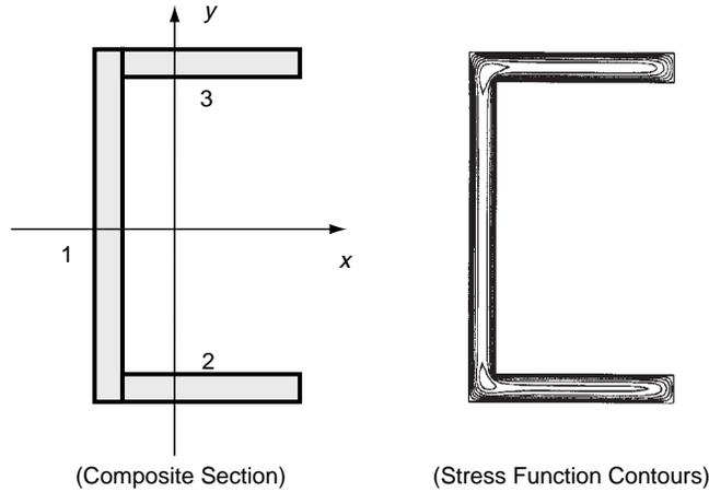
**FIGURE 9-14** Composite section of three thin rectangles.
