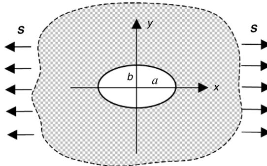
FIGURE 11-10 Infinite anisotropic plate with elliptical hole.
