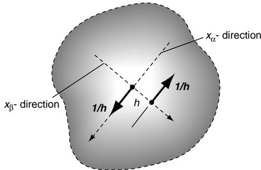
FIGURE 14-9 Double-force system with moment.
