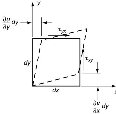
FIGURE 6-3 Shear deformation.
