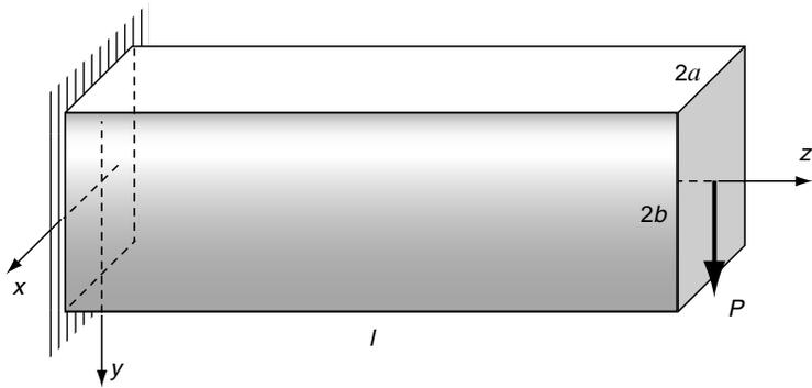
**Figure 9-21** Flexure of a beam of rectangular section.
