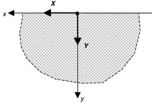
**FIGURE 11-8** Concentrated force system on a half plane.
