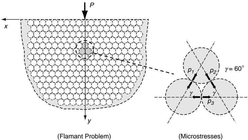
FIGURE 14-21 Flamant problem for the doublet mechanics model.
