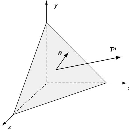
FIGURE 3-4 Traction on an oblique plane.
