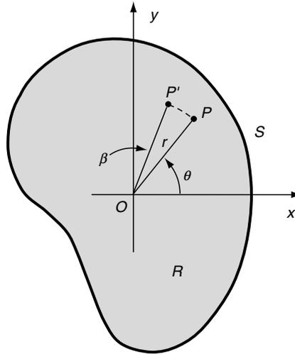
**FIGURE 9-2** *In-plane displacements for the torsion problem.*
