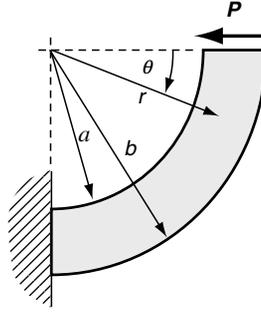
FIGURE 8-32 Curved cantilever beam with end loading.
