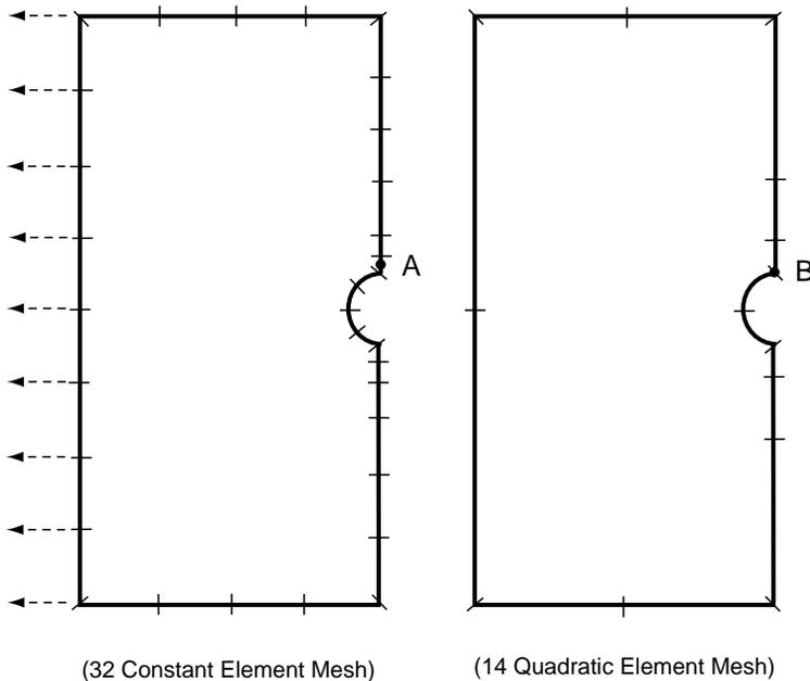
FIGURE 15-10 BEM solution of a plate under uniform tension containing a circular hole.
