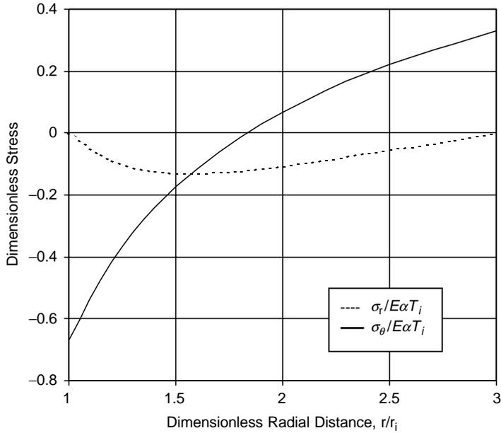
FIGURE 12-4 Stress distribution in annular plate ( $r_o/r_i = 3$ ).
