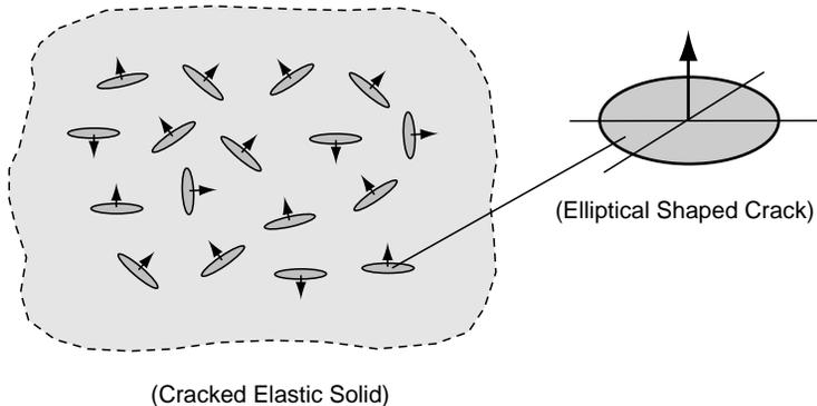
FIGURE 14-12 Elastic solid containing a distribution of cracks.
