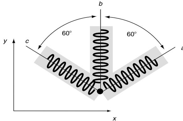
2-8\*. A two-dimensional strain field is found to be given by  $e_x = 0.002$ ,  $e_y = -0.004$ , and  $e_{xy} = 0.001$ . Incorporating the transformation relations (2.3.6) into a MATLAB code, calculate and plot the new strain components in a rotated coordinate system as a function of the rotation angle  $\theta$ . Determine the particular angles at which the new components take on maximum values.
