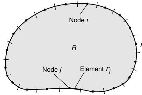
**FIGURE 15-9** Boundary discretization using elements with constant approximation.
