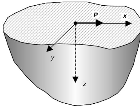
FIGURE 13-3 Cerruti's problem: tangential force on the surface of a half space.
