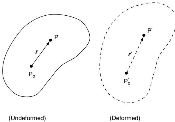
FIGURE 2-2 General deformation between two neighboring points.
