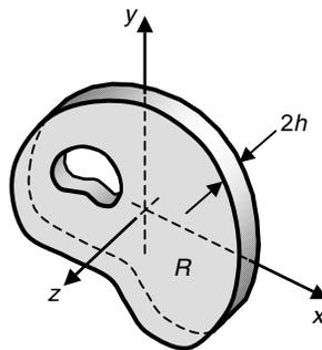
FIGURE 7-3 Thin elastic plate representing plane stress conditions.
