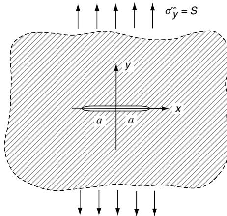
FIGURE 10-19 Central crack in an infinite plane.
