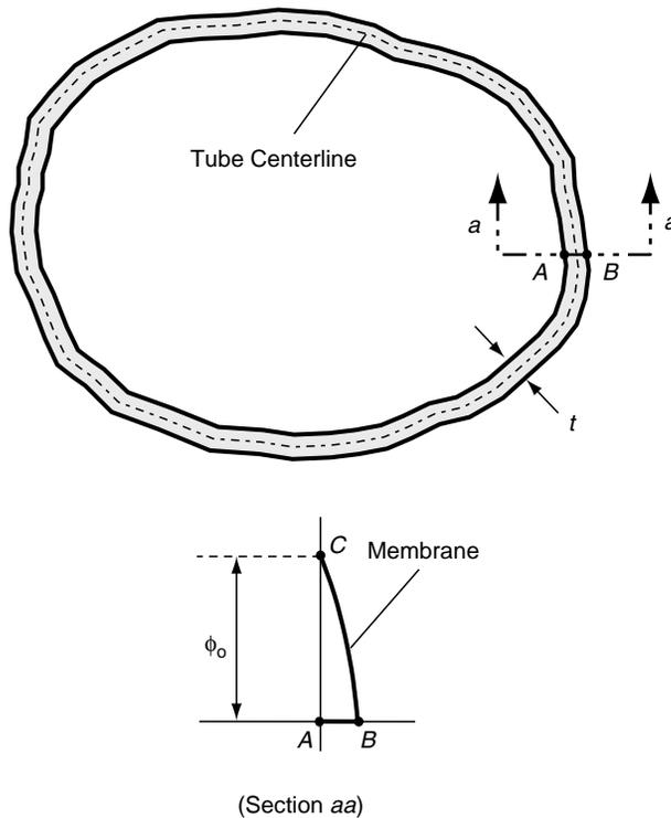
FIGURE 9-16 Thin-walled section.
