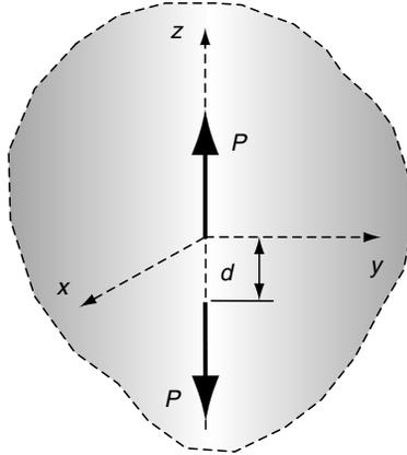
13-19. Using the results of Exercise 13-18, continue the superposition process by combining three force doublets in each of the coordinate directions. This results in a *center of dilatation* at the origin as shown in the figure. Using spherical coordinate components, show that the stress field for this problem is given by
