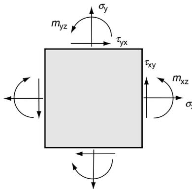
FIGURE 14-16 Couple stresses on planar element.
