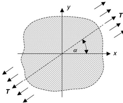
FIGURE 11-6 Uniform tension of an anisotropic plane.
