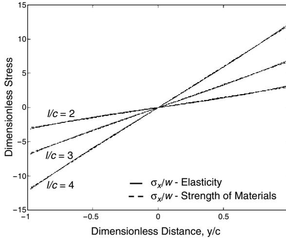
FIGURE 8-4 Comparison of bending stress in beam Example 8-3.
