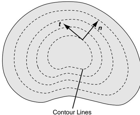
**FIGURE 9-6** Contour lines for the torsion-membrane analogy.
