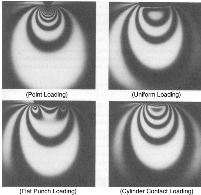
**FIGURE 8-28** Isochromatic photoelastic fringe patterns for several contact loadings on a half plane. (Taken from *Contact Mechanics* by KL Johnson, reprinted with the permission of Cambridge University Press.)
