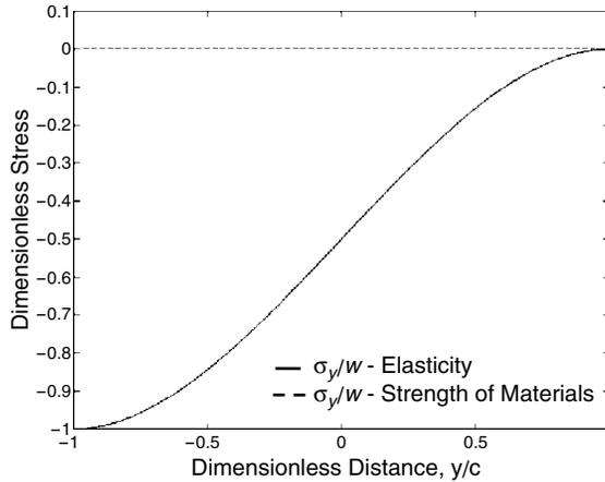
FIGURE 8-5 Comparison of  $\sigma_y$  stress in beam Example 8-3.
