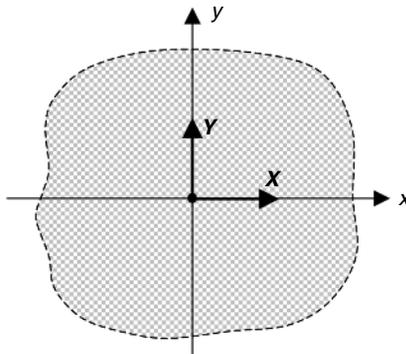
FIGURE 11-7 Concentrated force system in an infinite plane.
