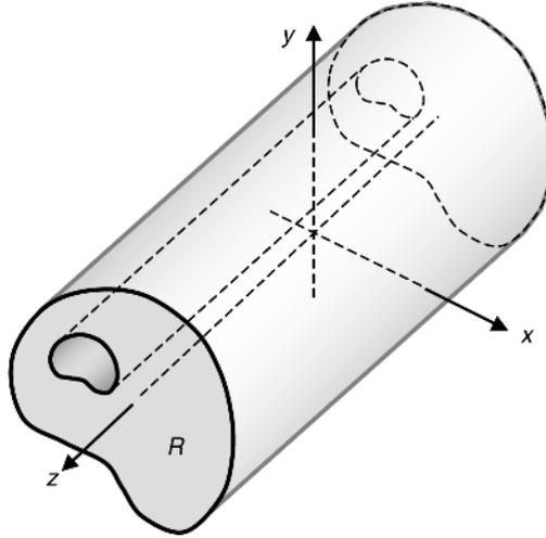
**FIGURE 7-1** Long cylindrical body representing plane strain conditions.
