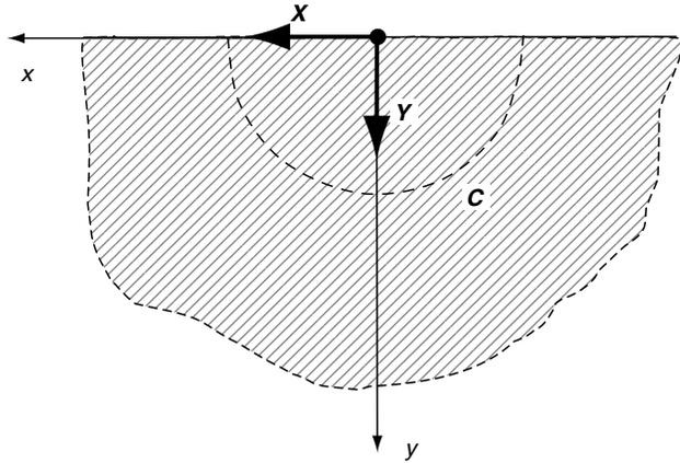
FIGURE 10-12 Concentrated force system on a half space.
