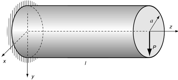
**FIGURE 9-20** Flexure of a beam of circular section.
