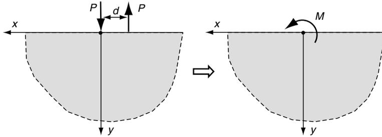
FIGURE 8-23 Half space with concentrated surface moment loading.
