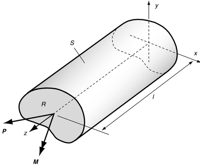
FIGURE 9-1 Prismatic bar subjected to end loadings.
