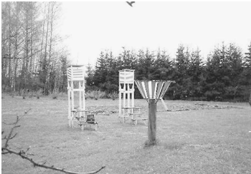
FIGURE 19.4 A synoptic weather station with a hut around temperature measurements and rain gauge.
