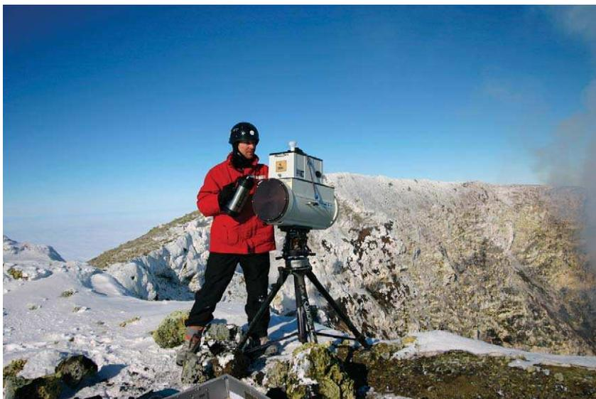
**Fig. 2.** MIDAC brand FTIR spectrometer (optically connected to a Newtonian telescope) being set up at the summit crater rim of Mt. Erebus, Antarctica. The detector dewar is being filled with liquid nitrogen. The volcano's active lava lake was used as an infrared source. The edge of the gas and aerosol plume emitted from the lake is visible at the right-hand edge of the photograph (photo C. Oppenheimer).
