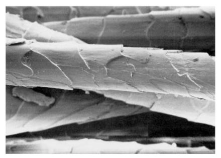
6.4 The scales on a wool fibre  $\times$ 1300.
