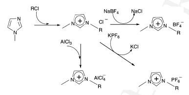
Fig. 1. Typical preparation routes for ionic liquids.
