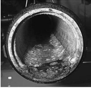
**Figure 13.8** Galvanized pipe damaged by corrosion. (Photo courtesy of Orr Protection Systems, Inc.)
