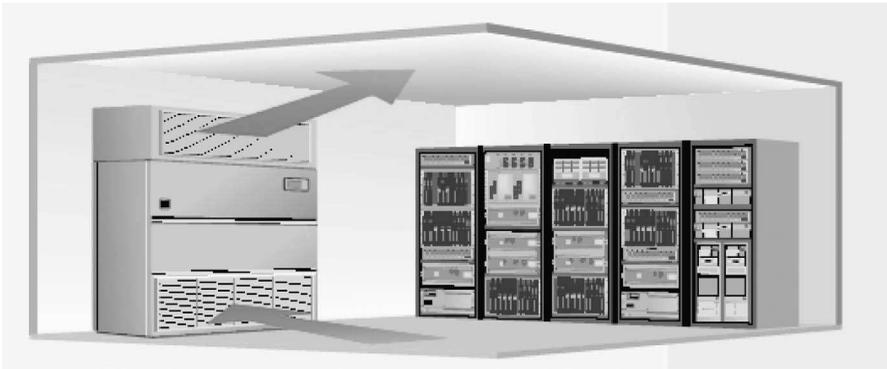
**Figure 11.27** Upflow CRAC unit airflow path. (Image courtesy of Liebert.)
