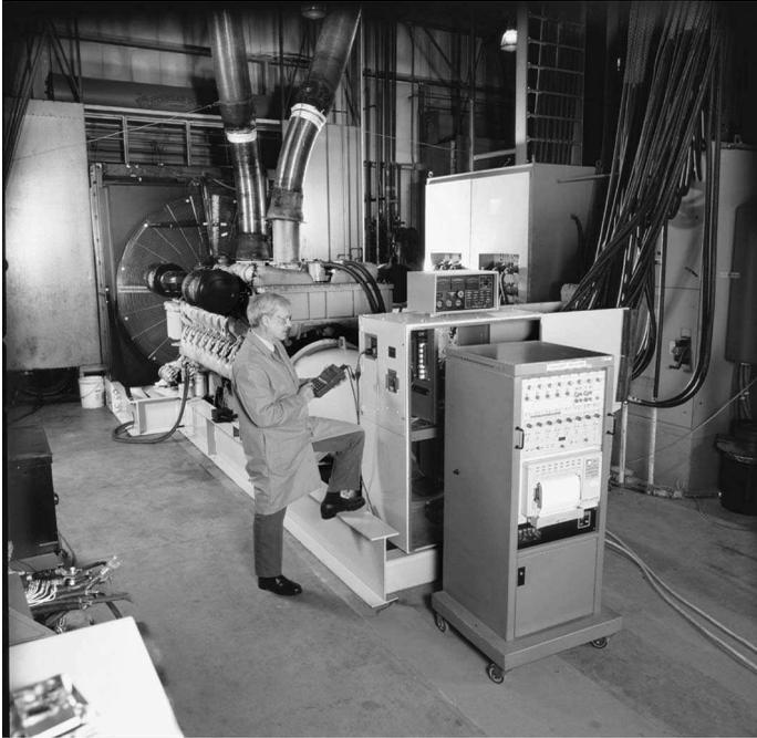
**Figure 5.2** Load bank testing. (Courtesy of ADDA)
