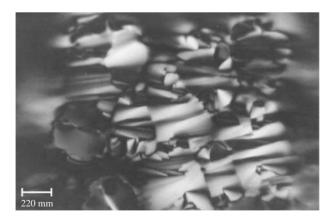
FIG. 1.35. Typical fan-like texture of a hexagonal phase for a 100  $\mu$ m thick sample of a potassium laurate/decanol/water mixture, in a polarizing light microscope, between crossed polarizers.
