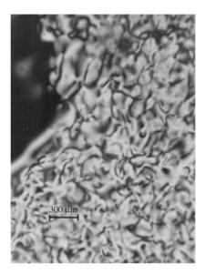
FIG. 1.25. Typical texture of coexisting nematic and micellar isotropic phases (for a 200  $\mu$ m thick sample of a potassium laurate/1-decanol/water mixture) in a polarizing light microscope, between crossed polarizers. The isotropic phase domain is located at the upper left side of the figure.
