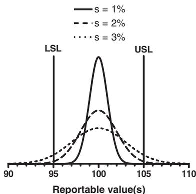
**Figure 10-6** Simulation of (single) reportable values for  $s = 1, 2$  and  $3\%$ .
