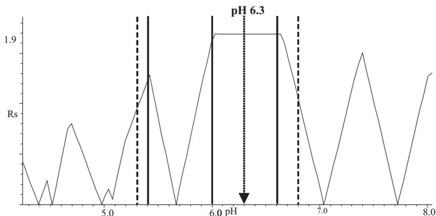
**Figure 2.7-9:** Final resolution map of a one-dimensional optimisation of mobile phase pH; solid lines represent the pHs for the experiments done (5.4, 6.0, 6.6); the dashed lines represent the range in which predictions are allowed. The arrow indicates the pH optimum.
