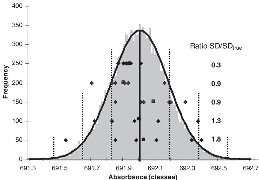
**Figure 2.1-2:** Histogram of 15 000 data with the theoretical Gauss curve. The intervals of 1, 2, and 3 (overall, true) standard deviations around the overall mean are indicated by dotted lines. The horizontally arranged diamonds represent random series of six subsequent data each, their means are given as squares. For each series, the standard deviation is calculated, as a ratio to the overall (true) SD.
