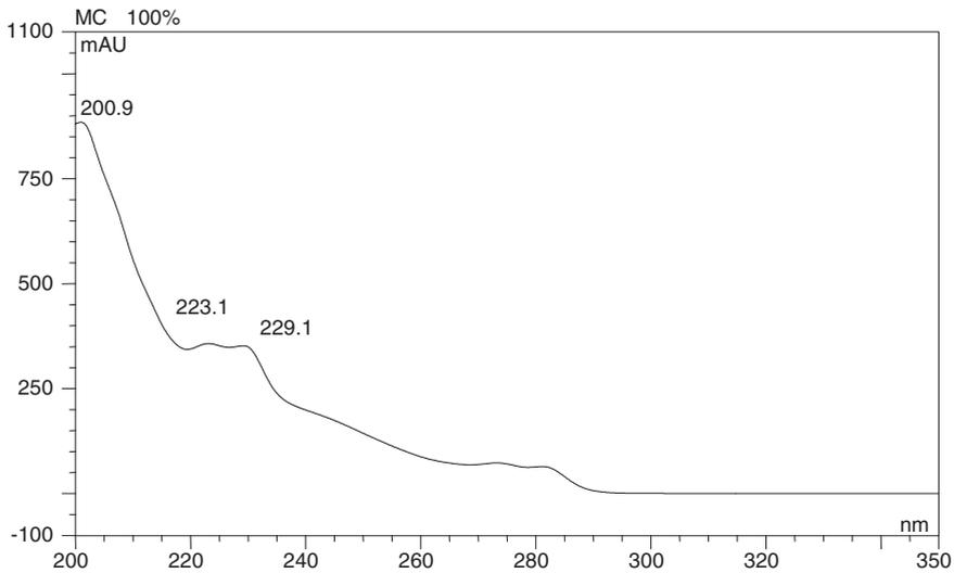
Figure 2.7-17: Section of the uv/vis-spectrum of the main component MC. Absorption [m AU] vs. wavelength [nm]
