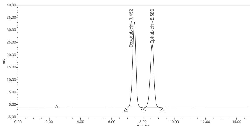
Figure 2.8-1: System Suitability Test – resolution between doxorubicin and epirubicin.
