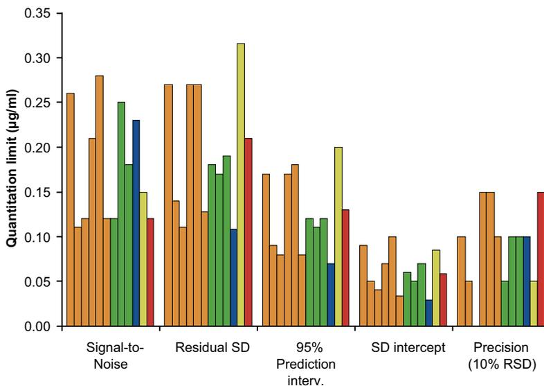
**Figure 2.6-6:** Intermediate QL study using five LC systems with one to six repetitions per system over nine months. The columns of the same colour illustrate the same LC-system used, and their sequence the repetition, i.e., the first orange column for each calculation mode corresponds to the first QL-study on LC-system 1, the second column to the second series on system 1, etc.
