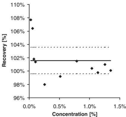
**Figure 3-7** Recovery of DP1 from spiked placebo and MC. The mean recovery and its 95% confidence limits are indicated by solid and dotted line(s), respectively.
