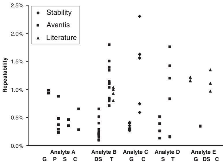
Figure 2.1-10: Repeatabilities for LC assay sorted according to the analyte. The letters correspond to the type of drug product (G = gel, P = powder, S = solution, C = cream, DS = drug substance, T = tablet). The origin of the data is indicated by the symbols and explained in the text.
