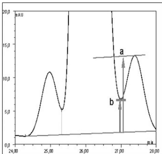
**Figure 2.2-2:** Peak separation indices for minor peaks [73]:
