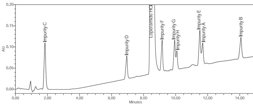
**Figure 2.8-4:** Chromatogram of loperamide hydrochloride for system suitability CRS.
