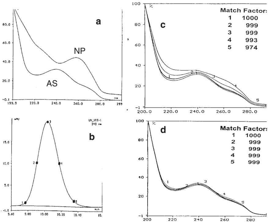
**Figure 2.2-7:** Investigation of chromatographic peak purity by means of diode array detection
