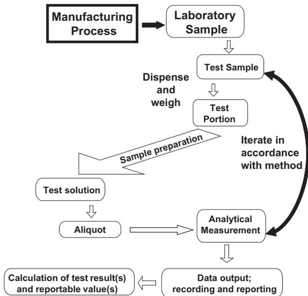
Figure 10-4: Analytical process flow.
