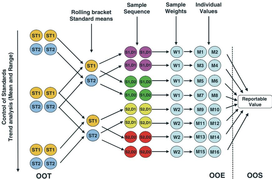
Figure 10-11 HPLC example; calculation method.
