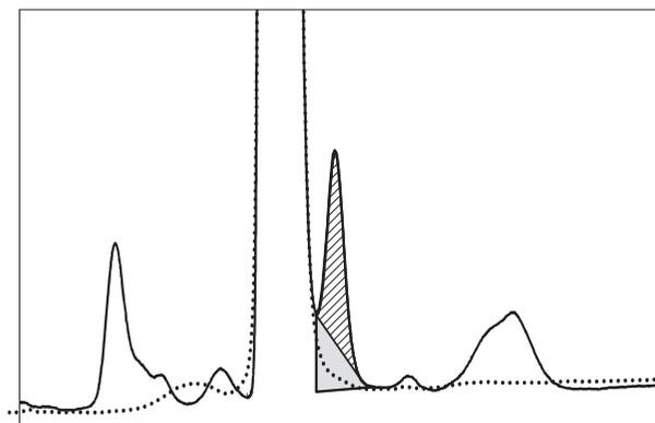
**Figure 2.3-2:** The influence of the mode of peak integration on the result. The solid and dotted lines represent the chromatogram of a peptide sample and an overlay of a heart-cut, re-chromatographed fraction from the main peak (in order to obtain an impurity-free sample), respectively. In the case of an integration as rider (hatched area), the impurity peak is only 62 % of the area obtained by a drop integration (grey area).
