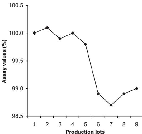
**Figure 9-6** Example of a shift in production process quality or change in assay.
