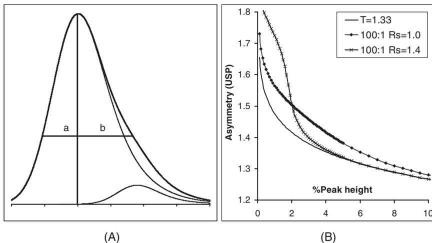
**Figure 2.2-5:** Peak asymmetry ( $(a+b)/2a$ , according to USP, A) and its dependence from the height (B) for various degrees of co-elution in the case of peak tailing (tailing factor 1.33) and a height ratio of 100:1. For smaller and larger size differences, the asymmetries at larger and smaller peak heights will be affected, respectively.
