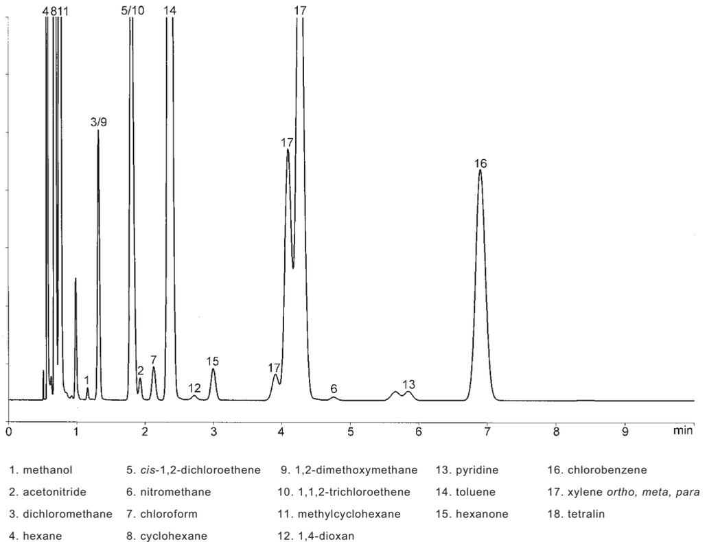
Figure 8-6 Chromatograms of Class 2 residual solvents using system B [45].
