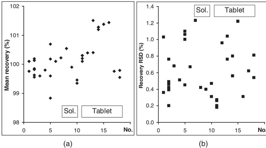
**Figure 2.3-7:** Mean (a) and relative standard deviation (b) of recoveries for LC-assays of 18 drug products. The results are sorted according to the type of drug product, with lyophilisates (No. 1-2), others (No. 3-6), solutions (No. 7-10), and tablets (No. 11-18).
