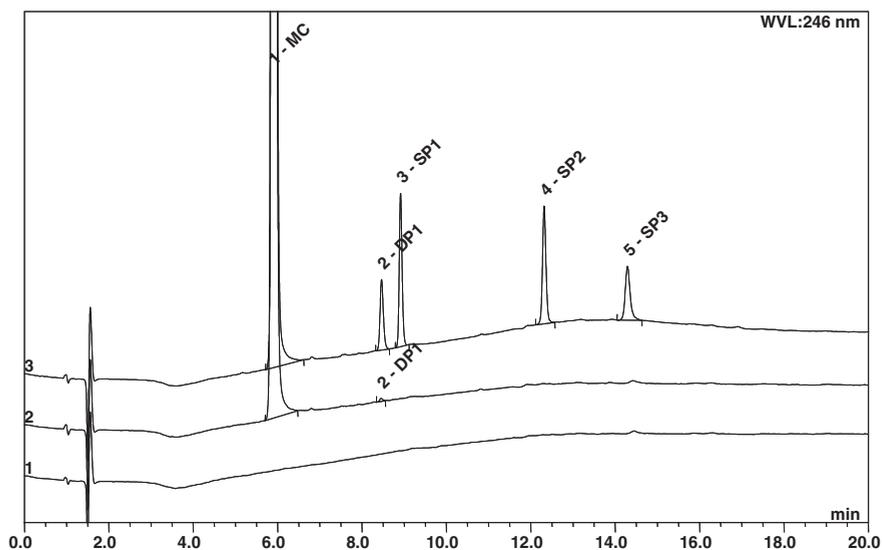
**Figure 3-1** Chromatograms of a solution comprising the main component (MC), process-related impurities (SP1-3) and the degradation product (DP1) at 1% of the working concentration (No. 3), of a degraded MC sample (No. 2), and of a placebo solution (No. 1).
