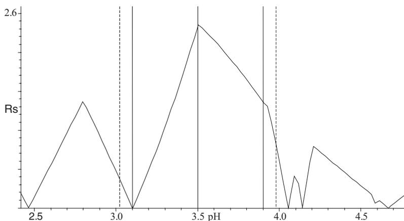
**Figure 2.7-8:** Final resolution map of a one-dimensional optimisation of mobile phase pH. The solid bars represent the pHs for the experiments done (3.1, 3.5, 3.9); the dashed bars represent the range in which predictions are allowed.
