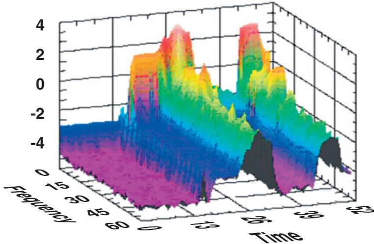
**Figure 11-2** Typical passive acoustic signal obtained during a high shear granulation process and revealing the distinctive features attributable to the dry mixing, wet massing and wet granulation phases of the process.
