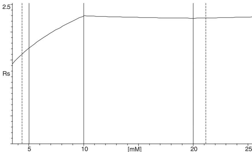
**Figure 2.7-6:** Resolution map of a one-dimensional optimisation of buffer concentration. Solid lines represent the concentrations for the experiments done (5, 10, 20 mM); the dashed lines represent the range in which predictions are allowed.
