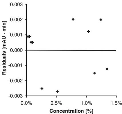
**Figure 3-5** Residual plot for the linear regression analysis of DP1. The scale of the y-axis corresponds to  $\pm 1.3\%$  of the signal at 100% working concentration.
