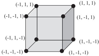
**Figure 2.7-10:** Experimental design for three factors ( $k=3$ ) at two levels ( $n=2$ ) in a transformed coordinate system.
