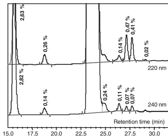
**Figure 2.3-3:** Chromatogram overlay at the nominal wavelength (240nm) and a check-wavelength (220nm). The chromatograms were normalised with respect to the main peak and the impurity peaks are quantified as percentage area.
