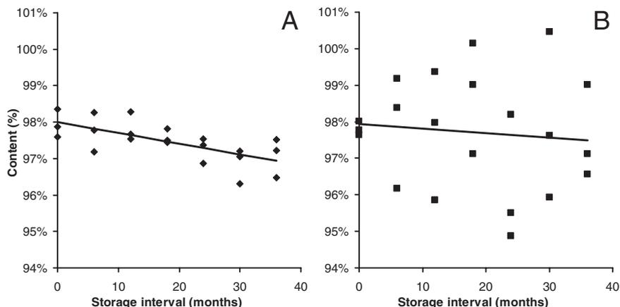
**Figure 1-3** Illustration of the requirements for assay of an active ingredient during a stability study. The three individual results per storage interval were simulated based on a 1% decrease of content within 36 months and a normally distributed error of 0.5% (A) and 2.0% (B) using Eq. (2.1-3). The slope of the regression line in B is not significant.
