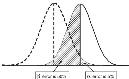
**Figure 2.6-9:** Statistical basis for the detection limit.
