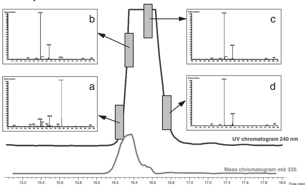
**Figure 2.2-8:** Investigation of chromatographic peak purity by means of LC-MS The upper and lower chromatogram display the UV (at 240 nm) and the extracted ion chromatogram (for  $m/z$  325), respectively. The inserts (a) to (d) are representative mass spectra over the investigated (UV) peak. The amount of co-eluting impurity corresponds to 0.5 %. (Reproduced with permission from [74].)
