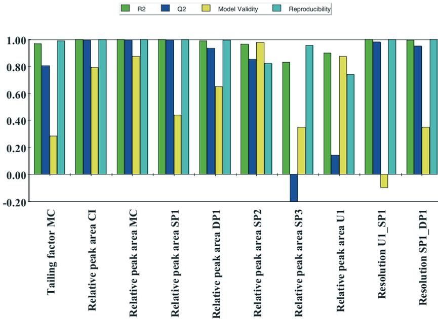
**Figure 2.7-13:** Summary of fit for all responses defined in this robustness study.  $R^2$  is the percentage of the variation of the response explained by the model.  $Q^2$  is the percentage of the variation of the response predicted by the model. The model validity measures the error of fit. Reproducibility is a comparison of the variation of the response under the same conditions with the total variation of the response.
