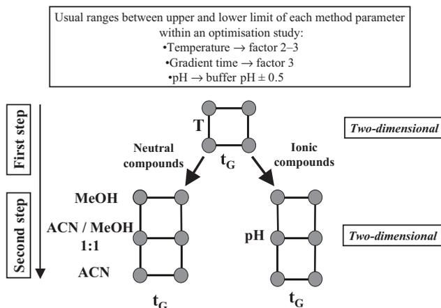
**Figure 2.7-3:** Standardised method development procedure using DryLab (Aventis, Frankfurt; GPD Analytical Sciences); the two-dimensional experiments of the second step can also be carried out one-dimensionally to save three experiments.
