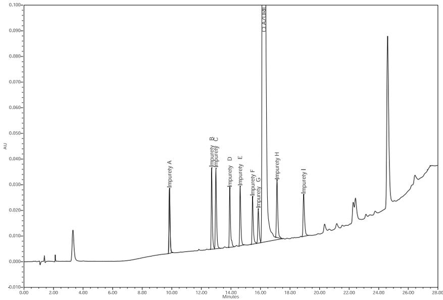
**Figure 2.8-3:** Chromatogram of clazuril for system suitability CRS.
