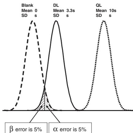
**Figure 2.6-10:** Statistical basis for the ICH detection limit and quantitation limits (DL and QL).
