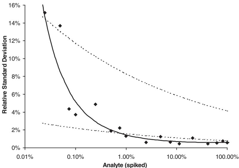
**Figure 2.1-6:** Repeatability investigations for an LC assay over a concentration range from 0.025 to 100% (data from [65]). The solid line illustrates the repeatability trend, obtained by quadratic regression of the logarithm of the standard deviation versus the logarithm of the concentration. The broken lines indicate the limits of the Horwitz range for repeatability [63].
