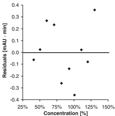
**Figure 3-3** Residual plot for the linear regression analysis of MC. The scale of the y-axis corresponds to  $\pm 1.1\%$  of the signal at 100% working concentration.
