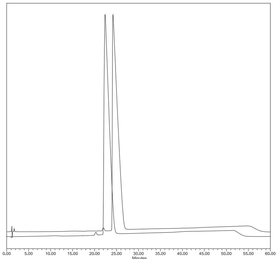
**Figure 2.8-8:** Chromatograms of 0.1% m/v trimethidine for system suitability CRS with pumps of 0.6 ml and 3.4 ml dwell volumes.
