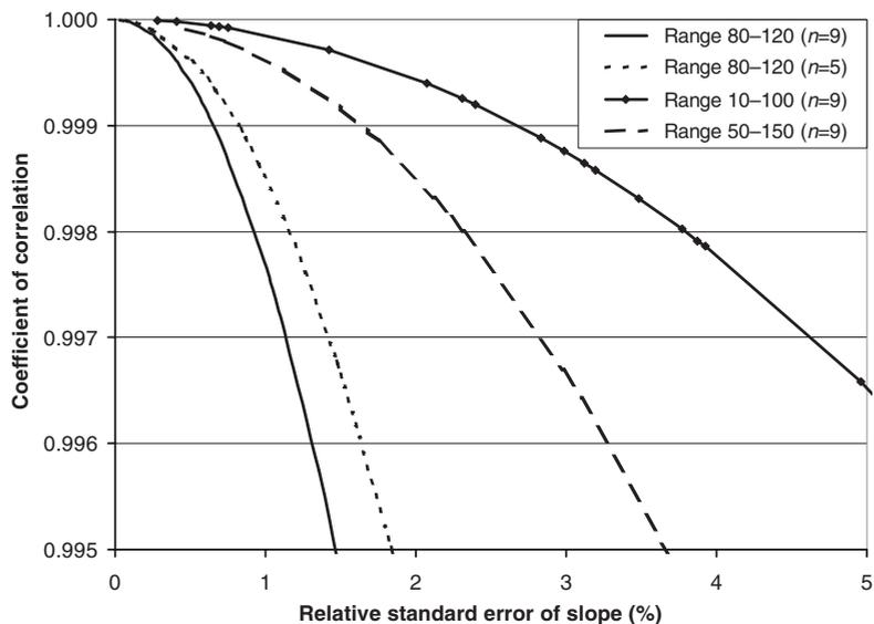
**Figure 2.4-5:** Relationship between the coefficient of correlation and the experimental variability. Data sets were simulated using the response function  $y=x$  and normally distributed errors with a constant standard deviation for each data set. The dependence of  $r$  is shown for several concentration ranges and numbers of data.
