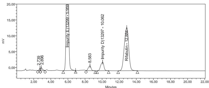
**Figure 2.8-2:** Chromatogram of rifabutin after alkaline hydrolysis. To 10 mg dissolved in 10 ml methanol, was added 1 ml dilute sodium hydroxide solution which was allowed to stand for 4 min. 1 ml of dilute hydrochloric acid was added and diluted to 50 ml with the mobile phase.
