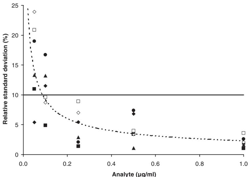
**Figure 2.6-16:** Repeated series of precision for decreasing concentrations. Six determinations were performed for each concentration. The estimation of the average precision function is illustrated by the dotted line, the defined precision acceptance limit by a solid line. Note that, for an acceptable individual precision (in the case of a defined general QL), a larger limit would be required, e.g., at 20% RSD.
