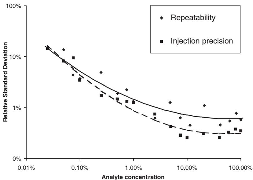
**Figure 2.1-8:** Investigations of injection precision and repeatability for an LC assay over a concentration range from 0.025 to 100% (data from [65]). The solid and broken lines indicate the repeatability and injection precision curves, respectively, and were obtained by quadratic regression of the logarithm of the respective standard deviations versus the logarithm of the concentration.
