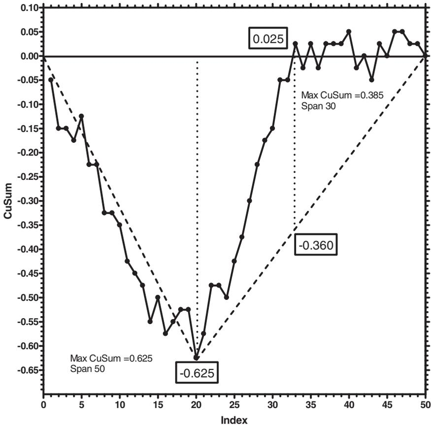
Figure 10-15 Analysis of CuSum turning points for HPLC  $R_s$  data.
