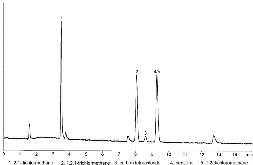
Figure 8-3 Chromatograms of Class 1 residual solvents using system A [45].
