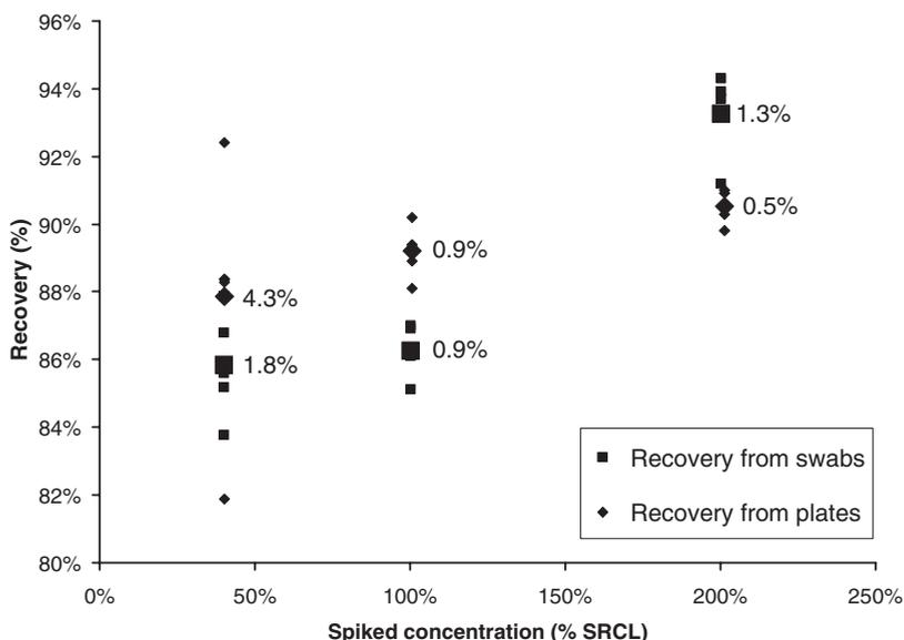
**Figure 2.3-5:** Recovery of meclizine from stainless steel plates and from swabs (data from [13]). Five individual spiking per concentration level were performed (smaller symbols). To the right of each mean (larger symbols), the relative standard deviation is indicated.
