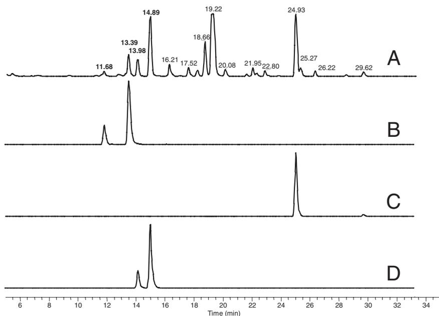
**Figure 2.2-1:** RP chromatography with UV (A) and mass spectrometric detection (B–D). The smaller peaks in traces B–D belong to the D-amino acids. (Reproduced with permission from [70].)
