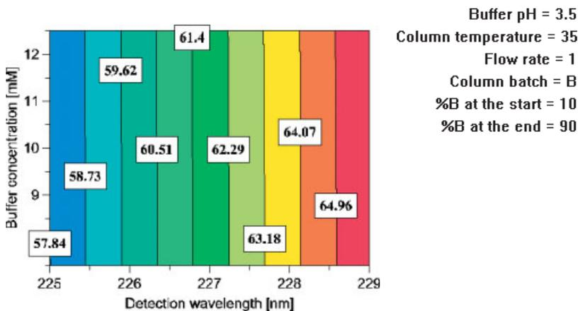
**Figure 2.7-22:** Contour Plot of the relative peak area of MC as a function of the buffer concentration and the detection wavelength; all other factors are kept at the centre levels; columns stationary phase material B selected.
