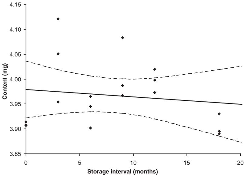
**Figure 2.1-14:** Stability study of a film tablet batch at 25 °C/60% relative humidity over 18 months. Besides the individual content determinations, the unweighted linear regression line with its 95% confidence intervals is shown.
