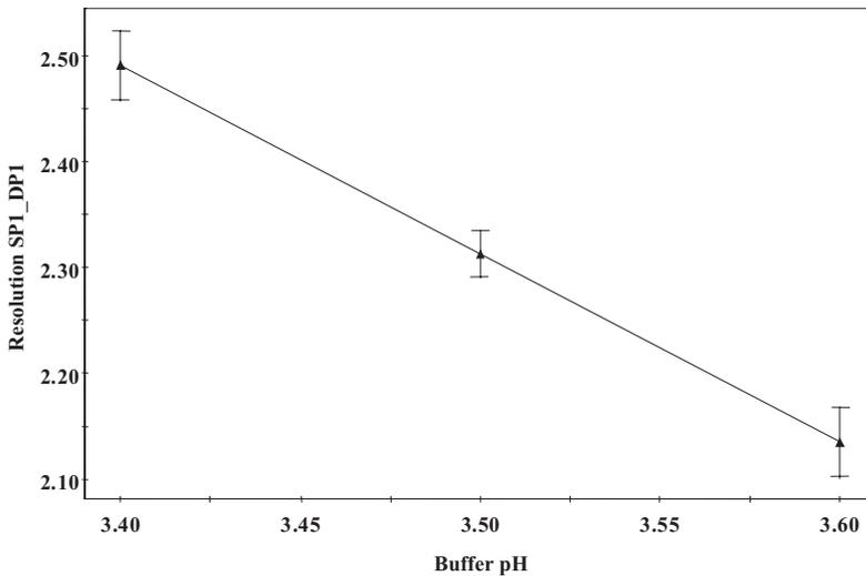
Figure 2.7-21: Main effect plot of the response Resolution SP1\_DP1 as a function of the factor pH.
