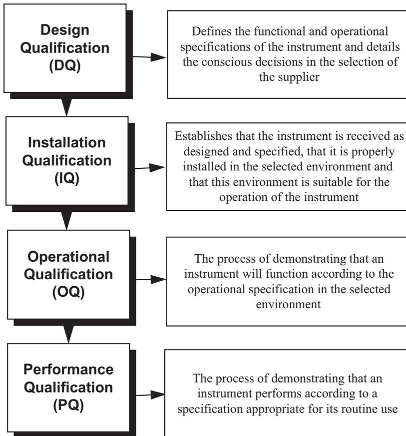
**Figure 4-1** The equipment qualification process.
