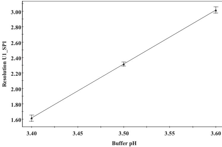
Figure 2.7-20: Main effect plot of the response Resolution U1\_SP1 as a function of the factor pH.
