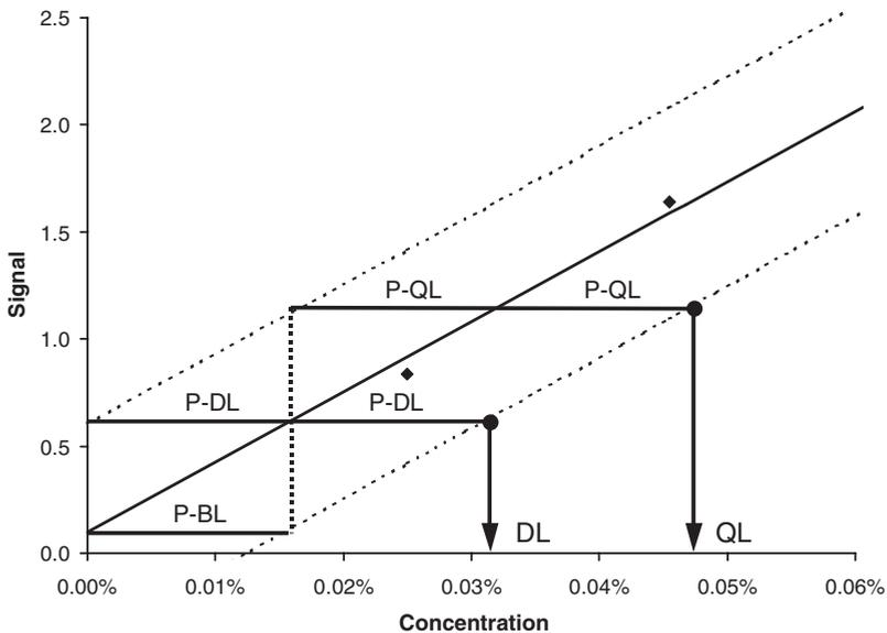
**Figure 2.6-14:** Utilisation of the 95% prediction intervals (dotted lines) of an unweighted linear regression (solid line) to obtain DL and QL (according to [103]). The horizontal lines indicate the 95% width of the probability distributions of the (upper half of the) blank (P-BL), the detection limit (P-DL), and the quantitation limit (P-QL).
