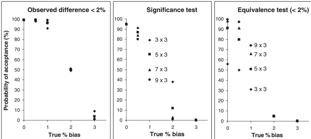
**Figure 7-2** Probability of concluding that a relative bias is acceptable in dependence on the true bias and the number of determinations for the three comparison approaches. Three replicates each are performed on three (diamonds), five (squares), seven (triangles), and nine (circle) days. The simulations are based on a true repeatability and intermediate precision of 0.5 and 1.0%, respectively (data obtained from [3]).
