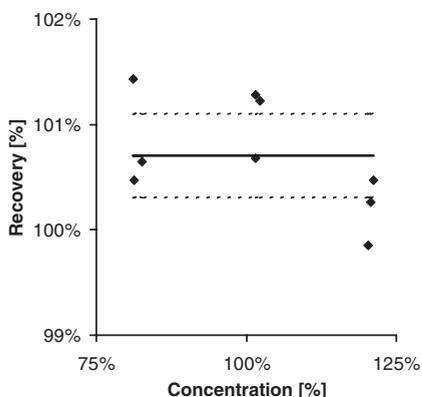
**Figure 3-6** Recovery of MC from spiked placebo. The mean recovery and its 95% confidence limits are indicated by solid and dotted line(s), respectively.
