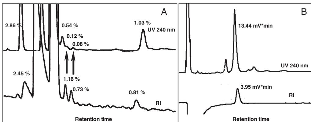
**Figure 2.3-4:** The estimation (A) and determination (B) of the response factor of an impurity by means of UV (upper chromatograms) and refractive index detection (lower chromatograms). The left chromatograms (A) show a whole sample, whereas in the right chromatograms (B) one of the relevant impurity peaks (labelled with arrows) was collected and re-chromatographed under conditions optimised for the RI detection.
