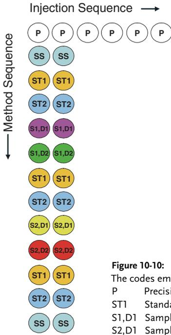
Figure 10-10: HPLC example: injection sequence.
