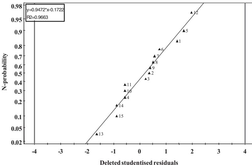
Figure 2.7-14: Normal probability plot for the tailing factor of the main component.
