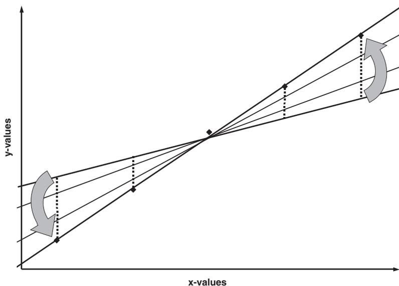
**Figure 2.4-1:** The principle of least-squares regression. The vertical distances between the experimental data and the regression line (i.e., the residuals, dotted lines) are squared and the line is varied until the sum of the squared residuals is at the minimum.
