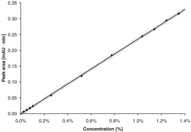
**Figure 3-4** Peak area of DP1 as a function of its concentration. Besides the experimental data points and the unweighted linear regression line, the 95% prediction intervals (dotted line) are indicated.
