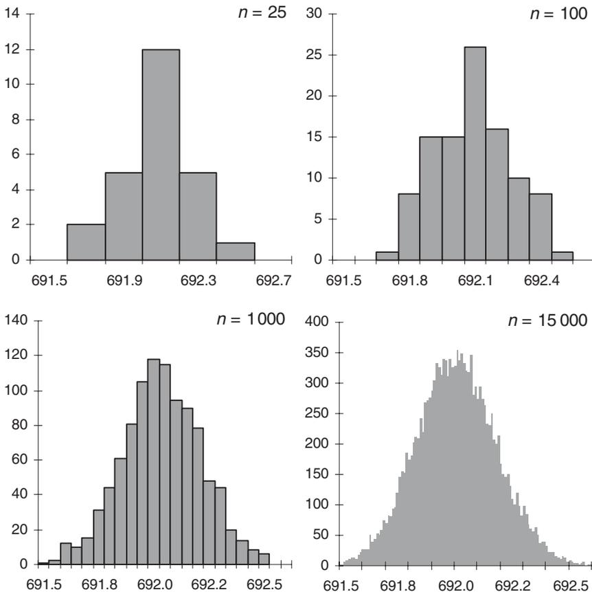
**Figure 2.1-1:** Histograms of 25, 100, 1000 and 15 000 data (for details see text). The y-axes display the frequency of the data within the absorbance intervals (classes) indicated on the x-axes. Apart from  $n=15\,000$  (where the number of classes is too high), each bar representing a data class is shown. The normal distribution of all four data sets was confirmed by  $\chi^2$ -tests.
