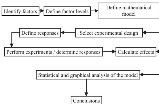
**Figure 2.7-11:** General procedure for statistical design, conductance, analysis and interpretation of experiments.
