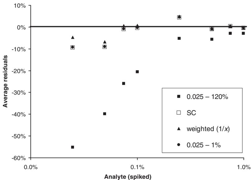
**Figure 2.4-10:** Residual plots for the regressions shown in Figure 2.4-9. The residuals are calculated with respect to the fitted signal (relative residuals), in order to illustrate the deviation for small concentrations, and only the average per concentration is reported. The concentrations on the x-axis are given in a logarithmic scale to facilitate the inspection of a larger concentration range.
