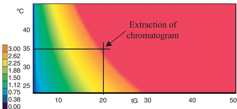
**Figure 2.7-4:** Resolution map of a two-dimensional optimisation of gradient time and temperature. The colour as the third dimension of the map represents the resolution for the critical peak pair, as shown in the legend left. The extraction of the optimised chromatogram is indicated at the intersection of the lines for gradient time and temperature.
