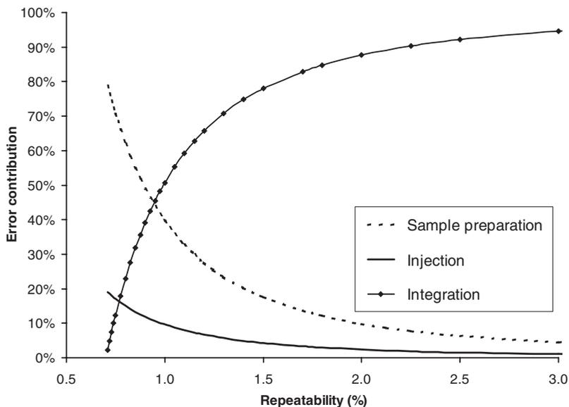
**Figure 2.1-7:** Error contributions to an increasing repeatability (data from [65]). The sample preparation error and injection error were estimated to 0.63% RSD and 0.31% RSD, respectively, calculated from seven data sets of five – seven samples each, between 10% and 120% of the nominal test concentration.
