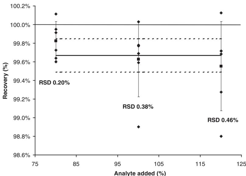
**Figure 2.3-1:** Recovery investigations for a lyophilised drug product. The diamonds represent the six individual spiking at 80, 100, and 120 % each (of the nominal concentration level). The relative standard deviations of the recoveries for each level are given. The mean and the 95 % confidence intervals for each level are shown as squares and bars, respectively. The overall mean, with 95 % confidence interval, is indicated by horizontal, solid and dotted lines, respectively.
