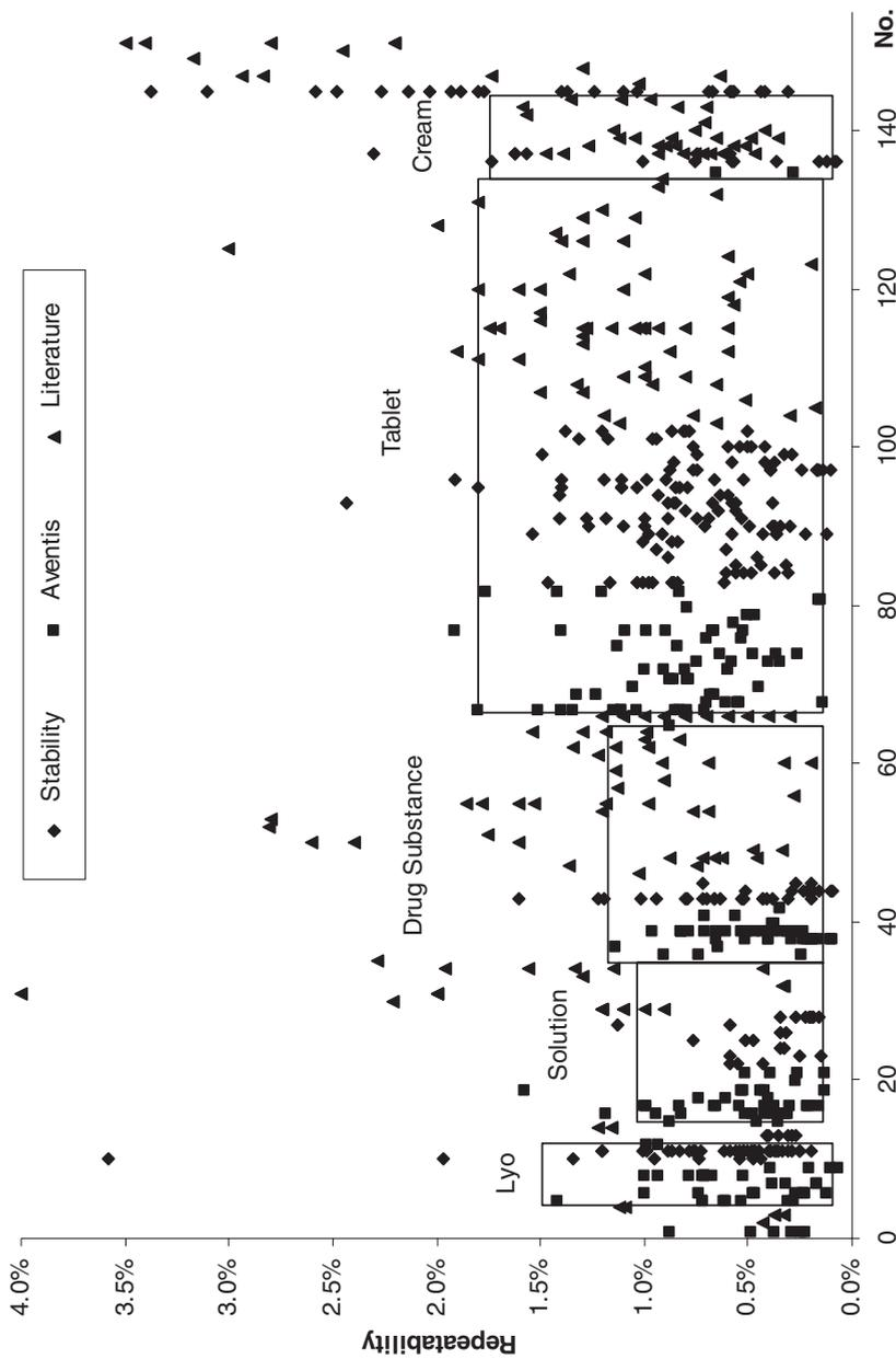
**Figure 2.1-11:** Repeatabilities for LC assay sorted according to the type of sample (drug product). The sequence on the x-axis corresponds to different analytes or sources. The origin of the data is indicated by the symbols and explained in the text. For sample types with sufficient results available (Aventis and Stability origin), the 95% distribution ranges are shown by rectangles.
