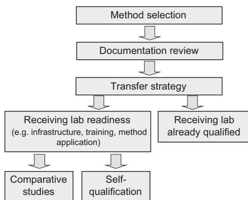
**Figure 7-1** A five-step process for analytical transfer.
