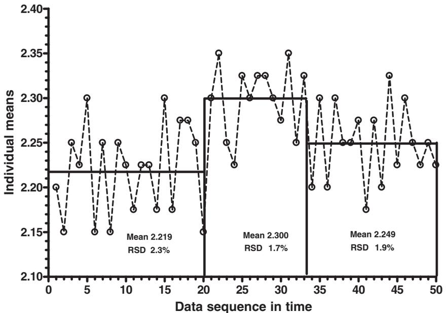
**Figure 10-16** Manhattan plot and regional means and RSDs for HPLC  $R_s$  data.
