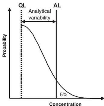
**Figure 2.6-7:** The acceptance limits of the specification (AL) must include both analytical and manufacturing variability. The (true) quantitation limit (QL) represents the maximum manufacturing variability with respect to impurity content. The analytical variability can be described by a 95 % prediction interval (for details, see Section 6.3).
