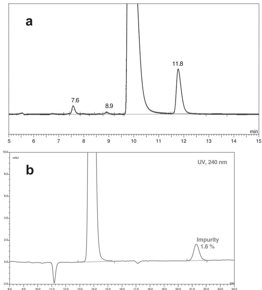
**Figure 2.2-6:** Investigation of chromatographic peak purity by means of re-chromatography. (a) Chromatogram of the method to be validated (acetonitrile/water/0.1% trifluoroacetic acid, RP C8 column). The main peak was heart-cut from 9.6 to 11.0 minutes. (b) Re-chromatography of the main peak fraction using another method (acetonitrile / 0.2M sodium phosphate buffer pH 4.0, RP C8-column). (Reproduced with permission from [74].)
