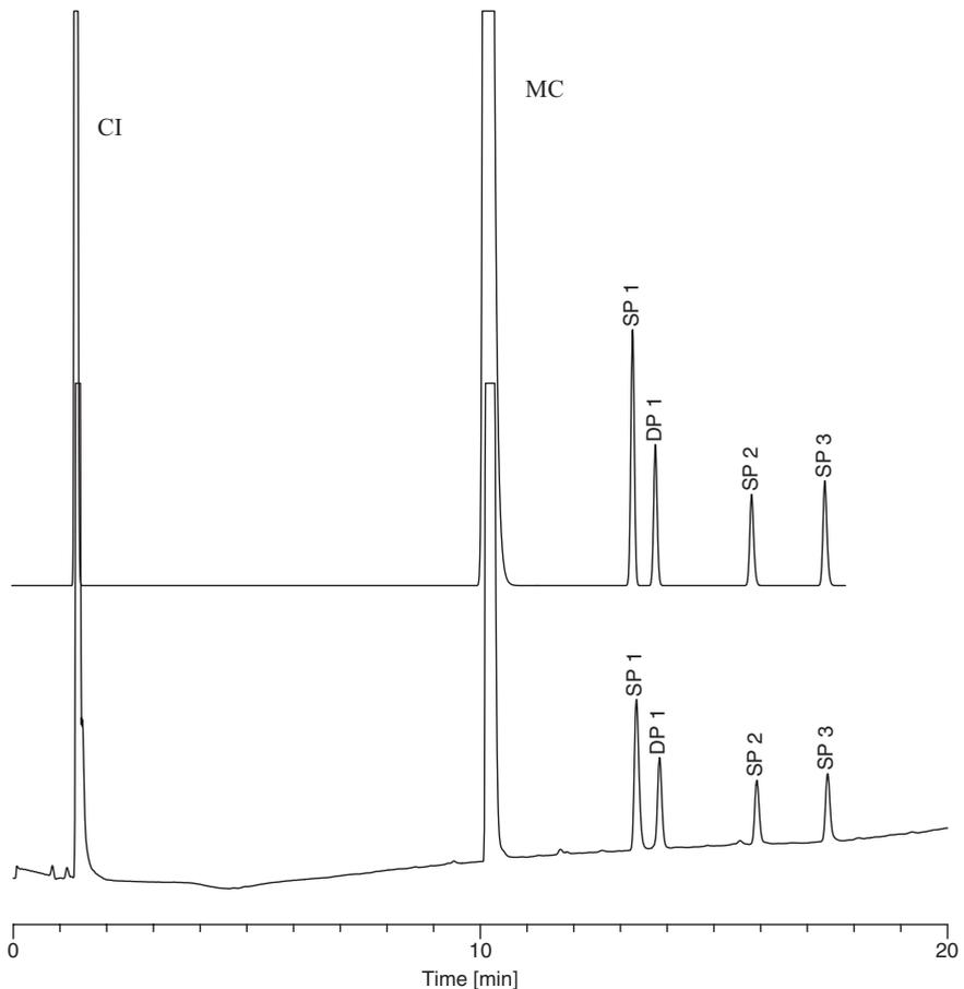
**Figure 2.7-5:** DryLab prediction obtained for 20 minutes gradient time and 35 °C column temperature (upper chromatogram) in comparison with the experimental run at these conditions (lower chromatogram)
