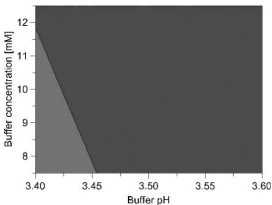
**Figure 2.7-24:** SweetSpot Plot –  $T_{MC}$ ,  $R_{U1\_SP1}$ ,  $R_{SP1\_DP1}$  vs. buffer pH and buffer concentration; SweetSpot:  $0.8 \leq T_{MC} \leq 1.7$ ,  $R_{U1\_SP1} \geq 1.8$ ,  $R_{SP1\_DP1} \geq 1.8$ ; CENTRE level for other factors; batch A of stationary phase material. Dark grey indicates that all criteria are met. Light grey represents the area where only two criteria are fulfilled ( $1.4 < R_{U1\_SP1} < 1.8$ ).
