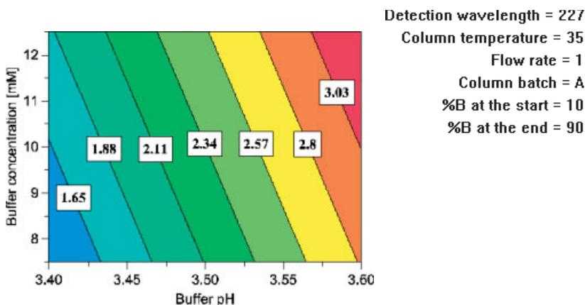
**Figure 2.7-23:** Contour Plot of the resolution between U1 and SP1 as a function of the buffer concentration and the buffer pH; all other factors are kept at the centre levels; columns stationary phase material A selected.
