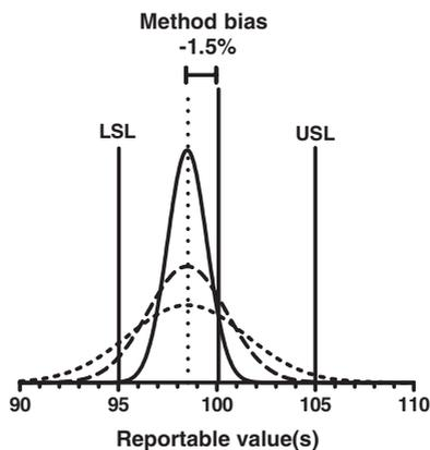
Figure 10-7 Process capability for a process mean of 98.5% (1.5% bias).
