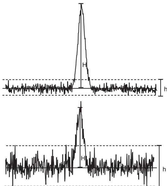
**Figure 2.6-8:** Signal-to-noise examples of 10:1 (top) and 3:1 (bottom), using the method of the EP [15].
