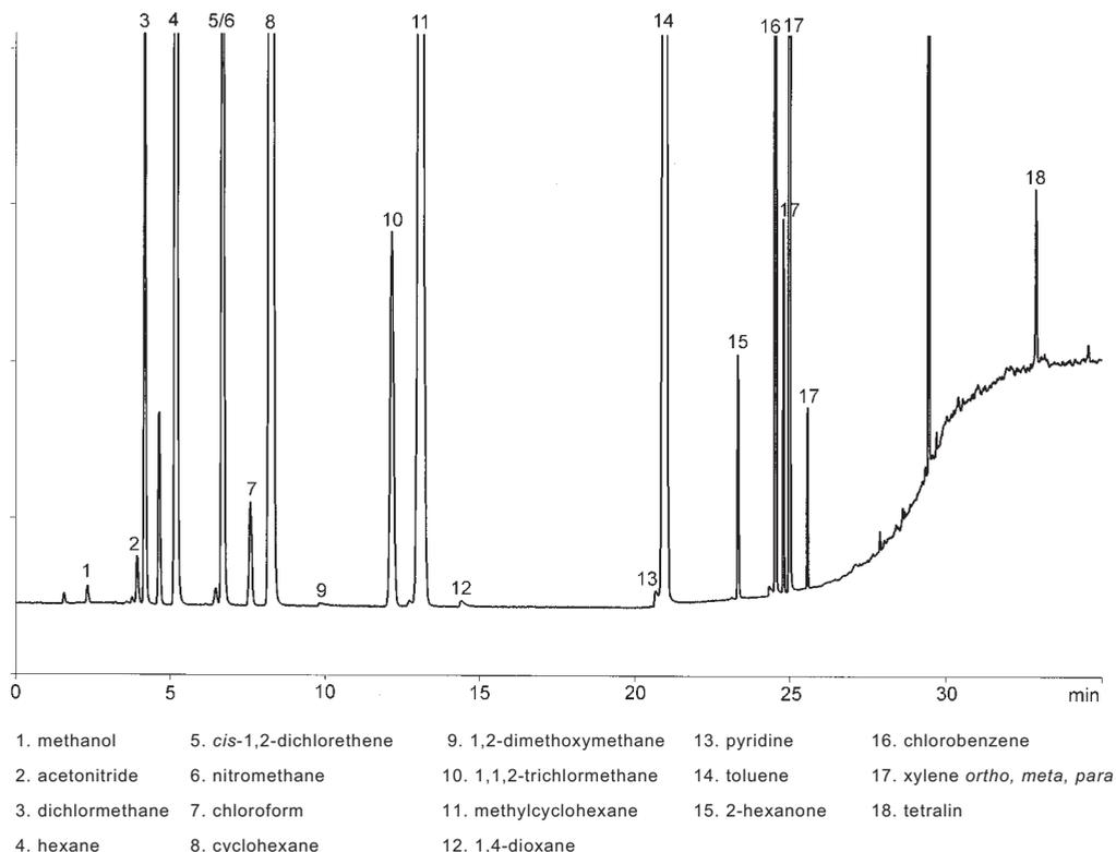
**Figure 8-4** Chromatograms of Class 2 residual solvents using system A [45].
