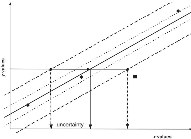
**Figure 2.4-2:** Linear regression line (solid) with the limits of the confidence (dotted line) and prediction intervals (broken line). The resultant uncertainty  $\Delta x$  and a possible outlier (square) are indicated. For details, see text.
