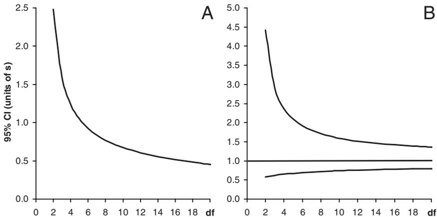
**Figure 2.1-4:** 95% confidence intervals of the mean (A) and of the standard deviation (B) as a function of the degrees of freedom (df) on which the calculation is based. The confidence intervals (CI) are displayed in units of the standard deviation. For one data set (one run or series) the degree of freedom is  $n-1$ , for several independent data sets  $k$ , the degree of freedom corresponds to  $k*(n-1)$ .
