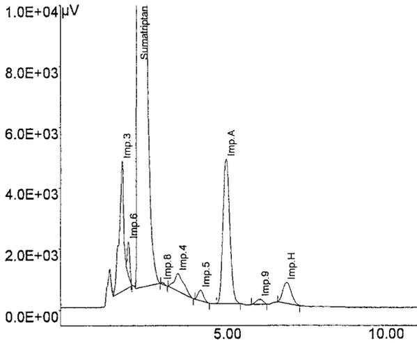
Figure 8-1 Chromatogram of sumatriptan for system suitability CRS to identify impurities A and H [37].
