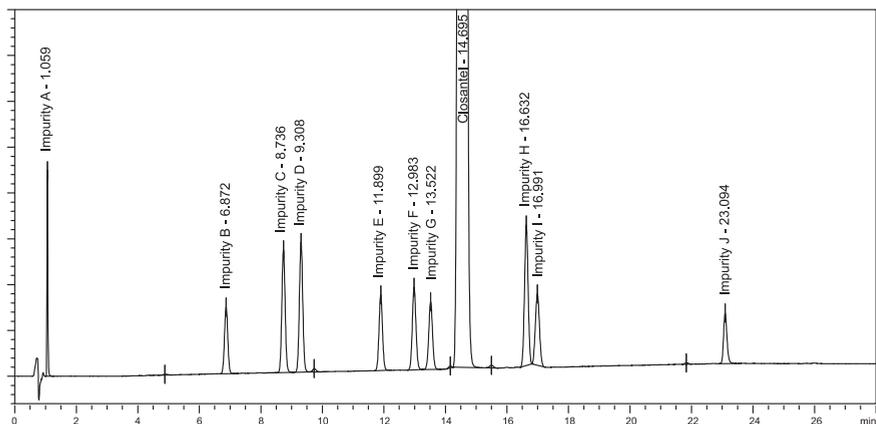
**Figure 2.8-5:** Chromatogram of closantel sodium dihydrate for system suitability CRS.
