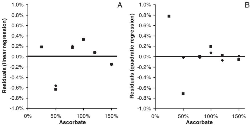
**Figure 2.4-6:** Residual plot for unweighted regression of an LC assay of ascorbate. A linear (A) and a quadratic (B) regression was performed in a concentration range of 25–150% (squares) and of 50–150% (diamonds). In order to facilitate the evaluation, the residuals are presented as percentages with respect to the fitted peak area.
