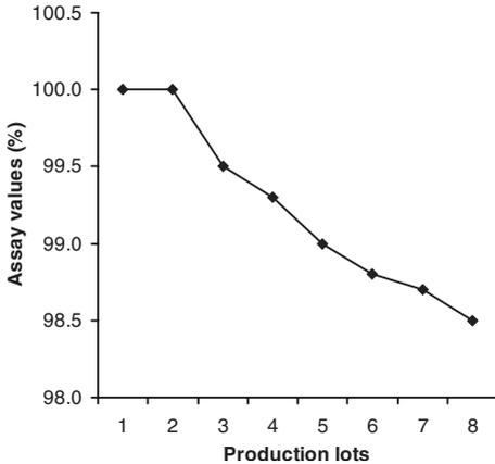
**Figure 9-5** Example of production process out of control.
