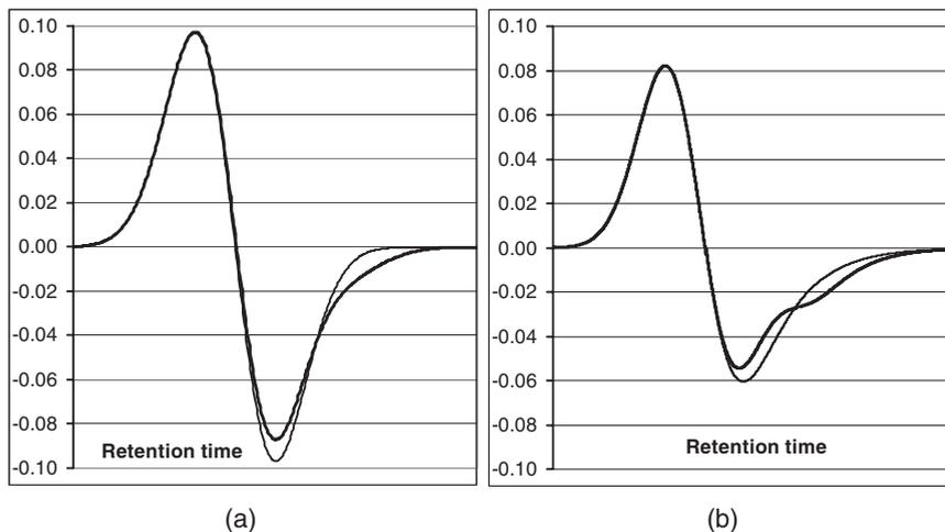
**Figure 2.2-4:** First derivative chromatograms of a symmetric (Gaussian, a) and an asymmetric peak (tailing factor = 1.33, b). The y-axes correspond to the first derivation of the signal. The thinner lines represent the derivation of the major peak alone, the thick lines those of the co-eluted peaks. The peak ratio of a major to minor peak is 10:1, the resolution factor is 0.5, and the minor peak is eluting after the main peak.
