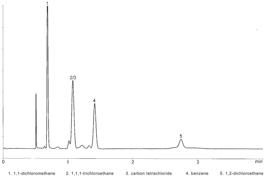
Figure 8-5 Chromatograms of Class 1 residual solvents using system B [45].
