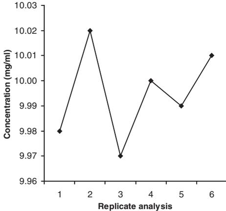
**Figure 9-3** Utilisation of a 10 mg/ml standard preparation as control sample.
