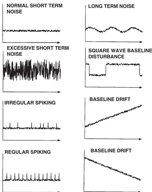
Figure 2.6-2: Noise and drift types (adapted from Table 6.1 [113]).
