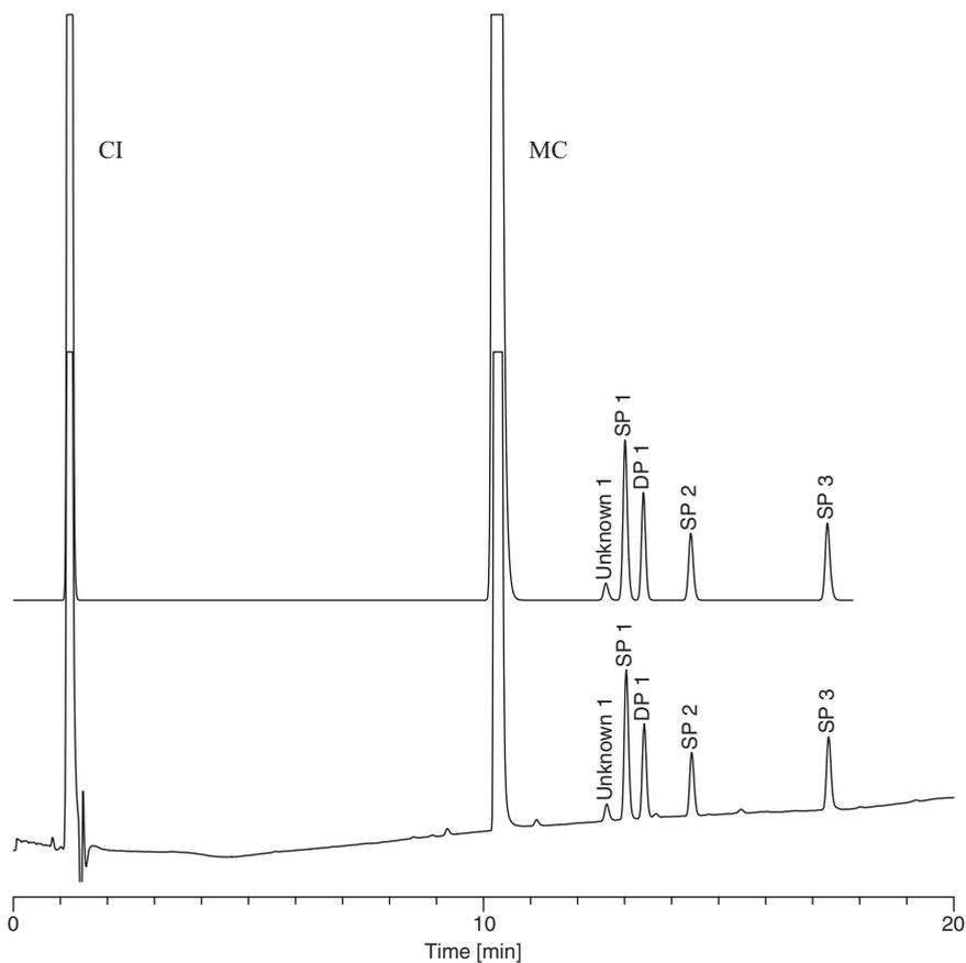
**Figure 2.7-7:** DryLab prediction obtained for 10 mM buffer concentration (upper chromatogram) in comparison with the experimental run under this condition (lower chromatogram).
