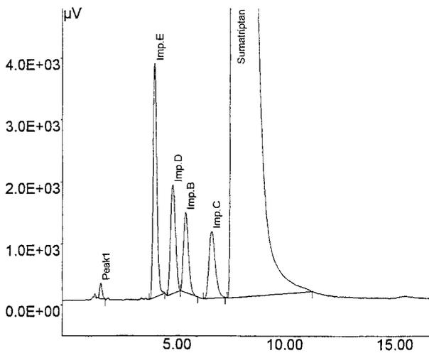
Figure 8-2 Chromatogram of sumatriptan impurity mixture CRS to identify impurities A, B, C, D and E [37].
