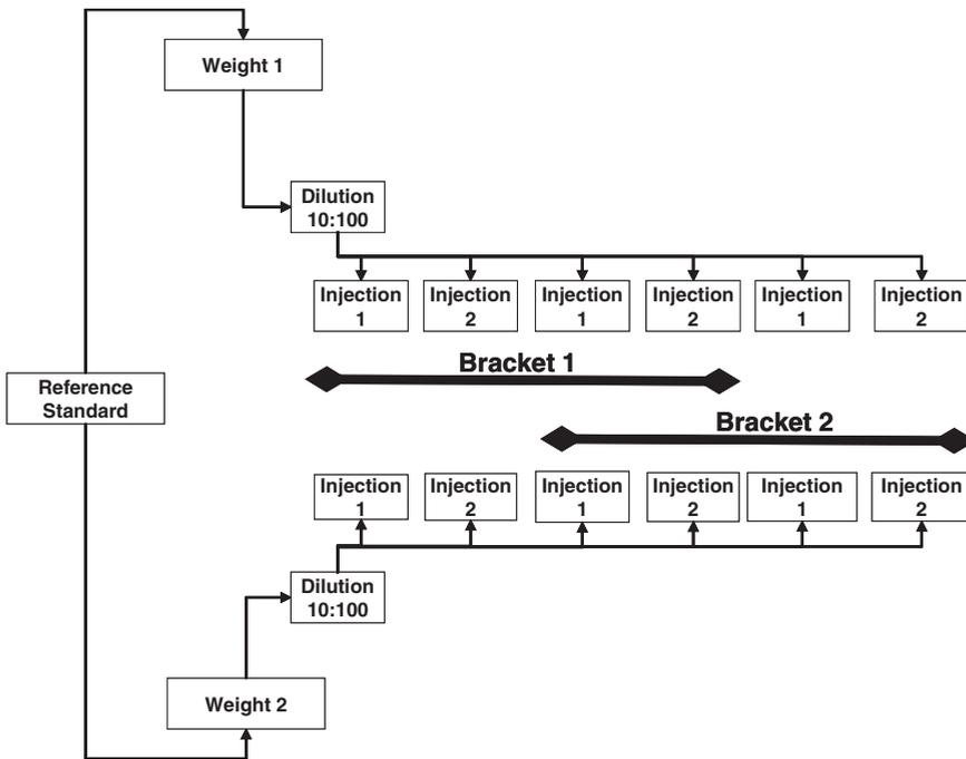
Figure 10-9 HPLC example: standard bracketing scheme.
