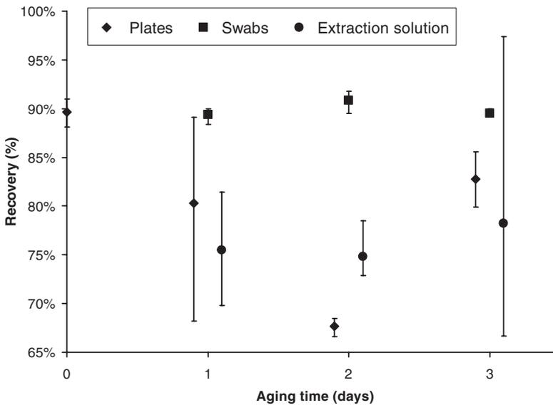
**Figure 2.3-6:** Influence of aging on the recovery of meclizine (data from [13]). The investigations were performed at 200% SCRL with three spikings per storage interval. The means are symbolised and the bars indicate the minimum and maximum recovery of each series. Aging of the samples on the swabs did not affect the result. The overall average and the relative standard deviation for these 12 samples were 89.9% and 1.15%, respectively.
