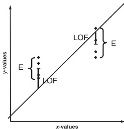
**Figure 2.4-7:** Illustration of the ANOVA lack-of-fit test. The measurement variability  $E$  ('pure error') from replicate determinations is obtained for all concentration levels and compared with the deviation of the means from the regression model LOF (lack of fit error).
