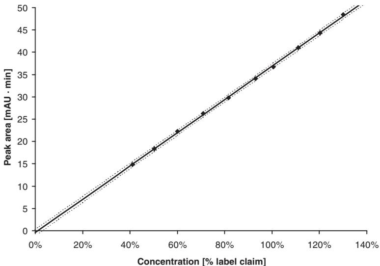
**Figure 3-2** Peak area of MC as a function of its concentration. Besides the experimental data points and the unweighted linear regression line, the 95% prediction intervals (dotted line) are indicated.
