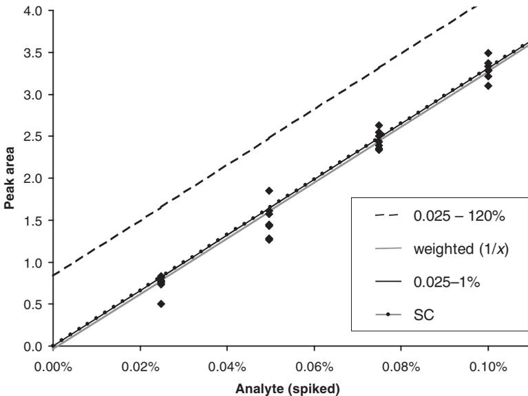
**Figure 2.4-9:** Linearity data (diamonds) and linear regression lines from 0.025 to 120% (data from [65]). Only the lower concentration range is shown. The regression lines for unweighted and weighted (weighting factor  $1/x$ ) regression are shown (broken and shaded line, respectively). Additionally, the line corresponding to the single-point calibration (SC) using the data at 100%, and the line for the regression from 0.025 to 1% (pearl and solid line, respectively) are shown.
