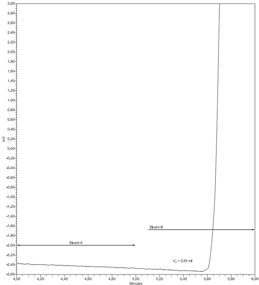
**Figure 2.8-7:** Determination of the dwell volume. Mobile phase A (water) for 5 minutes then mobile phase B (0.5% v/v acetone in water) between 5 and 10 minutes. Flow rate 1.0 ml/min, wavelength of detection 254 nm.
