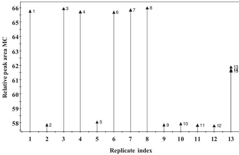
**Figure 2.7-12:** Replicates plot for the relative peak area of the main component MC (relative peak area MC as a function of the experiment number labels). The different levels indicate the absorptions at 225 nm, 229 nm and at the nominal level of 227 nm.
