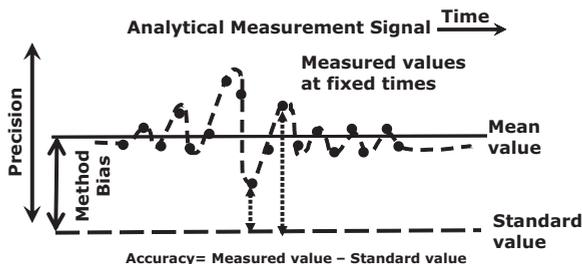
**Figure 10-2** Basic definitions and concepts for analytical measurements.
