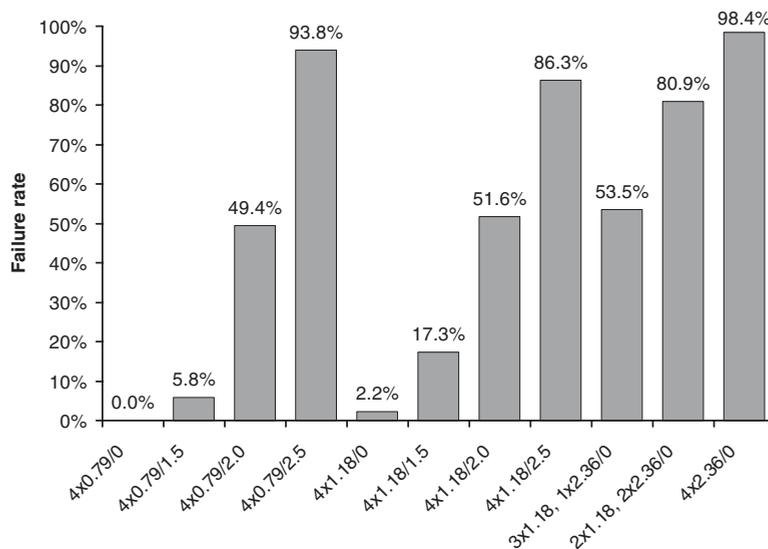
**Figure 7-3** Failure rate for 166 665 simulated collaborative studies of a drug product assay with the acceptance criteria given in Table 7-1. The true relative standard deviation in the four series with six determinations each is indicated first, followed by the true percentage difference between the laboratory means (bias).
