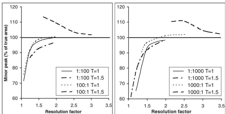
**Figure 2.2-3:** Resolution and (drop) integration accuracy with respect to the minor peak in dependence on peak size, elution order, and tailing (data from [75]). The numbers in the legend represent the ratio of the peak (area), their sequence corresponds to the elution order, and  $T$  indicates the tailing factor. For example, the solid line in the left diagram describes the accuracy of the integrated area of a 1% impurity peak, eluting before the main peak with tailing factors of 1.
