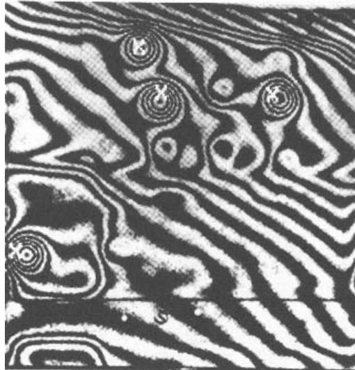
**Figure 11.2** Result of analysing a holographic interferogram by the method shown in Figure 11.1 (From Robinson, D. W. (1983) Automatic fringe analysis with a computer image processing system, *Applied Optics*, **22**, 2169–76. Reproduced by permission of the Optical Society of America and by Courtesy of D. W. Robinson)
