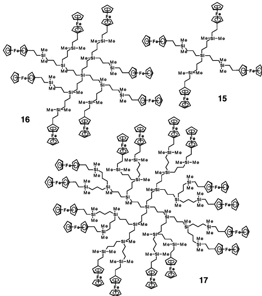
Scheme 6. Organometallic dendrimers in which the peripheral ferrocenyl groups are attached to the silicon-based framework through a two methylene spacer.
