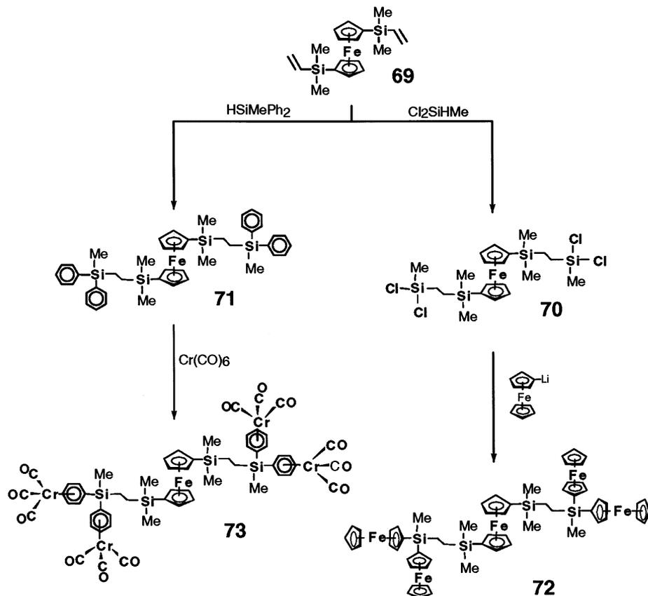
Scheme 26. Ferrocene as two-directional core for the synthesis of homo and heterometallic molecules.
