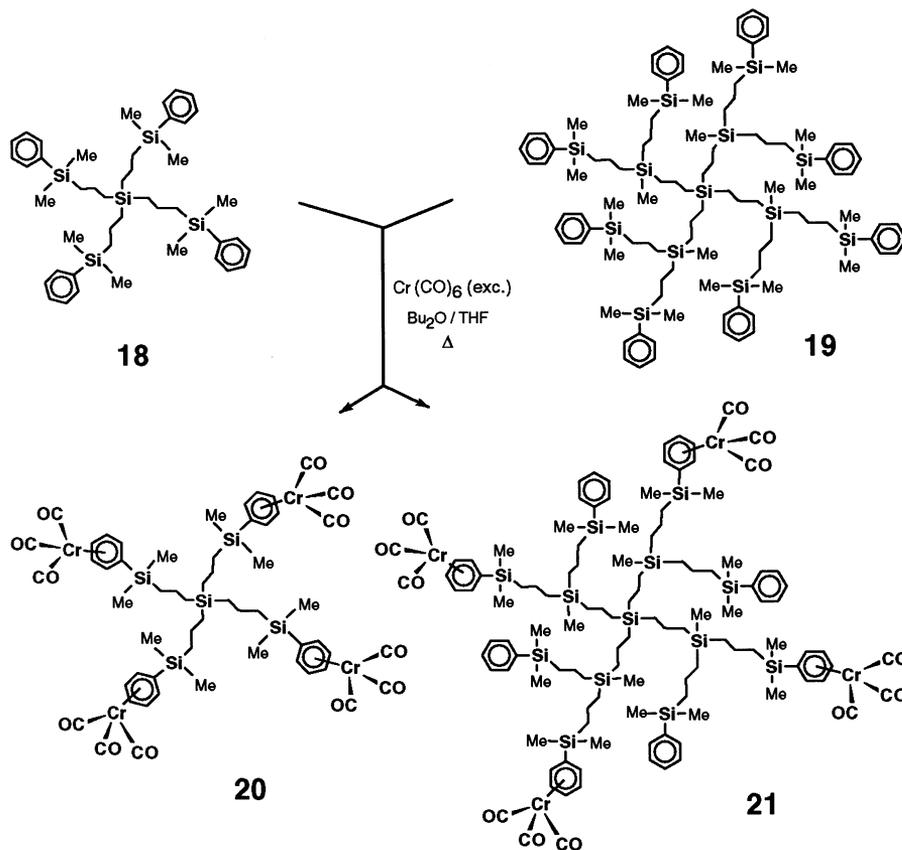
Scheme 7. Phenyl-terminated dendrimers and functionalization with  $\text{Cr(CO)}_3$  units.
