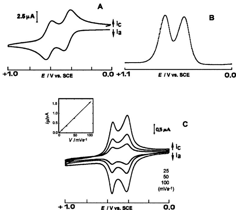
Fig. 7. Cyclic voltammogram (scan rate  $100 \text{ mV s}^{-1}$ ) (A) and DPV (B) of **49** in  $\text{CH}_2\text{Cl}_2 + \text{CH}_3\text{CN}$  (5:1 by volume). Supporting electrolyte:  $0.1 \text{ M Bu}_4\text{NPF}_6$ , Pt-disk electrode. (C) Voltammetric response of a Pt-disk electrode modified with dendrimer **49**, measured in  $\text{CH}_2\text{Cl}_2 + 0.1 \text{ M Bu}_4\text{NPF}_6$ ; (Adapted from Ref. [59]).
