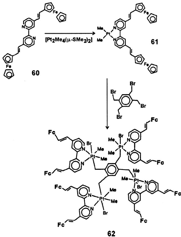
Scheme 22. Convergent synthesis of heterometallic dendrimers reported by Catalano et al.
