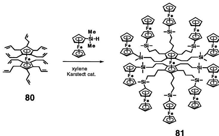
Scheme 29. Jutzi's synthesis of decaferrocenyl ferrocene.
