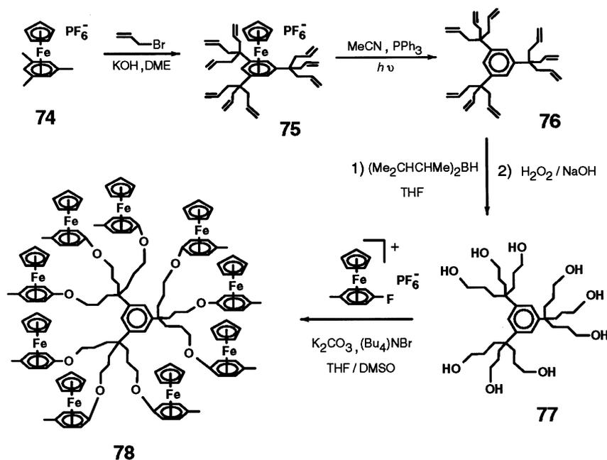
Scheme 27. Astruc's approach to the synthesis of a nonairon molecular tree.
