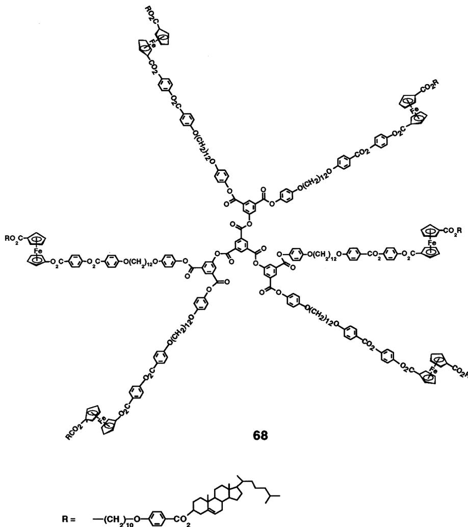
Scheme 25. A ferrocene-containing liquid crystal dendrimer synthesized by Deschenaux et al.
