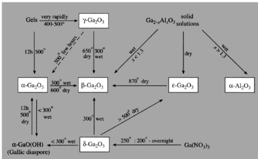
**Figure 7.13** Chart illustrating transformation relationships among the forms of gallium oxide and its hydrates. Conversion (wet) of the phase designated as  $\text{Ga}_{2-x}\text{Al}_x\text{O}_3$  to  $\beta\text{-Ga}_2\text{O}_3$  occurs only where  $x < 1.3$ ; where  $x > 1.3$  an  $\alpha\text{-Al}_2\text{O}_3$  structure forms.
