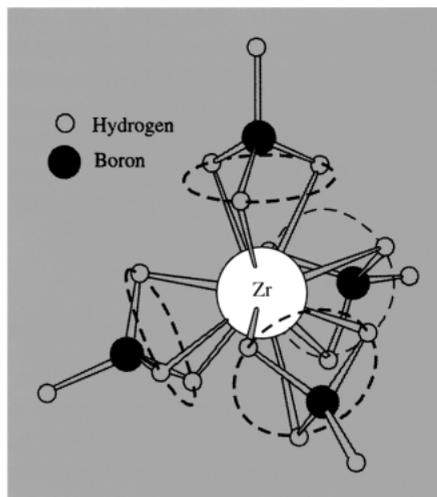
**Figure 21.7** Molecular structure  $[\text{Zr}(\text{BH}_4)_4]$  showing 4 trihapto  $\text{BH}_4$  groups.
