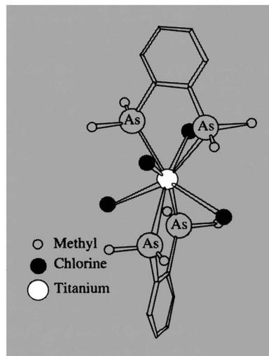
**Figure 21.5** Molecular structure of  $[\text{TiCl}_4(\text{diars})_2]$ . The dodecahedral coordination is produced by two interpenetrating tetrahedra (slightly distorted) of chlorine and arsenic atoms.
