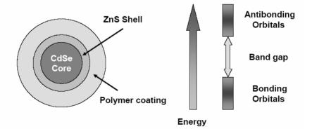
**Figure 2.8:** The organization of fluorescence quantum dots. The quantum dots are composed of a semiconductor core surrounded by a shell structures that are usually coated with some polymers to give them specific properties (e.g., negative or positive charge or functional chemical group). The fluorescence proprieties of the quantum dots arise from the energy gap of the confined electronic structures.
