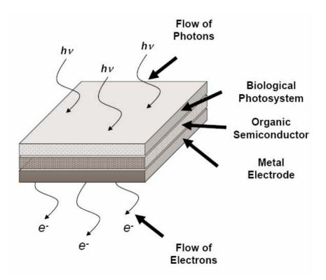
**Figure 8.3: Biomolecular solar cell.** As in silicone and other semiconductor-based photovoltaic cells, the biomolecular solar cell is based on the flow of electrons by the excitation of a semi-conductive material by electromagnetic radiation. The biological photosystem can significantly improve the efficiency of photon collection from the solar radiation.
