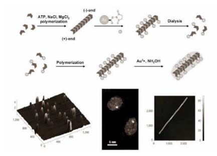
**Figure 7.6: Metal coating of actin fibrils.** The fibrils are chemically reacted to bind gold nano-particles, dialyzed, and re-polymerized with additional building blocks followed by gold enhancement. This results in continuous gold wires at the nano-scale. Reprinted by permission from Macmillan Publishers Ltd: Nature Materials (Patolsky *et al.*), copyright (2004). Courtesy of Itamar Willner.
