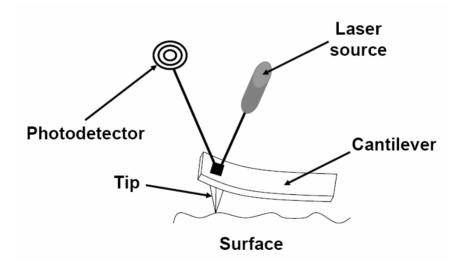
**Figure 2.2:** The principle of action of the atomic force microscope (AFM). A very fine tip travels over the surface of the sample. The topographic properties of the scanned surface affect the reflection of the laser light from the cantilever. The changes in the reelection are being translated into a three dimensional map of the scanned surface.
