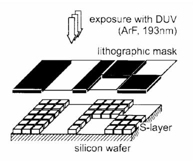
**Figure 7.1:** Schematic drawing of the patterning of an S-layer on a silicon wafer by DUV radiation using an ArF excimer laser. Courtesy of Uwe Sleytr.
