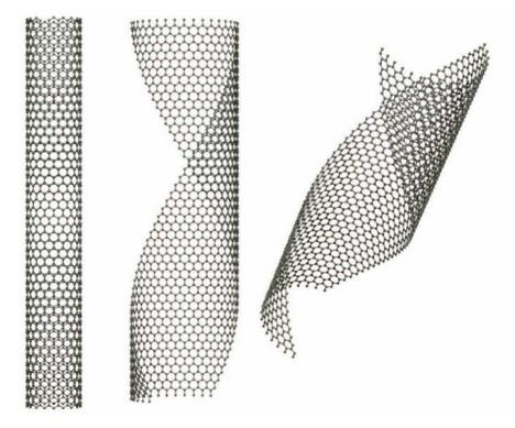
**Figure 2.5:** Model for the formation of carbon nanotubes by the two dimensional graphite-like layer. The tubes presented here are single-walled, although double-walled and multi-walled carbon nanotubes also present. Courtesy of Chris Ewels (©Chris Ewels www.ewels.com).
