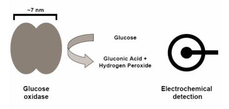
**Figure 1.2:** Detection of glucose level is based on the combination of enzymatic reaction and electrochemical detection. Hydrogen peroxide is being formed upon the oxidation of glucose by the glucose oxidase (GOX) enzyme. The level of the redox reaction is being determined electrochemically. In principle the reaction can be performed on the nanoscale as the size of the enzyme is less than 10 nm.
