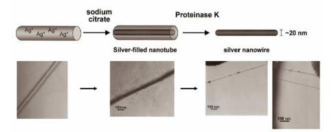
**Figure 7.7: Formation of silver nanowires with peptide nanotubes templates.** Ionic silver is reduced to metallic silver within the tube lumen. The peptide envelope is then removed by the use of enzymatic degradation. Modified from Reches and Gazit (2003).
