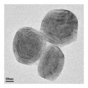
Figure 2.6: TEM micrograph of MoS2 fullerene-like nanoparticles. Courtesy of Reshef Tenne.
