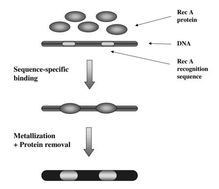
**Figure 7.4:** The use of the RecA protein for "molecular lithography". The RecA protein specifically binds to the unique sequence with the DNA and prevents the metallization of the specific region.
