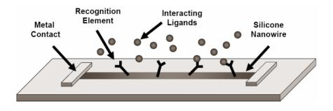
**Figure 8.2: The use of silicone nanowires for the detection of biological interactions.** The binding of charged ligands affects the current of either p-type or n-type silicone nanowires. The level of interaction could be monitored in real-time to provide information not only on the amount of the ligands but also on the kinetics of the association and dissociation.
