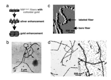
**Figure 7.5: Metal coating of the nano-scale protein amyloid fibrils. a.** Colloid gold binds to specific thiols within the amyloid building blocks, followed by silver and gold enhancements to achieve metal coated fibrils as observed by various microscopy techniques (**b-d**). Reproduced from Scheibel *et al.*, (2003) with permission. Copyright (2003) National Academy of Sciences, USA.
