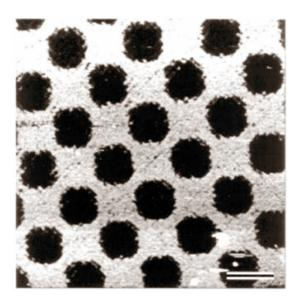
**Figure 7.2:** Scanning force microscopical image of a patterned S-layer on a silicon wafer. The bar represents a distance of 1000 nm. Courtesy of Uwe Sleytr.
