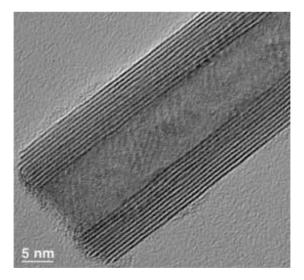
Figure 2.7: Transmission electron microscopy of  $WS_2$  nanotubes. Courtesy of Reshef Tenne.
