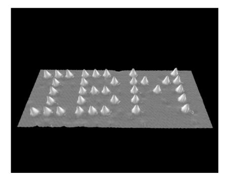
**Figure 2.3:** Spelling of "IBM" using 35 xenon atoms on a nickel surface. Courtesy of Dr. Donald Eigler. Image reproduced by permission of IBM Research. Unauthorized use not permitted.
