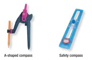
The A-shaped compass usually has a point and a pencil or lead point. The two legs of the compass are on a hinge so they can be adjusted for different settings. This kind of compass is often used by engineers and cartographers, people who draw maps. One use of a compass is to compare lengths of segments.
