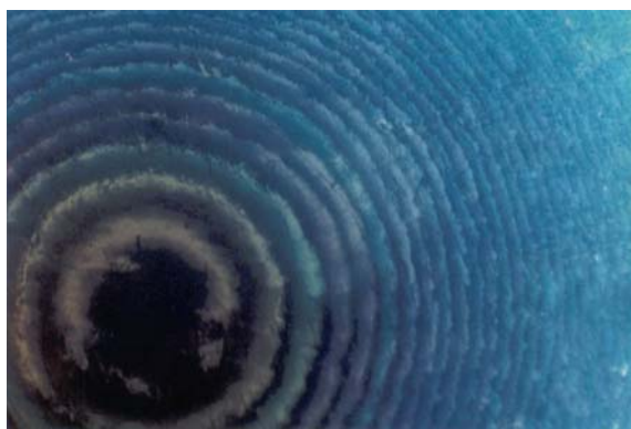
Plate 27. Preparation of a cholesteric sample in the Cano geometry between a planar substrate and a lens with the N^* helix axis being parallel to the direction of light propagation. The pattern of concentric rings can be used to determine the value of the cholesteric pitch. (Courtesy of W. Kuczynski.)
