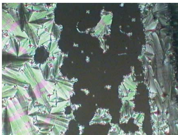
Plate 86. Planar and homeotropic regions at the transition from (a) \text{SmC}_{1/3}^* to (b) \text{SmC}_A^* . The so-called “ferrielectric” phase can easily be identified in the homeotropic sample area, due to a strongly fluctuating texture. Note that, in contrast to the grayish homeotropic \text{SmC}^* phase, the \text{SmC}_A^* appears black (pseudo-isotropic).
