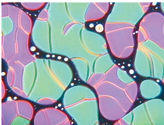
Plate 24. Same sample as Plate 23 at a slightly lower temperature, showing coalescence of the cholesteric droplets during the phase ordering process.
