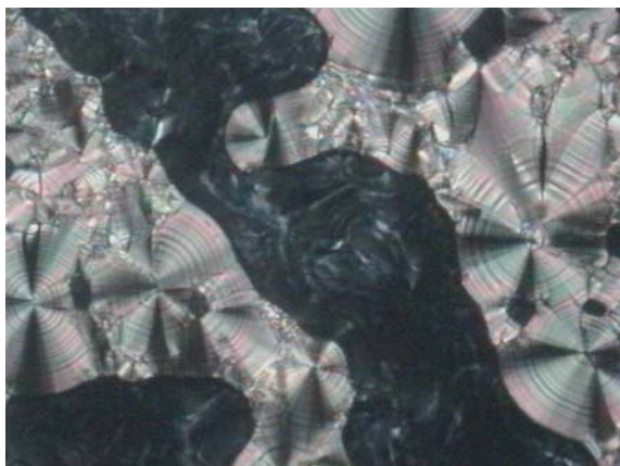
Plate 98. Coexisting planar and homeotropic regions of a soft crystal E phase.
