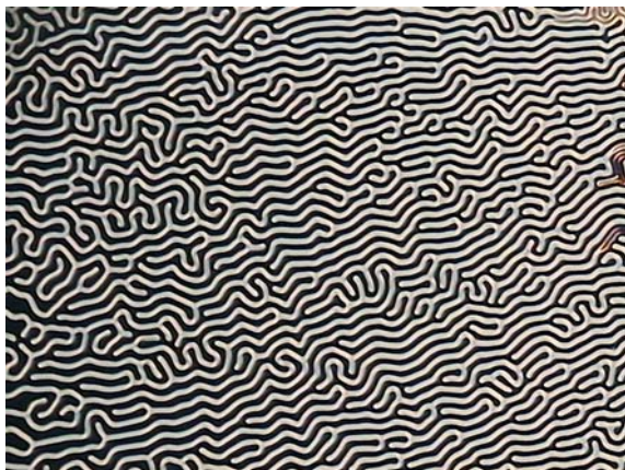
Plate 33. Sample with a diverging cholesteric pitch under homeotropic anchoring conditions, exhibiting so-called cholesteric fingers. In the strongly distorted director configuration, the dark areas represent a pseudo-isotropic, homeotropically aligned nematic.
