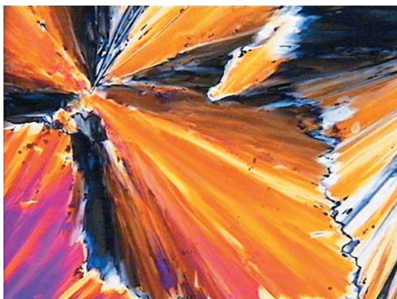
Plate 103. A crystalline phase after completed spherulite growth.
