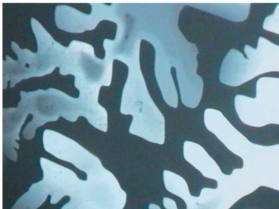
Plate 90. At the direct formation of the SmB phase (bright) from the isotropic melt (black), dendritic growth aggregates are often observed.
