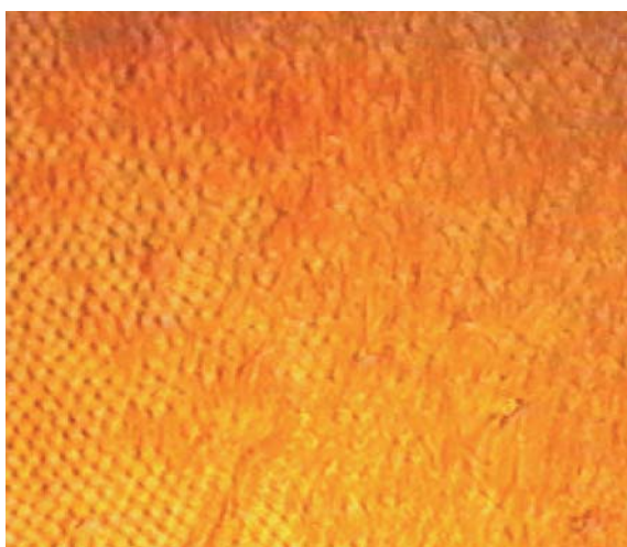
Plate 57. Square grid texture of the TGBC* phase under planar boundary conditions. The TGB helix is oriented perpendicular to the bounding plates, i.e. parallel to the direction of light propagation. The square grid pattern is presumed to be due to a helical director configuration within the individual SmC* blocks, with the helix axis being in the plane of the substrate and mutually perpendicular in adjacent smectic blocks. Another model of the square grid texture is that of the undulated twist grain boundary C* phase.
