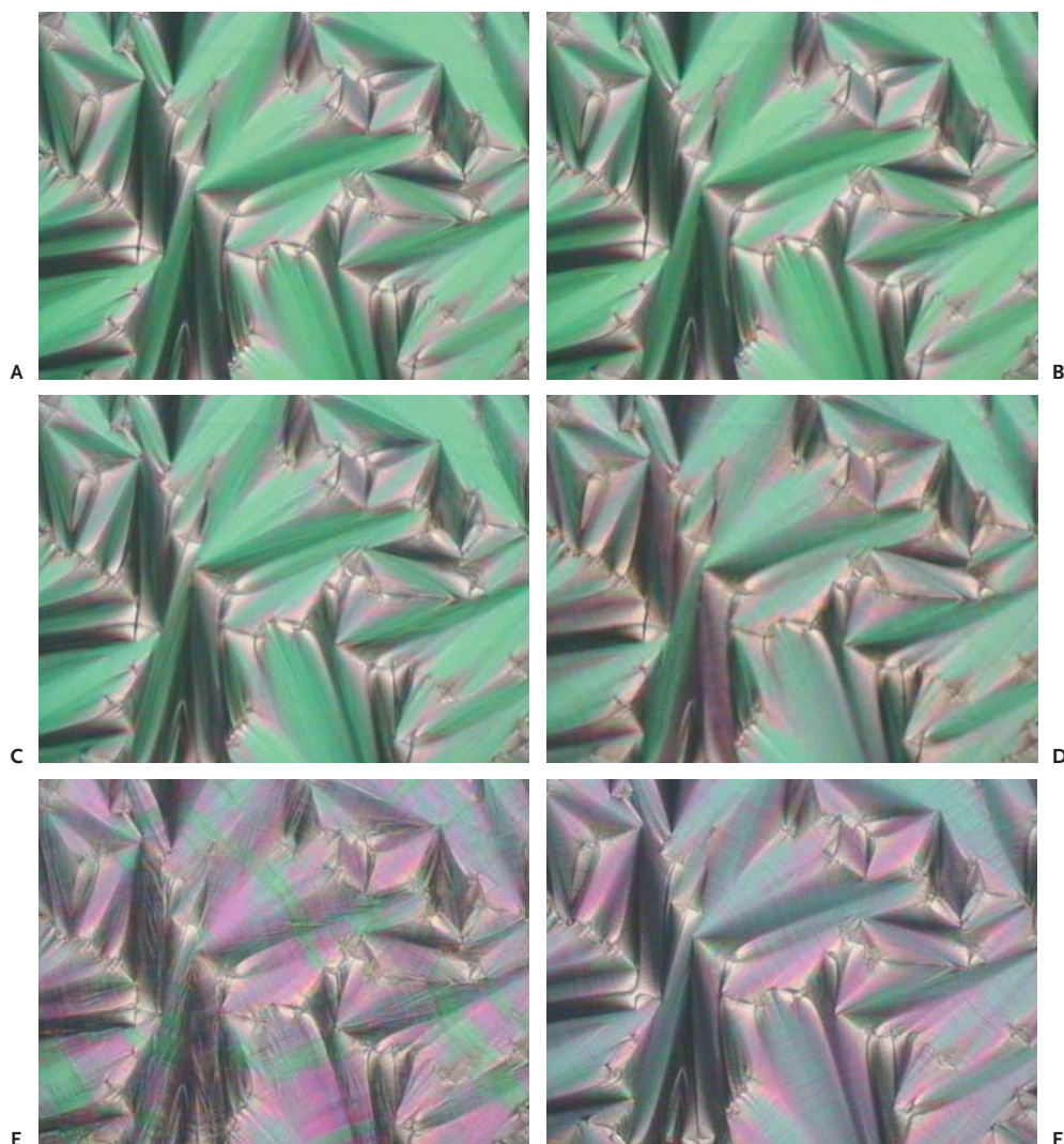
Plate 82. Texture series of MHPOBC showing the transitions through a number of different fluid smectic phases at the same sample region. Texture changes between (a) \text{SmA}^* , (b) \text{SmC}_a^* and
