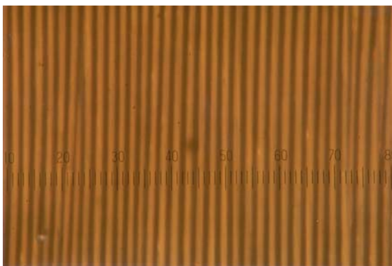
Plate 66. Electric field induced striped texture of a SmA* phase. The width of the stripes is approximately equal to the cell gap, in the present case approximately 6\text{ }\mu\text{m} .
