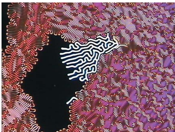
Plate 32. Coexistence of a cholesteric fingerprint texture with so-called cholesteric fingers (bright lines in the center) and a pseudo-isotropic region with a homeotropic nematic director configuration (black).
