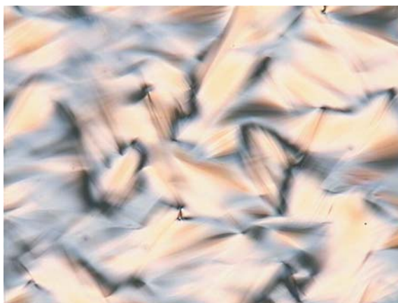
Plate 38. Textures of twist grain boundary phases often appear blurred and are hard to focus, like the fan-like texture of the TGBA^* phase depicted in this texture photograph.
