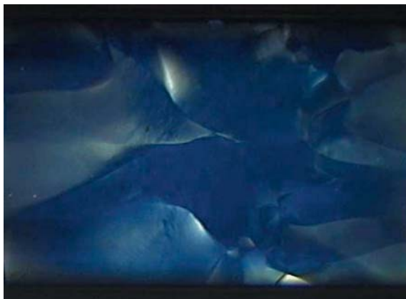
Plate 7. Typical texture of a smectic blue phase. (Courtesy of E. Grelet, B. Pansu, M. H. Li and H. T. Nguyen.)
