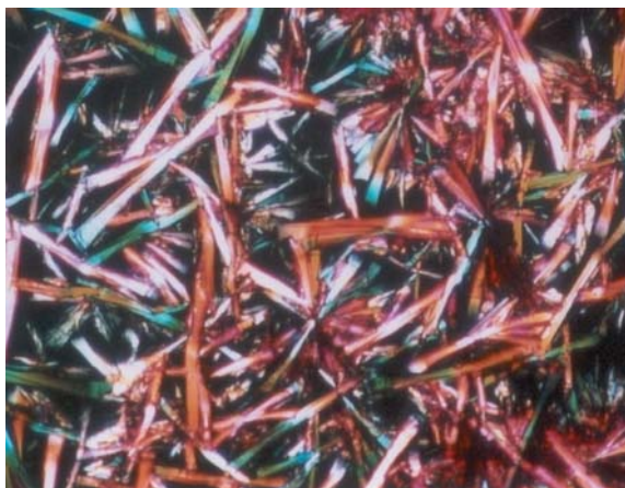
Plate 104. Needle growth during direct crystallization from the isotropic melt, without mesogenic behavior.
