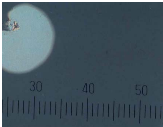
Plate 25. Two twist states of a long pitch cholesteric phase between substrates with planar boundary conditions, differing by a \pi turn of the helical superstructure. The discontinuous pitch jumps can be observed as domains of a different color nucleating and growing from a uniform N^* twist state. The different colors are not related to selective reflection.
