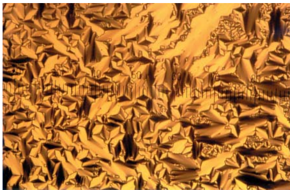
Plate 19. Fan-like texture of a short pitch cholesteric phase. Within individual fans the helix axis (equivalent to the optic axis) is oriented uniformly.
