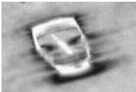
Fig. 11.5. Texture of a nematic liquid crystal, whose defect lines resemble a face, smiling at you. Application of an electric field of moderate amplitude pronounces the smile. (Image was taken by D. Green. Courtesy of H. F. Gleeson.)
