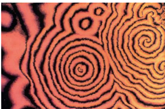
Plate 81. The smectic layer rotation under applied asymmetric electric fields can lead to spiral smectic layer instabilities, shown here for a \text{SmA}^* phase close to the transition to \text{SmC}^* . (Courtesy of G. Andersson.)
