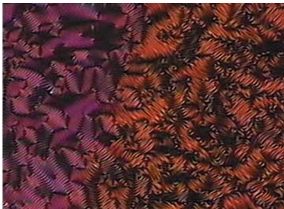
Plate 46. Sample on cooling under homeotropic boundary conditions at the transition from N^* (fingerprint texture at the right) to TGBA^* (filament texture at the left).
