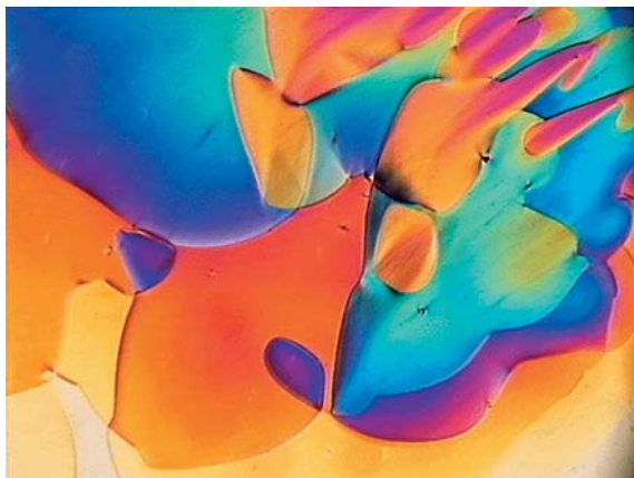
Plate 43. ATGBA* phase with relatively long pitch at planar anchoring conditions in the Grandjean orientation. The helix axis is parallel to the direction of light propagation and different colors are due to different twist states developing during cooling.
