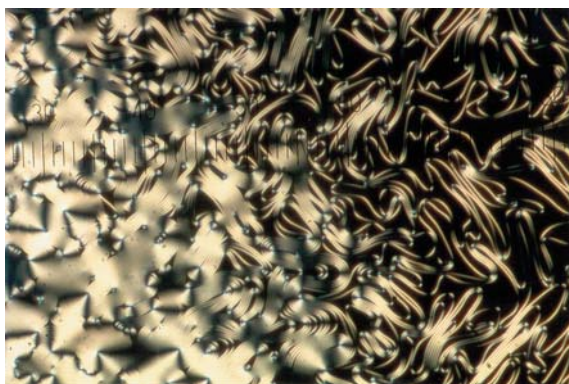
Plate 50. Same sample area as in Plate 49 at a slightly lower temperature. The TGBA* phase can be observed by its typical filament texture, while the pseudo-isotropic texture of the SmA* phase is seen as black areas, because here the optic axis is oriented along the direction of light propagation. (Reproduced by permission of Taylor & Francis, I. Dierking et al., Liq. Cryst. , 17 , (1994), 17 ( http://www.tandf.co.uk/journals ).)
