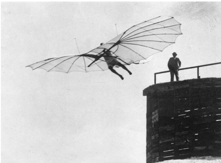
Fig. 1.7 Lilienthal’s glider flights were based upon experiments concerning the drag and lift of curved surfaces (Source: Deutsches Museum, Munich).
