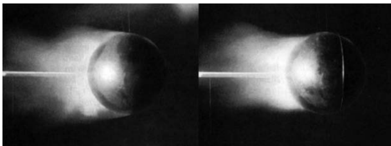
Fig. 2.12 A trip wire around a sphere (right image) makes the boundary layer turbulent, resulting in a smaller vortical wake and therefore a decrease of the drag.
