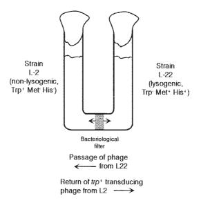
Fig. 9.1. Diagram of the U-tube apparatus used to analyze the transduction process. Two populations of cells are separated by a filter preventing cell passage. Fluid is pumped between the compartments by applying air pressure alternately to the upper openings. See text for details of experiment.
