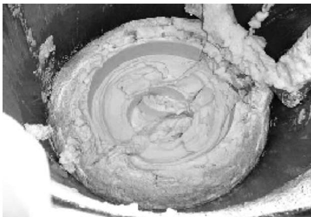
**Fig. 12** White precipitate at the bottom of the fermenter
