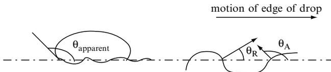
**Figure 6.8.** Schematic of a drop on a rough surface. Here, we measure an ‘apparent’ contact angle, and hence the differences between the advancing and receding angles, even though the true contact angle does not alter ( $\sim 90^\circ$  in the figure).
