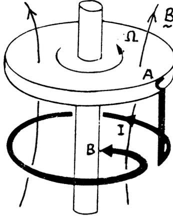
Figure 24: The homopolar generator.
