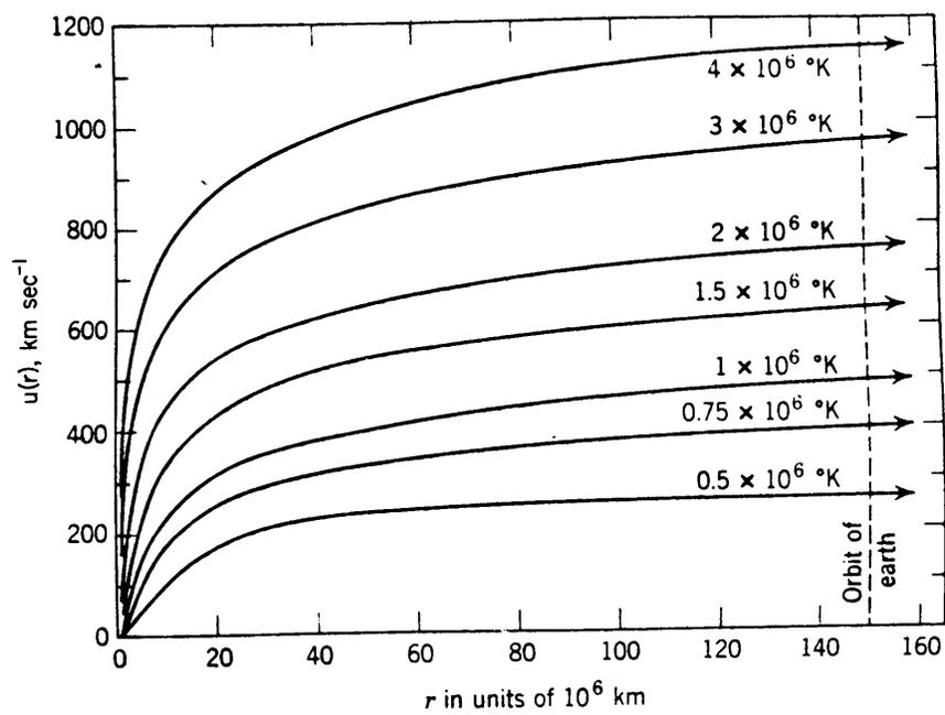
Figure 20: Parker outflow solutions for the solar wind.
