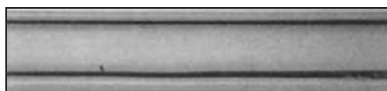
Stratified regime: wavy flow pattern
