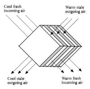
Figure 4.6 Air to air plate heat exchanger
