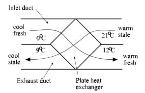
Figure 4.5 Location of plate heat exchanger in the ducting
