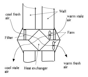
Figure 4.1 Ventilation unit with heat recovery
