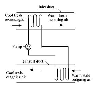
Figure 4.8 Run around coil
