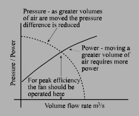
Figure IP11. Fan characteristic (radial bladed centrifugal fan)
