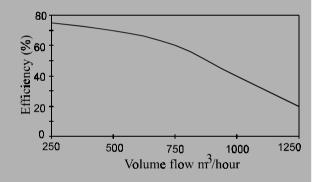
Figure IP12 graph of efficiency against airflow rate
