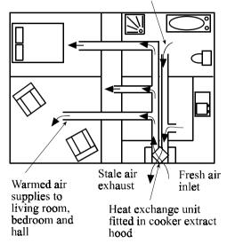
Figure 4.2 Whole house ventilation with heat recovery
