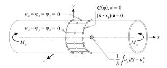
Fig. 27. Kinematic boundary conditions for a pipe segment in pure bending.
