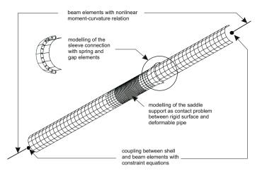
Fig. 26. FE-mesh for two adjacent pipes.
