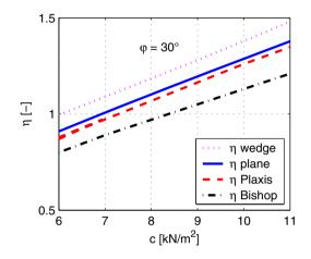
**Fig. 15.** Factor of safety  $\eta$  (14) for the slope in Fig. 1 calculated with different mechanical models:  $\eta$  wedge: wedge analysis with rigid bodies;  $\eta$  plane: planar shear surface;  $\eta$  Plaxis: finite element calculation, reduction of the shear parameters;  $\eta$  Bishop: BISHOP's method, circular shear surface
