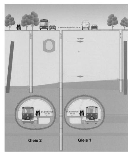
Fig. 14. Munich Trudering station – cross section
