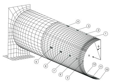
Fig. 21. FE-mesh for the pipe segment.
