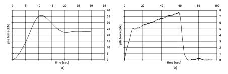
Fig. 37. Changes of the pile force due to a) removal of a sheet pile b) surface loads heavy truck.
