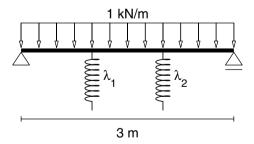
Fig. 1. Beam bedded on two springs.
