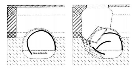
**Fig. 6.** Municipal railway tunnel, Bochum. Diagram of the tunnel collapse (after L. Müller 1978) [16]
