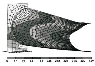
Fig. 22. Contour plot of the v. Mises equivalent stress for the pipe segment.
