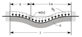
Fig. 31. Beam on elastic foundation.
