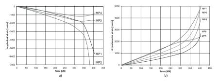
Fig. 18. Measured a) longitudinal and b) circumferential strains.
