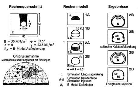
Fig. 8. Computational model for tunnel driving in soil, Farchant tunnel [15]
