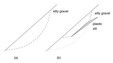
Fig. 3. Change of the shear surface, due to a weak layer: (a) In homogeneous conditions the shear surface (dashed line) can be assumed as a circular slip curve.
