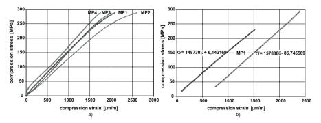
Fig. 11. Compressive stress-strain curves from stub-column tests; a) loading branches; b) individual loading and unloading branch.
