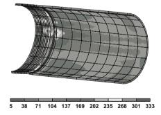
Fig. 5. Contour plot of the v. Mises equivalent stress  $[N/mm^2]$  of the pipe in the vicinity of the sleeve
