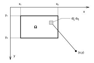
Fig. 4. Uniformly distributed load over a rectangular area.
