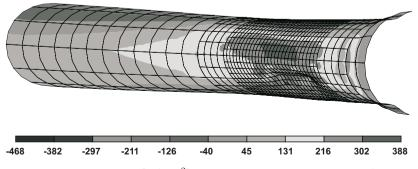
Fig. 34. Axial stress [N/mm<sup>2</sup>] for a pile-supported pipe DN600/K8.
