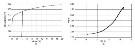
Fig. 12. Material behavior in tension: a) true stress-strain curve for loading, unloading and reloading; b) logarithmic diagram of plastic strains.
