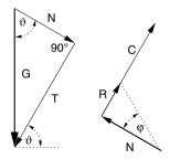
**Fig. 4.** Disturbing force T and resistance force R + C.
