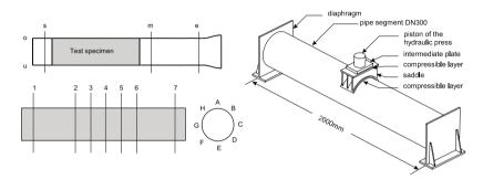
Fig. 6. Pipe segments and test set-up.
