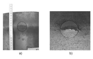
Fig. 16. Fracture at the a) outer surface of a stub-column test specimen due to b) a sinkhole at the inner surface of the specimen.
