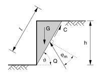
**Fig. 2.** Geotechnical model: planar failure surface.
