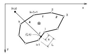
Fig. 3. Polygonal approximation of the loaded area.
