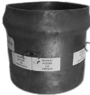
**Fig. 10.** Axially loaded pipe with  $L/D=1$  after testing.
