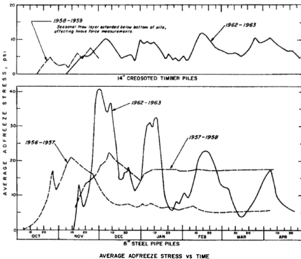
(Average tangential Adfreeze bond stress versus time, and timber and steel pipe piles with silt-water slurry in dry excavated holes. Piles were installed within annual frost zone only, over permafrost, to depths from ground surface of 1.1 to 2 meters (3.6 to 6.5 feet).)
