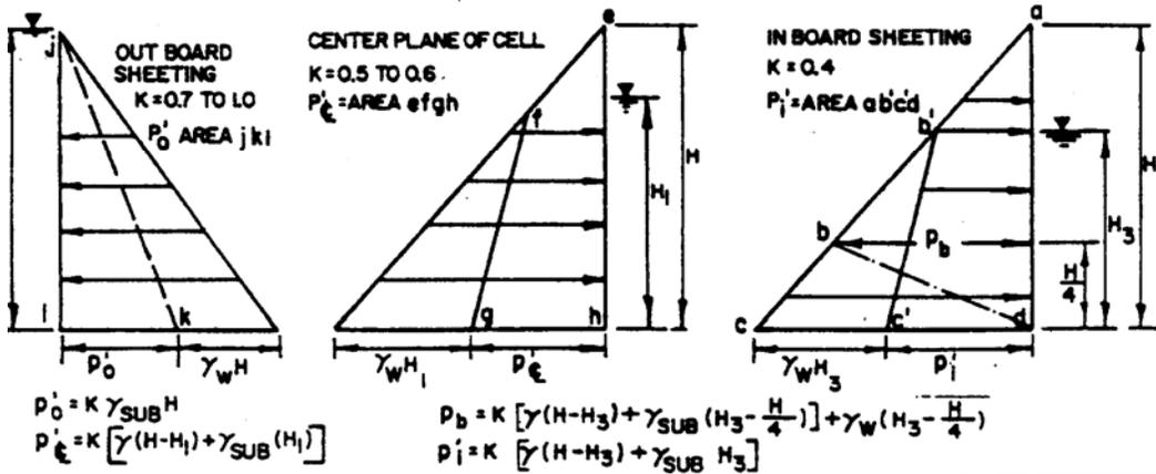
Figure 6-1 Design Criteria for Cellular Cofferdams
