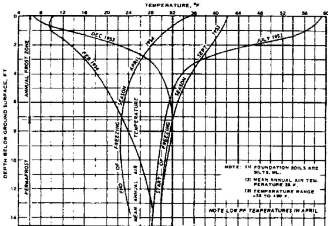
Figure 11-3 Ground Temperatures During Freezing Season in Fairbanks, Alaska
