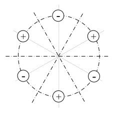
Fig. 1.4 Image charges for planes intersecting at 60°
