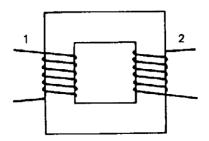
Fig.6.2. The arrangement of a simple transformer
