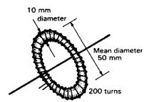
**Fig. 6.5.** A toroidal coil can be used as a transducer to measure the current in a conductor which passes through it.
