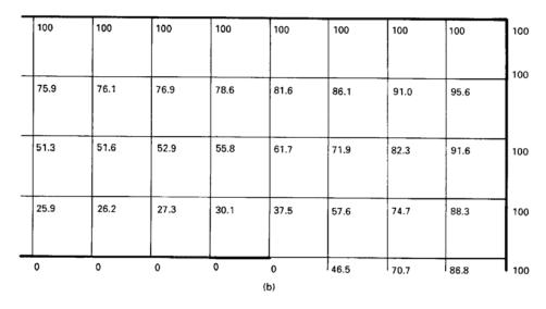
Fig.1.18. The finite difference solution for one quadrant of the problem: The final solution.
