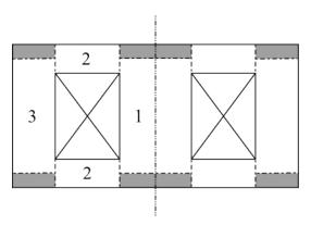
Fig. 5.9. The sections of the magnetic circuit.
