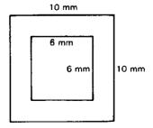
Fig. 2.14. Square coaxial electrodes
