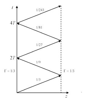
Fig. 7.4. Time of flight diagram for example 7.2
