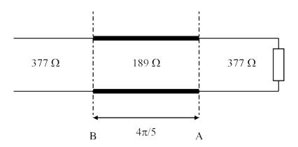
Fig. 8.1. Transmission line equivalent circuit for example 8.4
