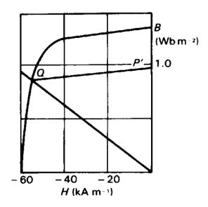
Fig. 5.12. The demagnetization curve for Columax.
