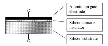
Fig. 2.1 Arrangement of layers in a MOS transistor.
