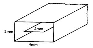
Fig. 7.9. A square coaxial transmission line
