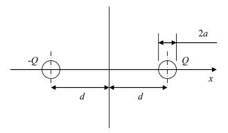
Fig. 1.11 The arrangement of the sphere and its image in the plane.
