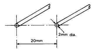
Fig. 7.8. Air-spaced two wire transmission line
