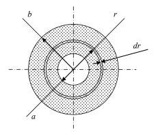
Fig. 3.1. Arrangement of a coaxial cable.
