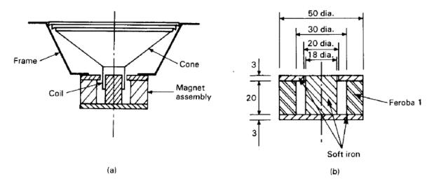
**Fig. 5.14.** (a) A cross-sectional view of a moving-coil loudspeaker. The coil is placed in the air gap of the magnetic circuit so that it experiences an axial force when a current is passed through it. The movement of the coil is transferred to the air through the motion of the paper cone. (b) An enlarged view of the magnet assembly.
