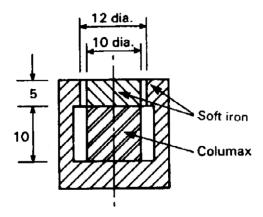
**Fig. 5.16.** The arrangement of a Columax loudspeaker magnet. Notice how the use of a magnet material with a higher energy product allows the permanent magnet to be put at the centre instead of outside as shown in Fig. 5.13(b).
