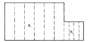
**Fig. 3.10** Approximate equipontential surfaces to find a lower bound for the resistance of the strip shown in Fig. 3.7.
