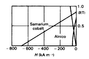
Fig. 5.18. The demagnetization curves for Alnico and samarium cobalt (SmCo<sub>s</sub>).
