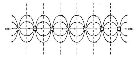
Fig. 1.6 The field pattern around a set of equispaced parallel wires charged alternately positive and negative.
