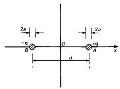
Fig. 2.3 Cross-sectional view of a parallel-wire transmission line
