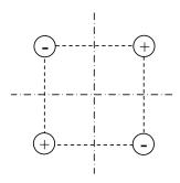
Fig. 1.3 Image charges for planes intersecting at 90°
