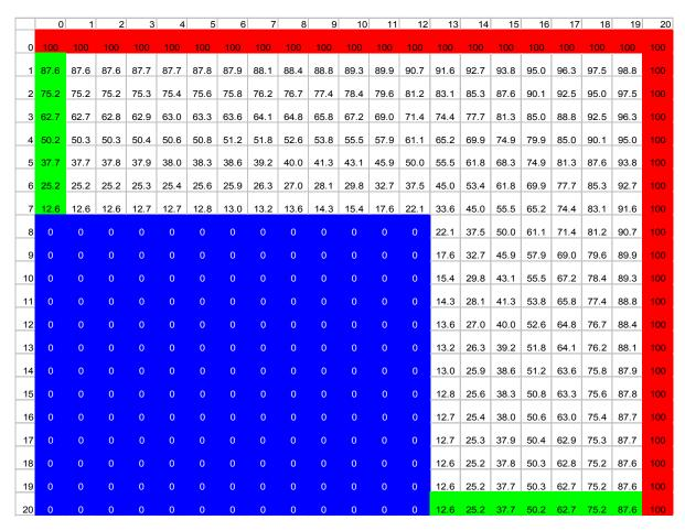
**Fig.1.20**. Finite difference calculation of the problem. Mesh step = 0.25 mm. The red and blue areas contain fixed potentials. The white area contains the standard formula and the green areas use formulae which assume symmetry at the boundaries.
