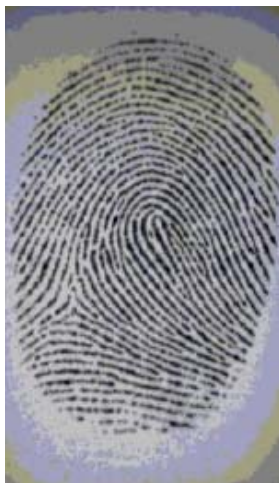
Figure 15: After Enhancement and compression PSNR = 28.87 dB
