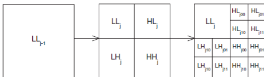
Figure 3: Image wavelet decomposition and Haar transform of high-frequency sub-images
