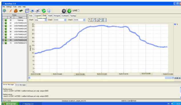
Fig. 4.b Evolution of temperature on the panel during 24 hours
