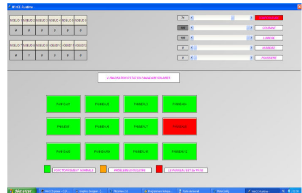
Fig 5.a: Case of dangerous Fault in Panel number 8 due to Temperature
