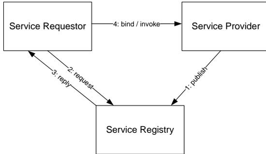
**Fig. 2.21.** Roles in service-oriented architectures
