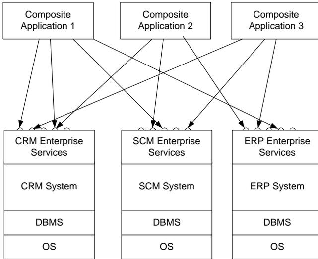
**Fig. 2.23.** Enterprise systems expose functionality through enterprise services
