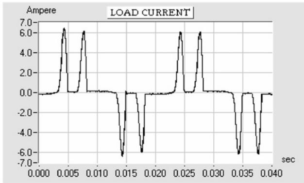
**Fig. 11.5.** Example of diode bridge polluting current.
