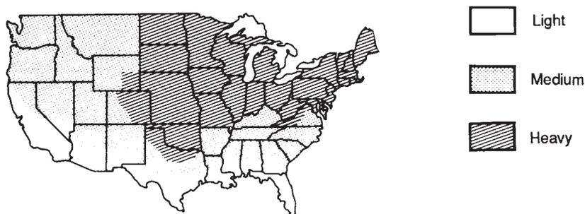
**Figure 2-7. Wind and ice load specifications.** Map shows territorial division of the United States with respect to wind and ice loading of overhead lines. Alaska is in the heavy zone and Hawaii is in the light. (*National Electric Safety Code*)
