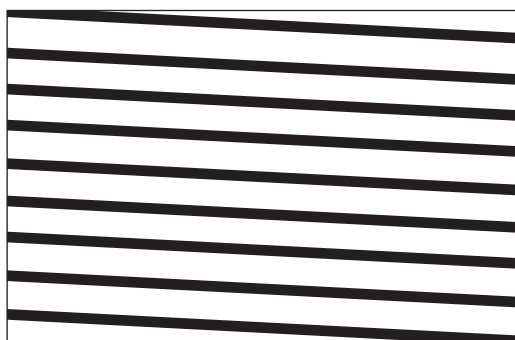
Figure 7.4 Effects of maladjusted timebase controls
