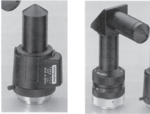
Figure 6.16 Typical pinhole lenses for covert applications. A right angled lens may be used where a covert camera is to be installed in a restricted space. (Photos courtesy of CBC (Europe) Ltd, manufacturers of Computar Lenses)
