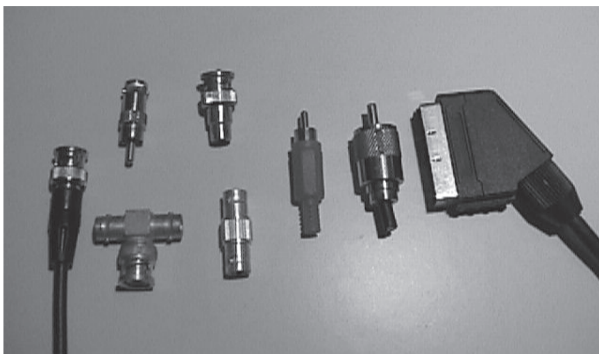
Figure 2.22 Range of connectors. From left to right: BNC crimp, BNC T coupler, BNC straight coupler, two variations of BNC/phono adapter (top), Phono, UHF, SCART
