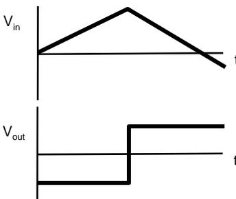
As the frequency of the input becomes larger, the slope of the input increases and thus the magnitude of the output increases, i.e. gain increases with increasing frequency.
