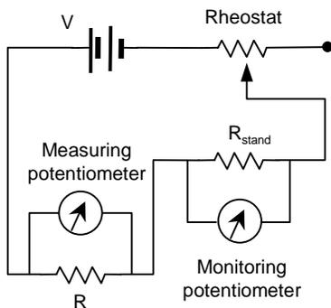
The resistance of the sensor changes with temperature. When the resistance changes, the current in the circuit changes. The rheostat is adjusted to bring the current back to its former value. This can be achieved by keeping the voltage across the standard resistor a constant using the rheostat. The change in voltage on the measuring potentiometer is thus due to a change in temperature only.
