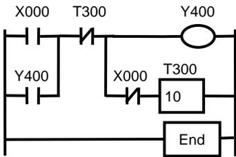
In this example, when the input X000 is true, there is logic continuity through the normally closed timer contacts T300 to the output Y400. This true state is fed back into the input to the normally closed contacts of the timer. Thus, when the input X000 goes false, the output Y400 remains on, it is **latched** by its own contacts.
