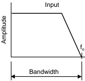
The Nyquist criterion requires us to sample the input at a frequency of at least twice that of the highest frequency component of the input signal:  $f_s \gg 2f_0$
