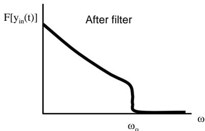
The resulting Fourier series or integral (using the modified transform as the amplitude coefficients) then represents the **filtered signal** in which noise is reduced.
