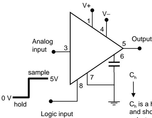
When logic input is high, output follows any changes in the analog input. When logic input goes low, the analog input signal is captured and passed through to the output. Output remains fixed at this value while logic input is held low.
