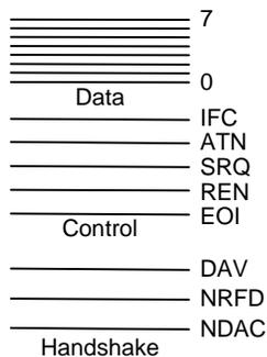
8-bit data can be transmitted in parallel, each bi-directional line carrying 1 Mbit/second. A maximum total cable length of 20 m with a maximum separation of 4 m between devices is recommended. Bus extenders and expanders can also be used.
