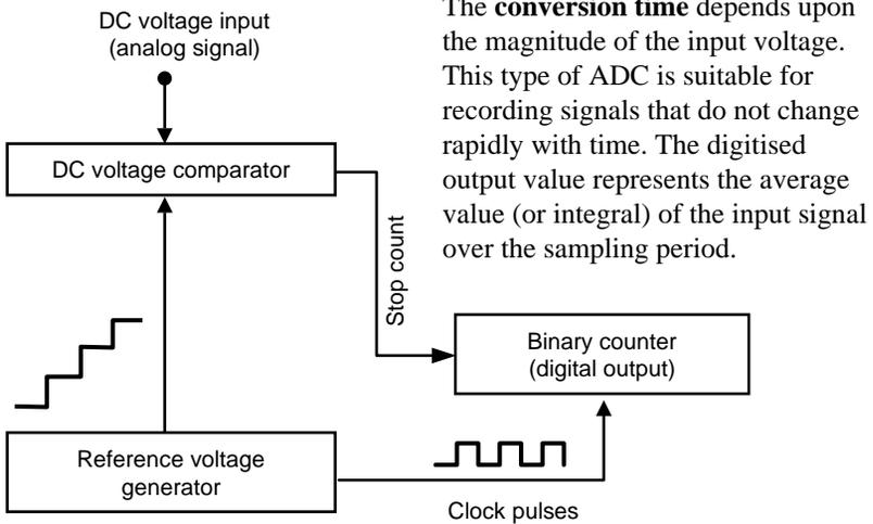
The **conversion time** depends upon the magnitude of the input voltage. This type of ADC is suitable for recording signals that do not change rapidly with time. The digitised output value represents the average value (or integral) of the input signal over the sampling period.
