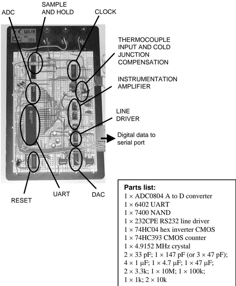
The ADC converts a 0–5 V analog signal to an 8-bit digital value (0–255). This digital value is passed through a UART which serialises the data into a bit stream for transmission over a single wire to the computer’s serial port.
