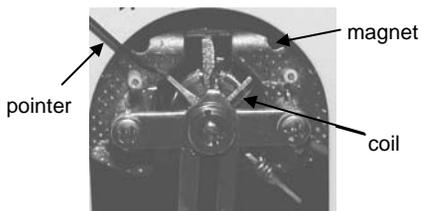
Although such a meter is designed to have a very high internal impedance, it has to draw some current from the circuit being measured in order to cause a deflection of the pointer. This may affect the operation of the circuit itself and lead to inaccurate readings – especially if the output resistance of the voltage source being measured is large.
