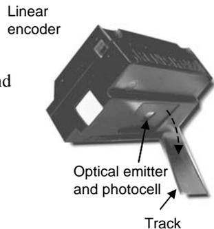
The output signal from an optical encoder may be a **quadrature signal**. The encoder produces two square waves out of phase by  $90^\circ$ . A motion controller can then extract four **phase changes** per cycle leading to a four-fold increase in step size. Some encoders can further **interpolate** the signals from the slots or gratings by up to a factor of 50. Step sizes of 0.1  $\mu\text{m}$  are routinely available with these types of encoders.
