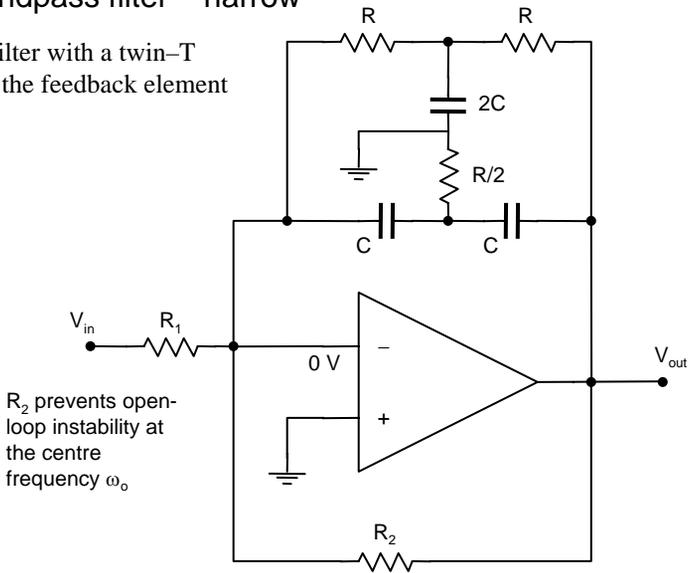
$R_2$  prevents open-loop instability at the centre frequency  $\omega_0$
