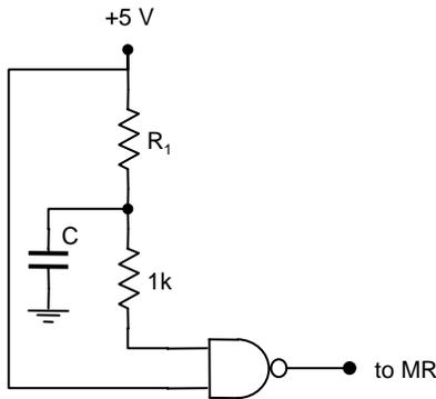
Initially, NAND output is at 0 V. When  $V_{cc}$  is applied, the NAND output goes to 1 since one input is at +5 V and the other at 0 V. As the capacitor charges up through  $R_1$ , voltage at upper input to the NAND rises and after a time characterised by  $R_1C$ , the NAND gate flips from 1 V to 0 V. The 1 k $\Omega$  resistor limits the current into the NAND for protection.
