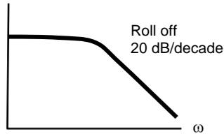
Two 1st order filters cascaded together produce a 2nd order filter:
