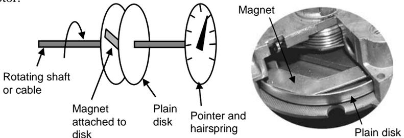
The disk is connected to a pointer and a hairspring. The scale is calibrated to indicate velocity in the desired units (e.g. mph or km/h).
