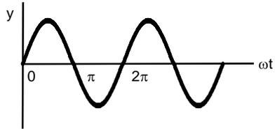
If we were to store this wave as a sequence of numerical data, we would choose data pairs  $(y,t)$  at convenient intervals. The smaller the interval, the more accurate the representation of the original signal when we come to reconstruct it from the data.
