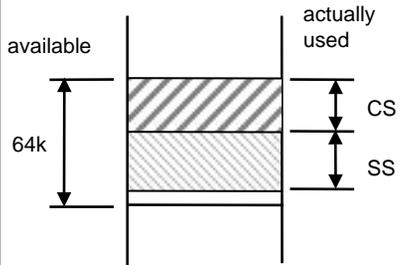
This example shows how the Stack Segment can be accommodated within a 64K block which is only partially used by the Code Segment.
