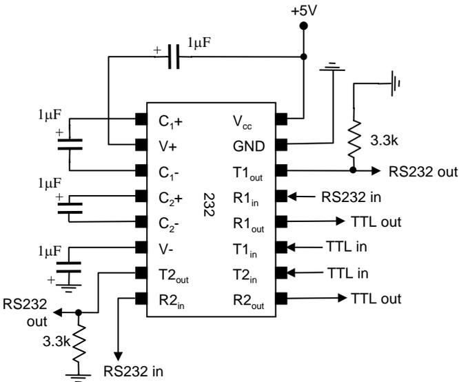
Transmitting: TTL input, RS232 output
