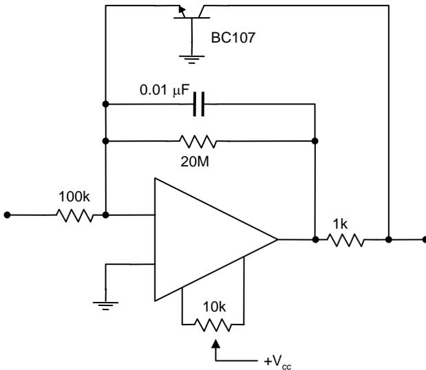
1. Connect the op-amp as an inverting amplifier with a gain of about 100 (i.e. do not use the transistor as a feedback element yet). With  $V_{in} = 0$ , balance the offset voltage to zero.
