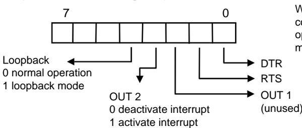
The MCR is not set by the 8250 UART itself. We must set bits in it to control the UART operation and/or the modem control lines.
