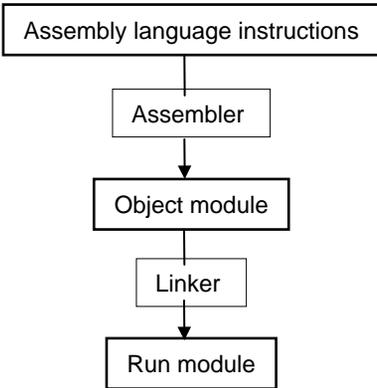
Source code in ASCII text. Symbolic labels are used in jumps so that absolute addresses need not be calculated by the programmer.
