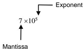
The computer stores the mantissa and the exponent in different places. In a simplified system, the mantissa may occupy 4 bytes of storage followed by a 1 byte exponent. Decoding of this format is typically done in software, although a specialised **maths co-processor** chip is fitted to most microcomputers to perform these conversion routines in hardware, and thus more quickly.
