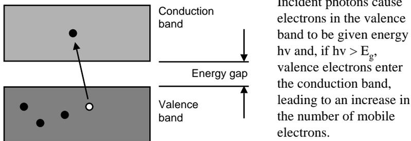
The increase in conductivity manifests itself as an increase in the current through the device for a given applied voltage and as such may be called a light dependent resistor (LDR).
