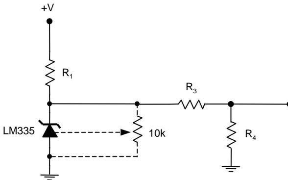
The nominal sensitivity of the LM335 is 10 mV/K and we need to factor this down to the  $\mu\text{V/K}$  range. We choose R<sub>3</sub> and R<sub>4</sub> so that:
