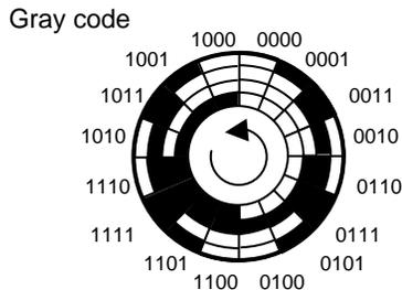
In the Gray code, only one track changes state at any one time during a rotation. Should a read error occur, then the resulting number will be in error by only one bit value. The Gray code is a **non-weighted** code. Any binary number can be converted into the Gray code, there is no upper limit to the number of code combinations. Conversion from Gray to binary can easily be done in a computer and so this code makes it ideal for this type of instrumentation purpose.
