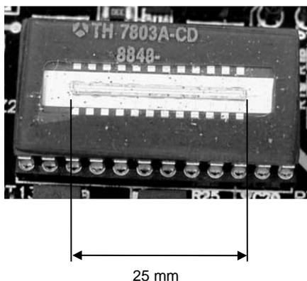
The output from a diode array is an analog signal that gives the distance from the edge of the array to the **centroid** of the incident light spot. The response of a diode array is very fast (**rise time**  $\approx 5 \mu\text{sec}$ ) and the device has very high **positional resolution** ( $\approx 250 \text{ nm}$ ) and a linearity of less than 1% of full scale.
