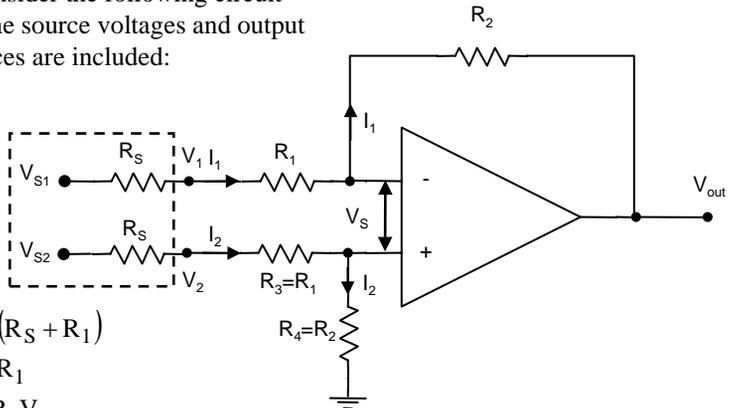
$$V_{S1} = I_1 (R_S + R_1)$$
