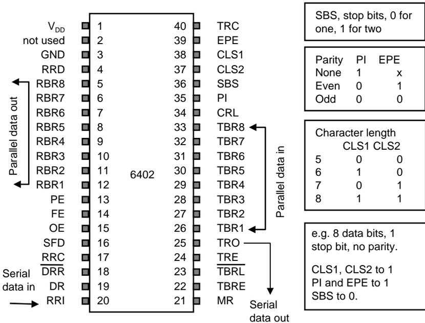
When TBRL goes low, data is read from the input pins TBR1–8 and transferred to the Transmitter Buffer Register. When TBRL goes from low to high, data is transferred from the Transmitter Buffer Register to the Transmitter Register whereupon data is shifted and transmitted out on TRO.
