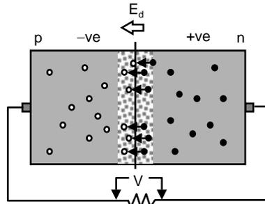
Current will flow in external circuit as long as photons of sufficient energy strike the material in the depletion region.
