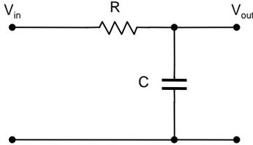
It can be shown that the output voltage is the time integral of the input voltage:
