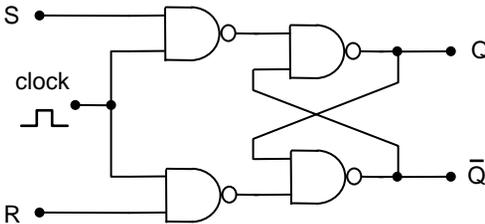
Data at terminal S gets transferred to Q on the clock pulse and remains at Q even if the signal at S disappears and the clock goes low.
