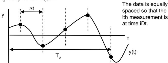
Thus, we can say that the continuous frequency spectrum of a **non-periodic** signal can be completely specified by a set of regularly spaced frequencies a minimum of  $\Delta\omega = 2\pi/T_o$  radians/sec apart. That is, for the purposes of analysis, we say that a **non-periodic signal of finite length** is periodic with a period equal to the length of the signal. The component frequencies consist of equally spaced intervals:
