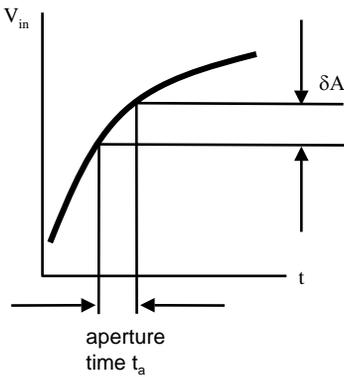
During conversion time, the signal changes. For there to be no error in the digitised output, this change must be less than the smallest increment registered by a single bit: i.e. the product  $(\delta)(A)$ .
