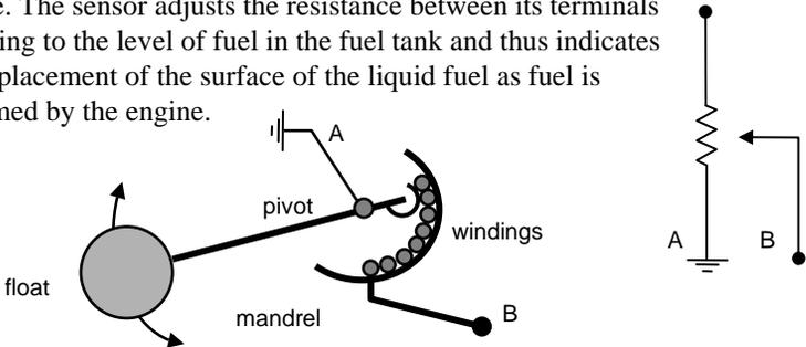
A non-linear response can easily be obtained by altering the dimensions of the **mandrel**. For example, to show a larger deviation in  $R$  at low fuel level (increased sensitivity), then the mandrel can be shaped or the spacing of the windings altered according to position.
