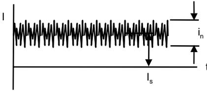
The signal-to-noise ratio is the ratio of the signal power over the noise power.
