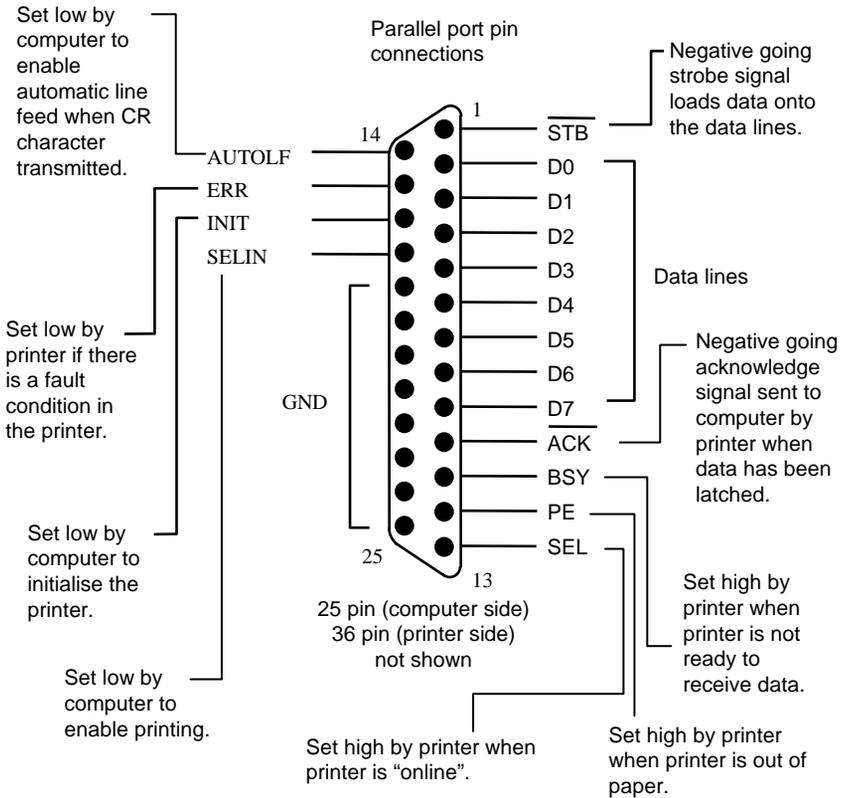
The printer port is driven by the parallel port adaptor. In the adaptor, there are three registers which are assigned I/O port addresses. The byte to be printed is held in the data register which is at the port base address. The printer status register contains the information sent to the computer by the printer, and has an address of base+1. The printer control register has address base+2 and contains the bit settings for computer control of printer functions.
