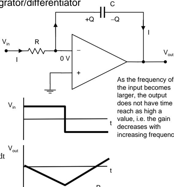
As the frequency of the input becomes larger, the output does not have time to reach as high a value, i.e. the gain decreases with increasing frequency.
