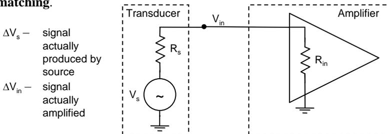
Ideally,  $R_{in} \gg R_s$  because otherwise, negligible  $\Delta V_{in}$  appears at the amplifier. That is, if  $R_s \gg R_{in}$ , then most of the voltage variations  $\Delta V_s$  appear across  $R_s$  and not at the amplifier input. Amplifiers should have a high input impedance  $R_{in}$  compared to  $R_s$ , the output resistance of the source.
