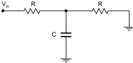
The **transfer impedance** of a network is defined as the ratio of the voltage applied to the input terminals to the current which flows at the output terminals when the output is grounded.
