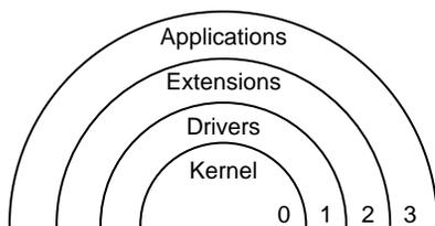
Unlike real mode operation, I/O operations from a user application do not have the required privilege level and so must perform these functions in conjunction with an I/O **device driver** which does. This ensures that I/O is done without violating not only the address space of another running application, but also that the I/O does not adversely affect the low level task sequencing and memory management responsibilities of the CPU.
