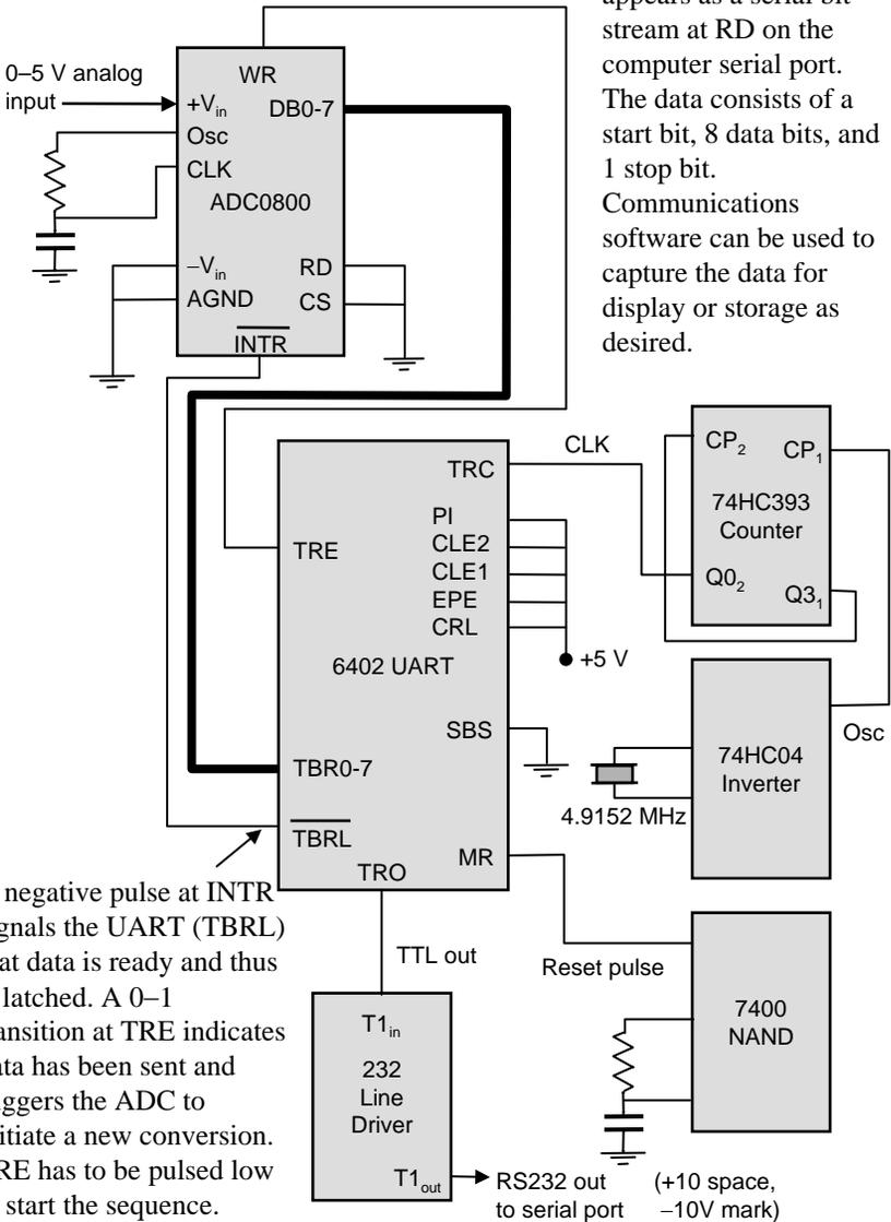
A negative pulse at INTR signals the UART (TBRL) that data is ready and thus is latched. A 0–1 transition at TRE indicates data has been sent and triggers the ADC to initiate a new conversion. TRE has to be pulsed low to start the sequence.
