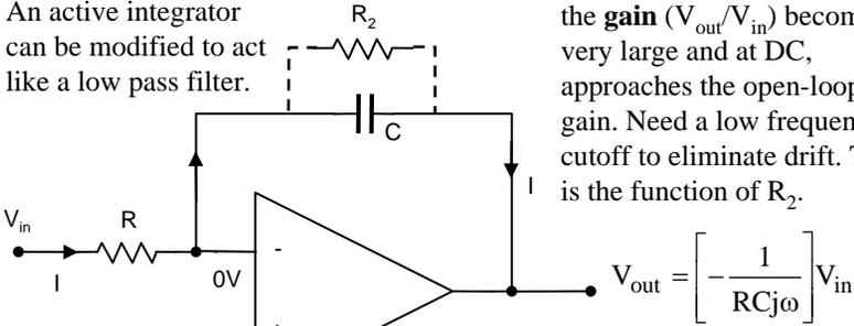
Without  $R_2$ , at low frequency, the **gain** ( $V_{out}/V_{in}$ ) becomes very large and at DC, approaches the open-loop gain. Need a low frequency cutoff to eliminate drift. This is the function of  $R_2$ .
