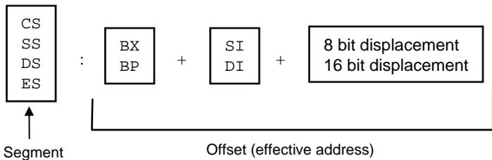
Various combinations of the elements may be used to form an effective address. Not all the elements are required.
