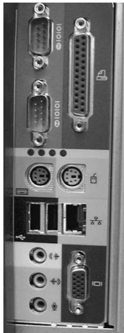
Typical I/O ports on a microcomputer
