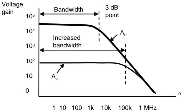
The upper frequency limit is due to the presence of internal capacitances within the IC itself which are present intentionally to enhance stability under feedback conditions.
