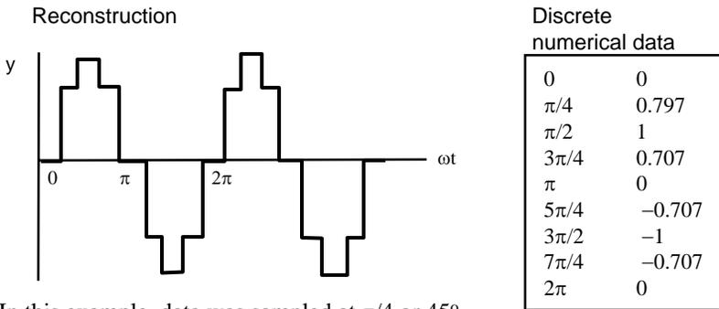
In this example, data was sampled at  $\pi/4$  or  $45^\circ$  intervals. If we decreased the sampling interval to  $\pi/8$  (i.e. an increase in the sampling rate), then we would obtain a more accurate representation of the original analog curve.
