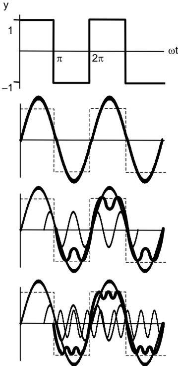
Fourier analysis, or the breaking up of a signal into its component frequencies, is important when we consider the process of filtering and the conversion of an analog signal into a digital form.
