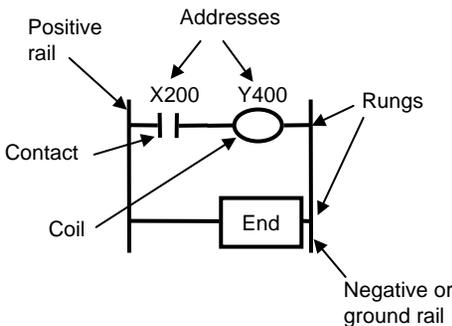
Each rung must contain one or more inputs and one or more outputs. The first object on a rung must be an input and the last object on a rung should be an output, a counter, timer or an internal relay. The last rung in a ladder diagram is an END instruction.
