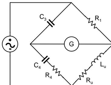
An unknown component is inserted into the bridge and the values of the others are altered to achieve balance condition.
