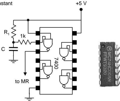
15. Connect the output of the master reset circuit to MR on the UART.
