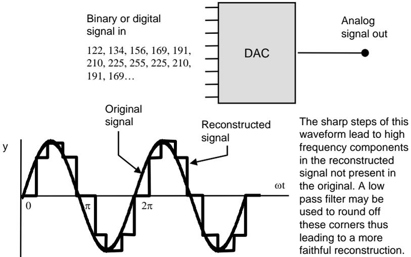
Digital to analog conversions may be made using a **ladder network** of resistors or a **weighted input** to a summing amplifier. The voltage on the output depends upon the voltages applied to the inputs. These voltages may be either 0 (for logic 0) or some supply voltage  $V_{cc}$  (for logic 1). The TTL input connected to the lowest value resistor carries more weight than the others, thus, a larger binary or digital input results in a larger analog output voltage.
