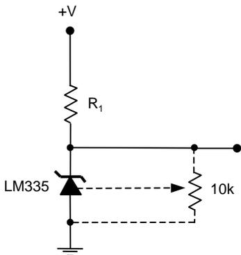
$$V_{outT} = V_{outT_o} \frac{T}{T_o}$$
