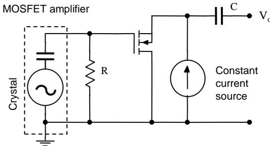
When the voltage across R varies, the bias voltage across the MOSFET changes and the signal is passed through the coupling capacitor C providing a measure of force.
