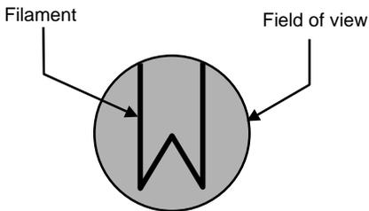
Usually, a **red filter** is used at the eyepiece so that matching is done at a particular wavelength (makes it easier to obtain a match). A correction table is used to obtain a true temperature from the indicated value which accounts for non-black body radiation when using the red filter.
