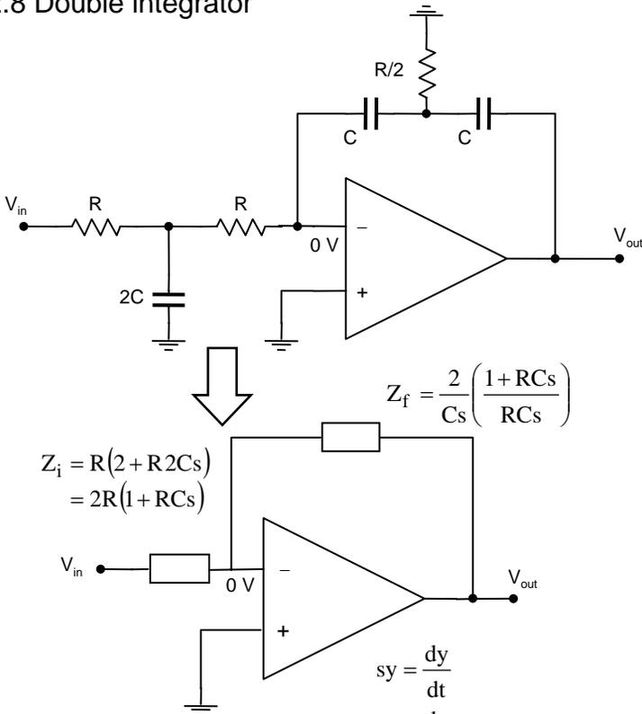
The transfer function for this circuit is easily obtained in the s-domain using transfer impedance results for the T-networks shown previously. The final transfer function involves a  $s^{-2}$  term. Now,  $s$  is a differential operator so that  $s^{-1}$  is an integral operator. Here, we have an  $s^{-2}$  which means that the circuit takes the integral twice – a **double integrator**.
