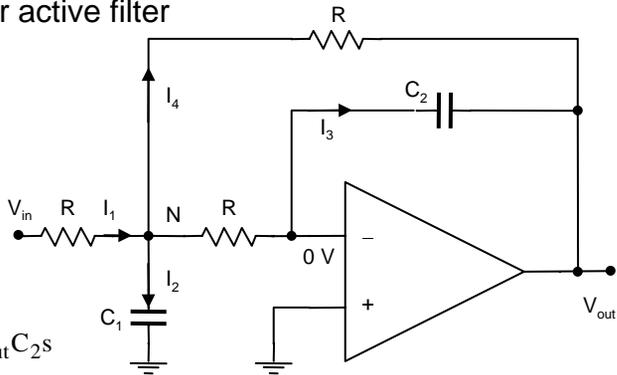
$$\frac{V_{in} - V_N}{R} = V_N C_1 s + -V_{out} C_2 s + \frac{V_N - V_{out}}{R}$$
