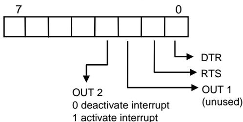
For COM2, the MCR port address is 2FC
