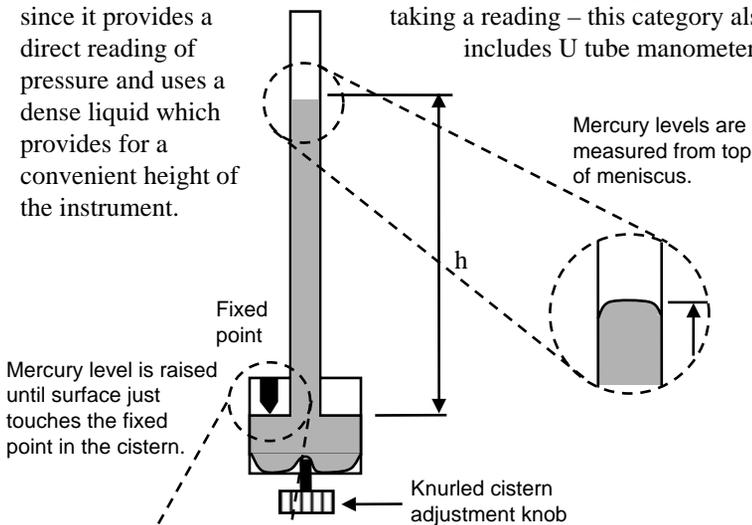
Mercury level is raised until surface just touches the fixed point in the cistern.
