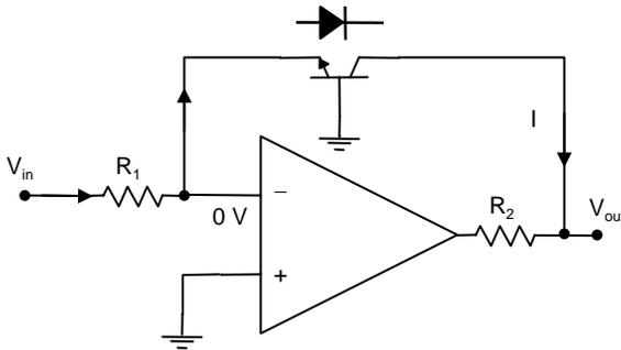
The **feedback transistor** has its collector at 0 V (virtual earth) and the base is also at ground potential (0 V). With the collector and base effectively shorted together, the device acts like a diode across the base-emitter pn junction.
