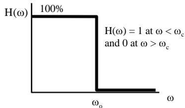
If this function  $H(\omega)$  were multiplied with the Fourier transform of  $y_{in}$ , then the amplitude of all components of the Fourier transform above  $\omega_0$  would be reduced to zero thus eliminating (or at least reducing) the high frequency noise component of the signal.
