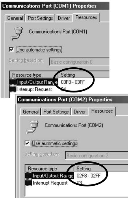
Each port address is a **register** that allows the serial port to be initialised and operated on by software commands. That is, the serial port controller chip, the 8250 UART, is **programmable** in the sense that its operation can be controlled by software rather than hard-wired circuitry.
