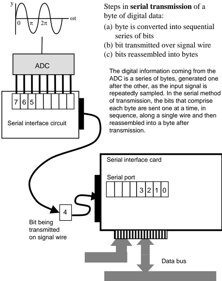
Steps in **serial transmission** of a byte of digital data:
