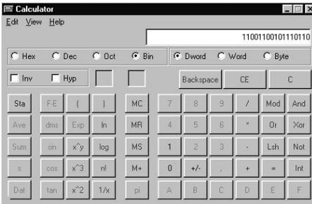
2. Set the Calculator to HEX mode and set to BYTE and then type in FFFF. Convert this number to Decimal and then Binary by selecting the appropriate buttons:
