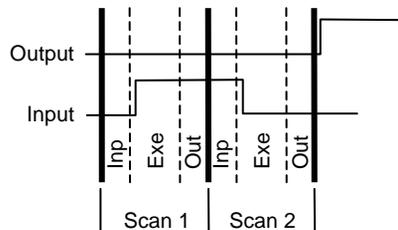
In some PLCs, the program is executed line by line. The control unit scans the inputs actually referenced by each program statement as it is executed. The output named in each program statement is then updated according to the logical operation in the program statement and then held or latched in that state.
