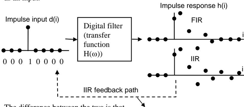
The difference between the two is that for the FIR, the output of the filter decays to zero for an impulse input. The output of an FIR filter depends on the present, and previous inputs (the filter is non-recursive). The output from an IIR filter employs a feedback mechanism so that the output depends upon past outputs as well as past and present inputs (i.e. recursive).
