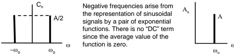
This plot is the magnitude of the *exponential* components of the signal. A frequency spectrum using trigonometric coefficients would be a single line of height  $A$  at  $\omega_o$ .
