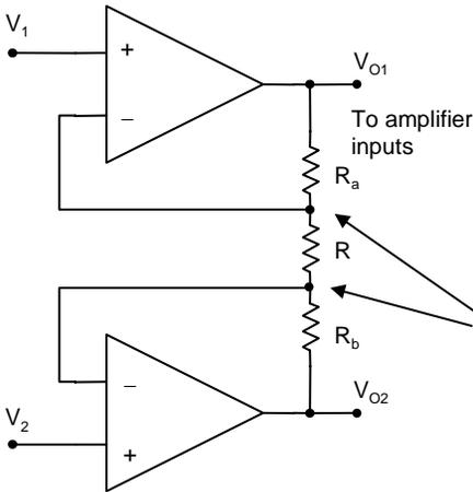
Note: This input stage is **not a difference amplifier**. The difference in the output voltages = the gain times the difference in the input voltages. Common mode signals are passed through without being amplified. A proper difference amplifier rejects the common mode signal altogether.
