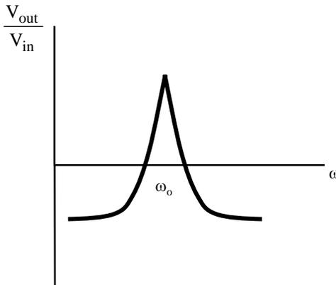
If the twin-T filter moved to the input, we would obtain a **band reject** or **notch** filter.
