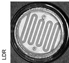
e.g. A popular material for LDRs is cadmium sulphide (CdS). CdS has a peak response at 600 nm,  $E_g = 2$  eV and matches the frequency response of the human eye quite closely. In contrast, lead sulphide (PbS) ( $E_g = 0.4$  eV) has a peak response at 300 nm.
