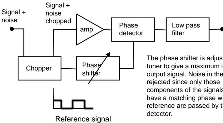
The phase shifter is adjusted like a tuner to give a maximum in the output signal. Noise in the signal is rejected since only those components of the signals which have a matching phase with the reference are passed by the phase detector.
