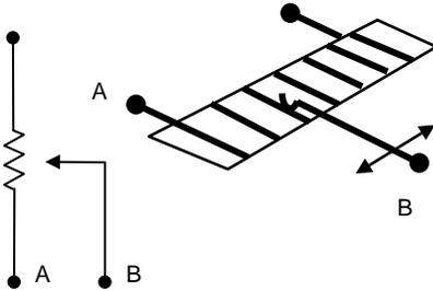
A coil of wire is wound on a mandrel. If the winding is uniform and the wire is of a constant cross-section  $A$  and resistivity  $\rho$ , then the resistance  $R$  is:
