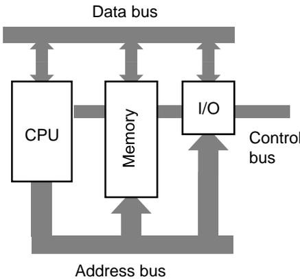
Binary information is transferred as TTL logic across wires called the **bus** – the **address bus**, the **data bus** and the **control bus**. When an address is placed on the address bus, the byte of information at or for that memory location is placed on the data bus. Signals on the control bus tell the CPU whether a read or write operation to that memory cell is required.
