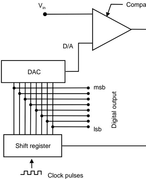
This method allows high speed data acquisition (up to 100 000 conversions/sec). However, the opportunity for errors to be introduced is greater. The fixed conversion time means that the input signal needs to be steady or at least captured during the sampling period.
