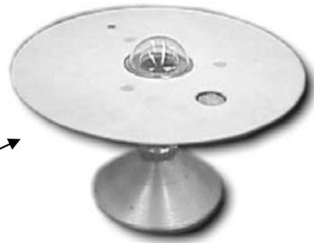
Still yet another type of thermal detector utilises the **pyroelectric** property of certain ferroelectric materials. Incident radiation causes a change in the surface charge of a residually polarised ceramic. The effect can only be measured in a pulsed mode of operation and hence an AC amplifier is used to produce a reasonable output.
