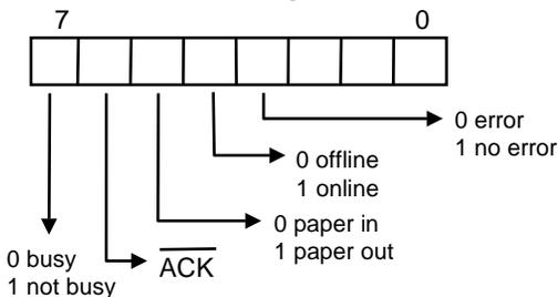
**Printer port control register (base +2) 37A**
