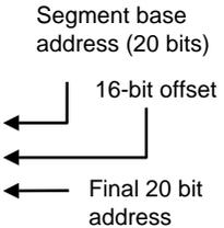
2. The 16-bit offset is added to the segment base address to obtain the 20-bit absolute address.
