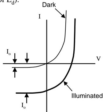
The reverse bias current is directly proportional to the luminous intensity. Sensitivity is in the order of 0.5 A/W.
