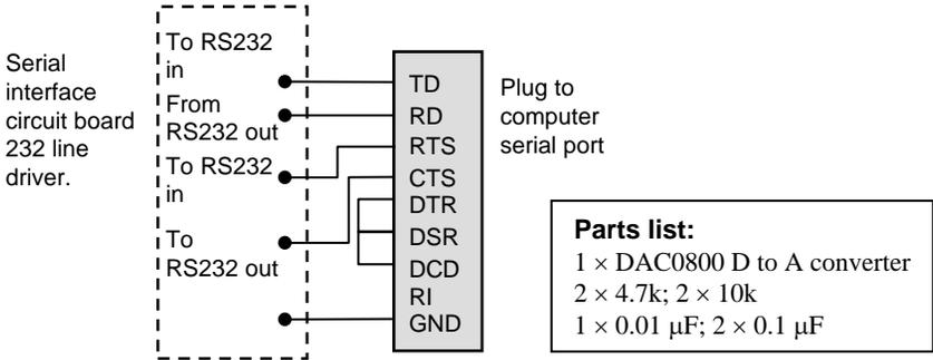
1. The first step in our DAC converter is to obtain a digital signal from the serial port of the computer. Connect the TD signal line from the computer serial port to an available RS232 IN pin on the 232 line driver. Connect the corresponding TTL out to pin RRI (receive register input) on the 6402 UART.
