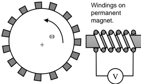
Magnetic teeth on rotor modifies the **magnetic circuit** when the rotor is rotating. This induces a voltage in the windings which surround the magnet.
