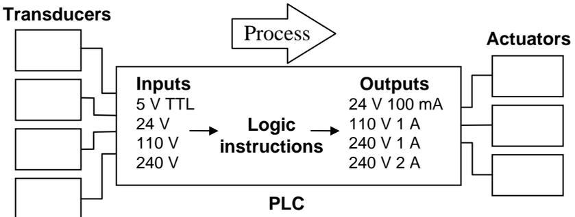
A PLC itself consists of the control unit (or CPU) as well as connections for input and outputs, RAM memory ( $\approx 10$  Kb) and a power supply. Inputs are opto-coupled to the input circuits in the PLC to protect the PLC from noise.
