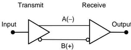
In tri-state logic, pins can be at logic 0, logic 1 or high impedance. The last state effectively disconnects the driver from the line. The high impedance state is set by an "enable" signal on the driver chip.
