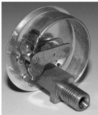
The tube itself is made from brass and has a flattened elliptical or rectangular cross-section.
