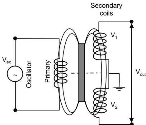
Note: Arrangement of secondary coils means that the voltage induced in each of them is opposite in polarity:
