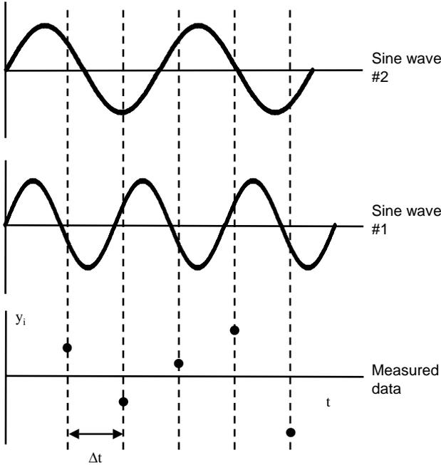
Consider a set of measurements of a quantity  $y$  taken at equal time intervals  $\Delta t$  (a sampling frequency of  $1/f$ ).
