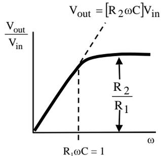
$$\left| \frac{V_{out}}{V_{in}} \right| = \frac{R_2}{R_1} \frac{R_1 C \omega}{\sqrt{1 + (R_1 \omega C)^2}}$$
