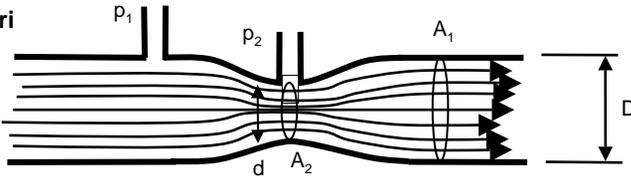
For an incompressible fluid, and frictionless flow, the theoretical volume flow rate  $Q_{th}$  is:
