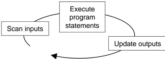
The states of all the inputs are copied into RAM before the program instructions are executed. Instructions are then processed in sequence. The resulting output states are stored in RAM. When the program execution is completed, the stored output states are transferred to the output terminals of the PLC.
