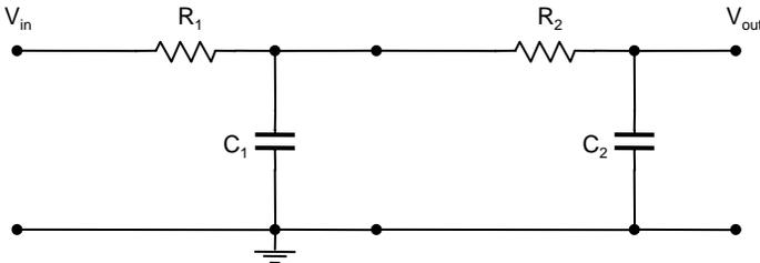
Input Z of 2nd stage = output Z of 1st stage. To minimise loading,  $R_2 \gg R_1$  and  $C_2 \ll C_1$ .
