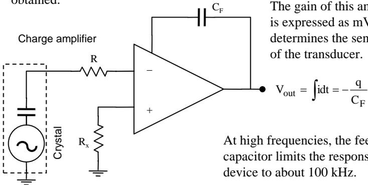
The gain of this amplifier is expressed as mV/pC and determines the sensitivity of the transducer.
