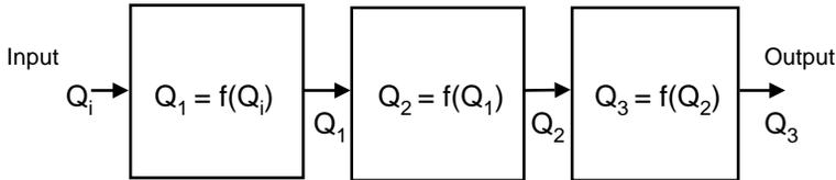
It is desirable to have linear relationships between the inputs and outputs of the various processes so that  $Q_3 = K_1 K_2 K_3 Q_i$ .
