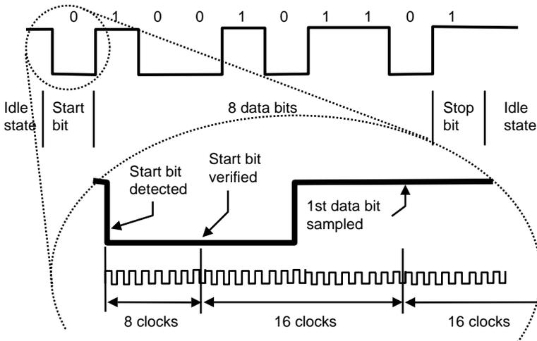
The receiver clock is usually made 16 times the bit rate. When a mark to space transition is detected, the receiver counts 8 clocks. If the signal is still at space, then it is assumed that the signal is a valid start bit. The receiver counts off another 16 clocks and then samples the data until all the data bits and stop bit(s) have been received. The bit sampling thus takes place in the centre of the signal levels.
