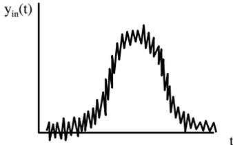
The high frequency noise would lead to an increase in  $F[y_{in}(t)]$  at high frequencies. If it were possible to separate out the signal of interest  $y_s$  from the noise  $y_n$ ,  $F[y(t)]$  for each would be something like:
