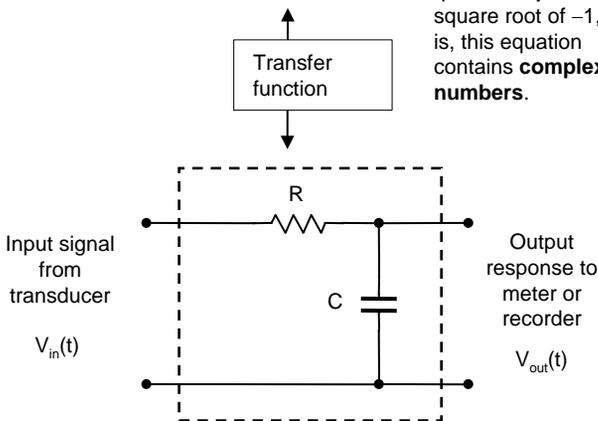
Later, we shall see how the transfer function for a wide variety of circuits (mainly filter circuits) can be obtained easily using **operator** notation. The transfer function for a particular filter circuit can be used to modify the signal being measured so as to eliminate **noise** (i.e. unwanted information). The mathematical representation of the transfer function allows the effect of various filter and amplifier circuits to be analysed and designed before any actual circuit is constructed.
