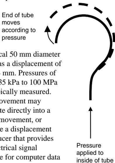
A typical 50 mm diameter tube has a displacement of up to 4 mm. Pressures of about 35 kPa to 100 MPa are typically measured. The movement may translate directly into a meter movement, or activate a displacement transducer that provides an electrical signal suitable for computer data acquisition.
