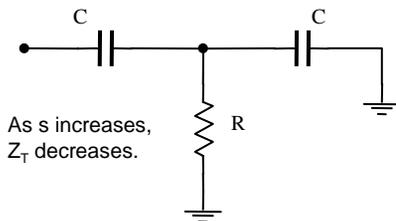
$$Z_T = \frac{V_{in}}{I_2} = \frac{1}{Cs} \left( \frac{1 + 2RCs}{RCs} \right)$$
