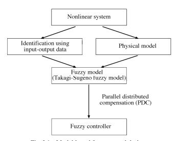
Fig. 2.1 Model-based fuzzy control design.
