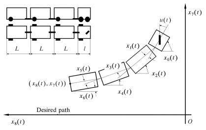
**Fig. 8.1** Vehicle model with triple trailers.
