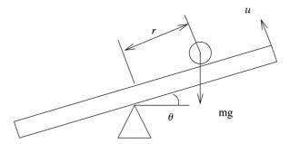
Fig. 12.1 The ball and beam system.
