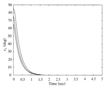
**Fig. 2.18** Angle response using two-rule fuzzy control.
