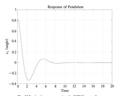
Fig. 13.2 Angle response using the DPDC controller.
