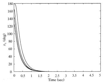
Fig. 2.20 Angle response using four-rule fuzzy control.
