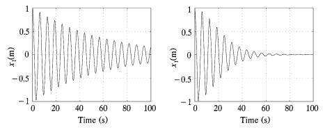
**Fig. 7.3** Control results for TORA with parameter change ( $\varepsilon = 0.05$ ).
