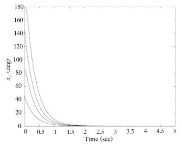
**Fig. 2.23** Closed-loop angle response with *l* changed.
