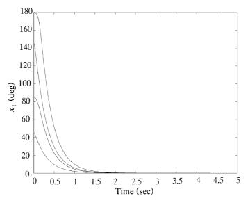
Fig. 2.21 Closed-loop angle response with m changed.
