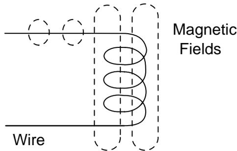
**Fig. 10.1** Magnetic fields (dashed lines) around current-carrying wire.
