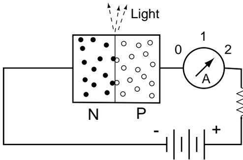
**Fig. 14.1** A PN diode, "forward biased," with current flowing. Black dots are electrons, and circles are holes. (A "bias" is a small voltage applied to a device, tending to make a current flow in a certain direction.)
