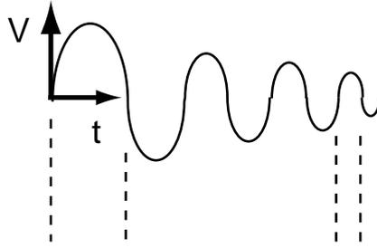
**Fig. 19.3** Voltage versus time for a damped wave.
