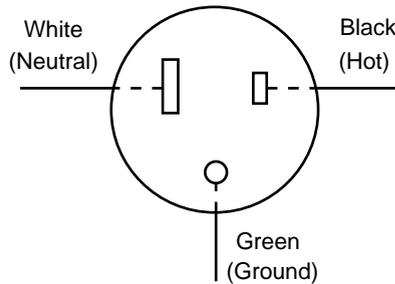
**Fig. 6.2** Standard wall socket ("power outlet" or "mains") for 120 volt ac.
