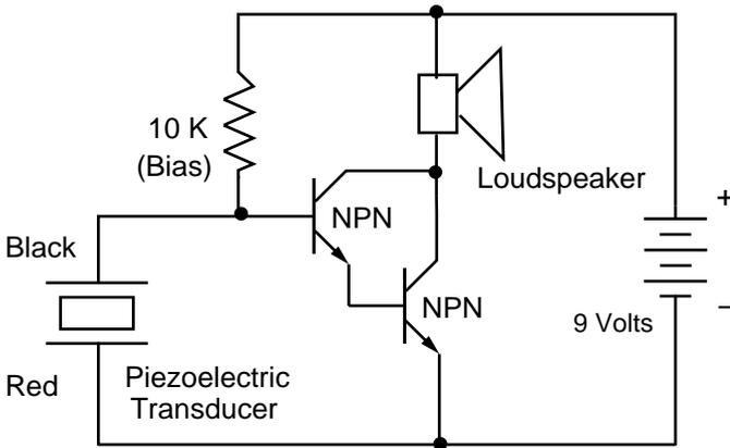
**Fig. 15.8** A Darlington circuit, driving a loudspeaker.
