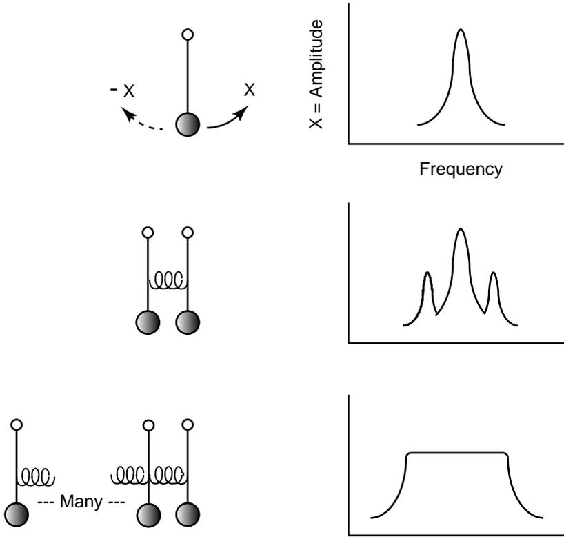
**Fig. 13.1** Coupled pendula, vibrating at their natural frequencies.
