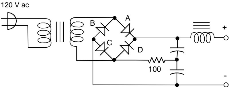
**Fig. 14.8** A full wave rectifying voltage doubler.
