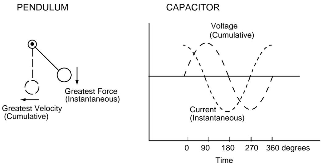
**Fig. 9.7** "Out of phase" situations in a pendulum and a capacitor.
