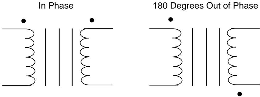
**Fig. 10.6** Coils drawn a different way. (Also, the dots show phases.)
