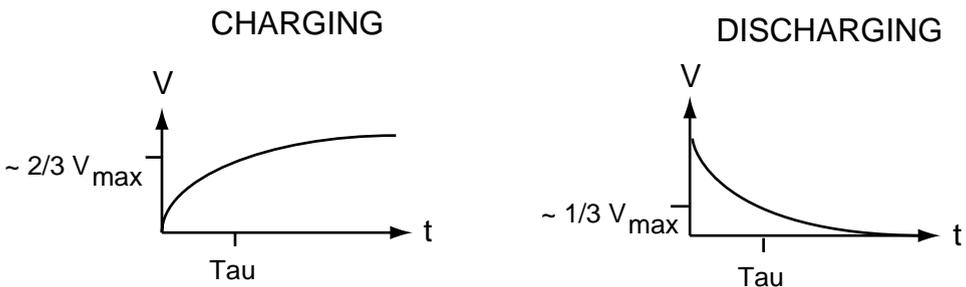
**Fig. 9.4** The voltage across a capacitor, versus time.
