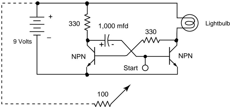
**Fig. 17.2** A monostable multivibrator that generates a pulse.
