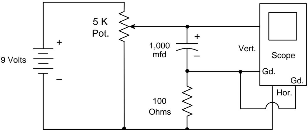
**Fig. 9.6** Voltage versus current in a capacitor.
