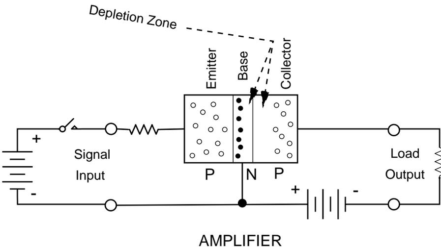
**Fig. 15.1** A PNP transistor in a "common base" arrangement. (All the currents go through the same base wire.)
