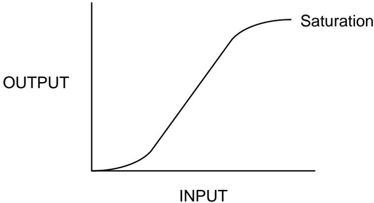
**Fig. 15.7** The characteristic curve of a transistor.
