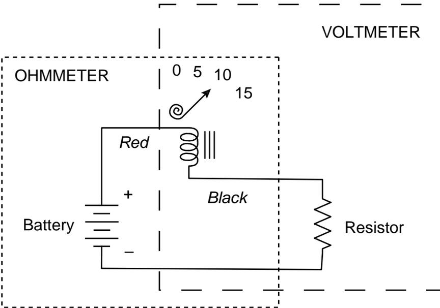
Fig. 2.4 A "multimeter."
