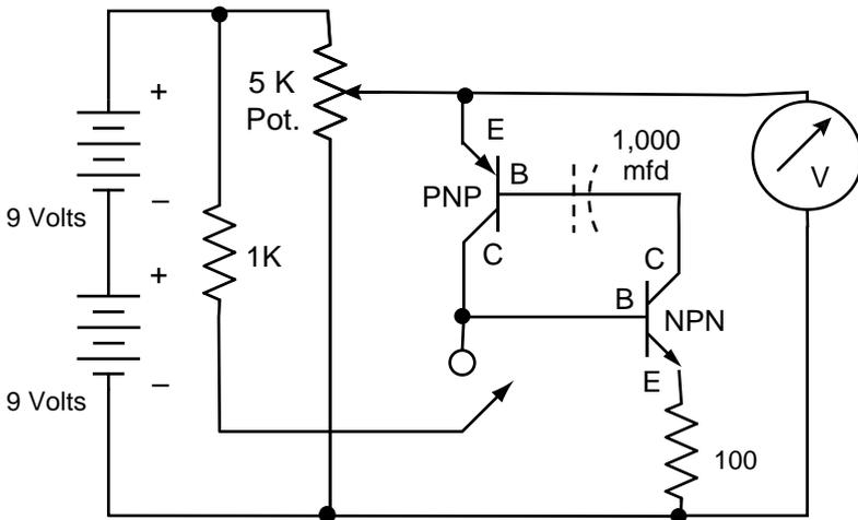
**Fig. 21.2** Complementary monostable multivibrator ("trigger").
