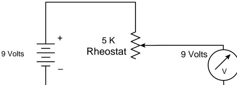
**Fig. 4.4** A rheostat, which does not control voltage.
