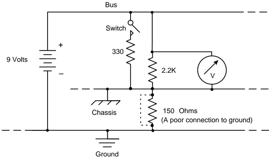
Fig. 6.3 One component interfering with another's operation ("SSN").
