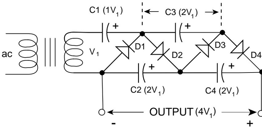
**Fig. 14.9** A half wave rectifying voltage quadrupler.
