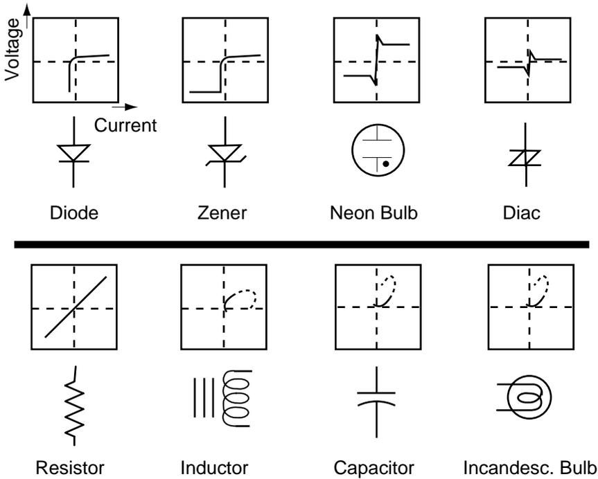
Fig. 14.4 Curve traces for various kinds of diodes.
