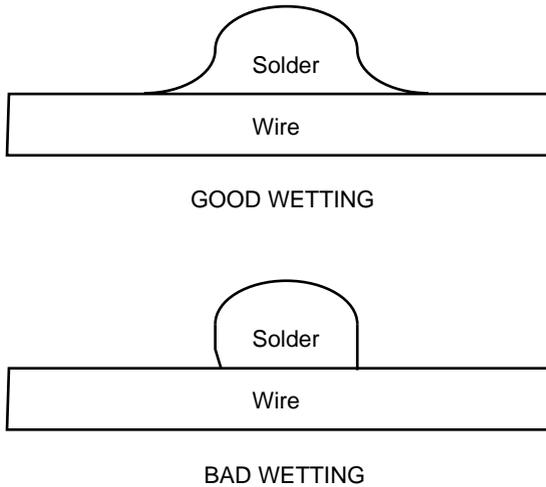
**Fig. 7.2** Good and bad solder "contact angles."
