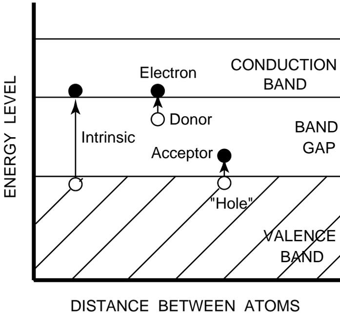
**Fig. 13.2** Energy bands (vertical), extending across a crystal (horizontal).
