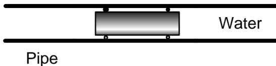
**Fig. 10.4** A piston analog of an inductor, with an O-ring seal at each end.
