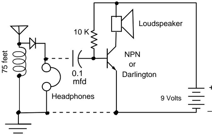
**Fig. 19.1** Ultra-simple "crystal radio," with optional amplifier.
