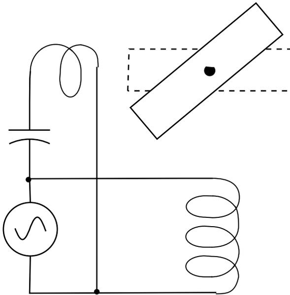
**Fig. 20.6** An ac motor with a capacitor starter.
