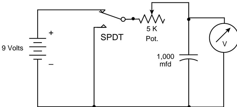
**Fig. 9.5** Circuit for charging and discharging a capacitor.
