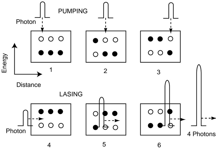
**Fig. 22.2** Light amplification by stimulated emission (a laser).
