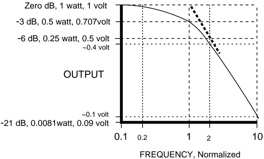
**Fig. 11.2** Output of the filter in Fig. 11.1, when  $R = X_C$ . Both the transfer function and the frequency are normalized in this diagram. The frequency labeled "1" is really  $1/2\pi RC$ . (Log  $V$  versus log  $f$  is called a "Bode plot.")
