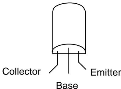
**Fig. 15.2** The TO-92 plastic package for a transistor.
