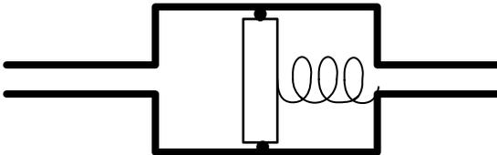
**Fig. 9.1** A water analog of a capacitor.
