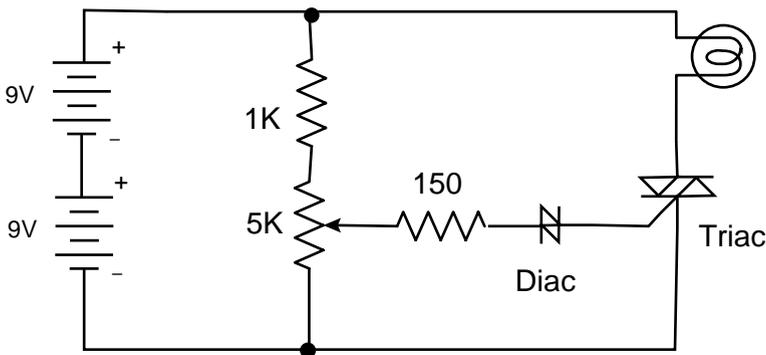
**Fig. 21.5** Triggering and gating circuit (optional experiment).
