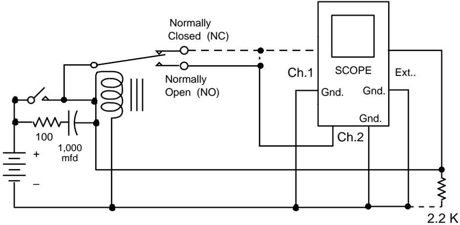
**Fig. 12.4** Measuring the speed of relay operation. (In some cases the 2.2K might be needed, in order to discharge a capacitor that is in the scope's "external trigger" circuit, before each new timing operation.)
