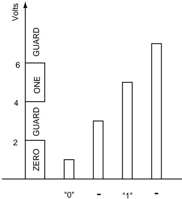
**Fig. 19.5** Digital signal pulse heights and gate ranges.
