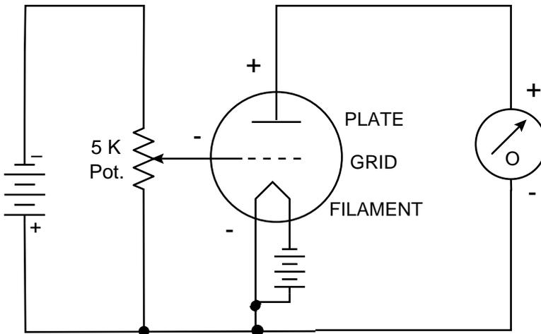
**Fig. 18.1** Triode vacuum tube amplifier. (Compare to page 168.)
