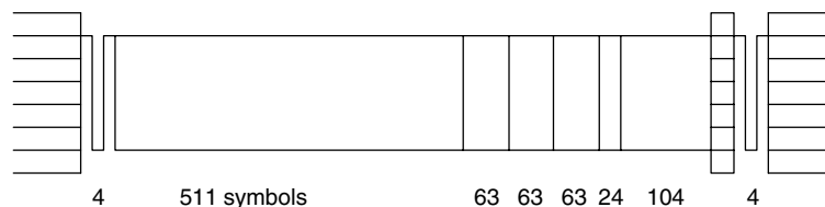
Figure 1-7. Field sync for the ATSC system. (From ATSC DTV Standard A/53, Annex D; used with permission.)
